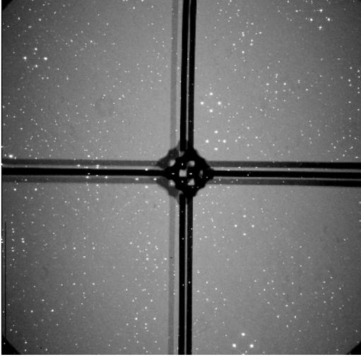
**Figure 1.** An example of a RoboPol image. Each point in the sky is mapped to four spots on the CCD. A focal plane mask, held in place by four support legs, reduces the sky background level for the central target.
