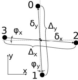
**Figure 3.** The pattern of 4 spots at each position  $(x, y)$  on the CCD and 6 parameters describing it.  $\Delta_x(x, y)$  is the distance between the horizontal spots,  $\delta_x(x, y)$  is the distance from the right-spot to the central point, and  $\phi_x(x, y)$  is the angle between the CCD x-axis and the line connecting horizontal points.  $\Delta_y(x, y)$ ,  $\delta_y(x, y)$  and  $\phi_y(x, y)$  denote similar quantities for the vertical pair of spots.
