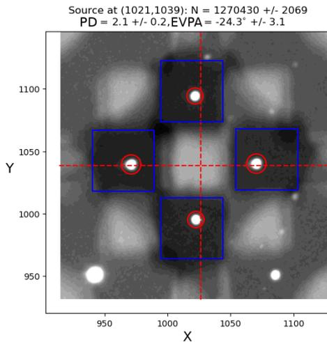
**Figure 2.** Masked central area of the RoboPol image with the central science target. The red circles are the photometry apertures. The blue squares are the automatically identified background estimation areas for the central science target.
