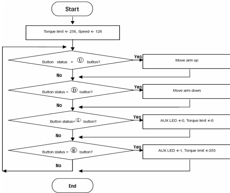
Figure 2.11: Typical Flow Chart Structure
