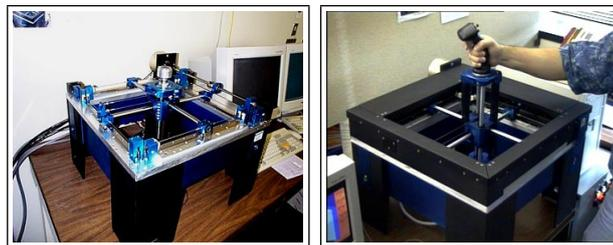
Figure 1.4: The Linear Haptic Display
