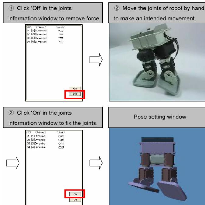
Figure 2.9: The Procedure for Manually Making Poses
