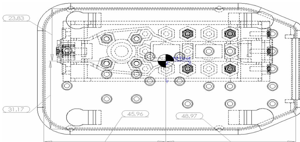
Figure 6.1: The Support Polygon's Dimensions
