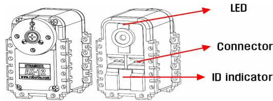
Figure 2.6: The Main Parts of the AX-12
