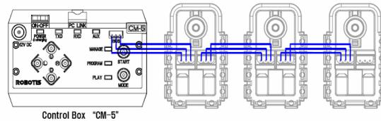
Figure 2.16: Serial Chain Connection of Cm-5 and AXs
