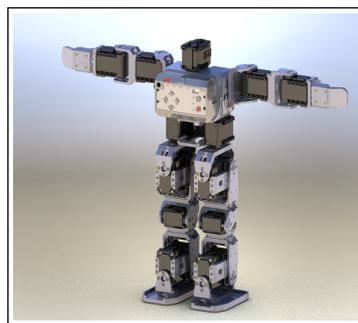
Figure 3.5: The Total Assembly Rendered in Solidworks
