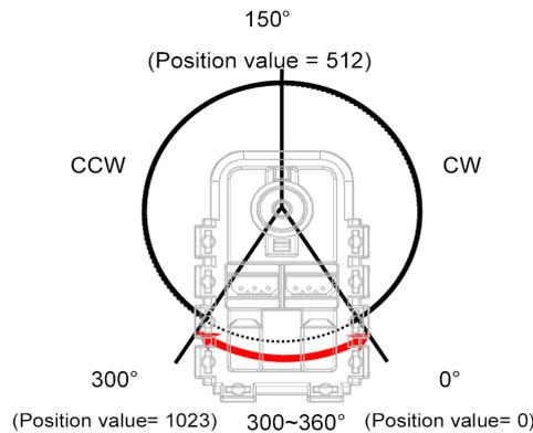
Figure 2.5: The Acceptable Actuator Values
