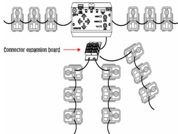
Figure 2.8: The Communication Chain between CM-5 and AXs
