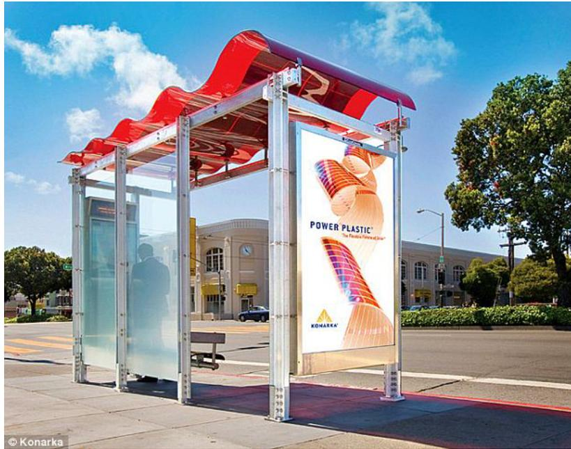
Figure 1.12: Wi-Fi enabled transit shelter in San Francisco based on Power Plastic PV module
