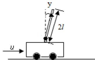
**Figure 4.2 Inverted pendulum on a cart**
