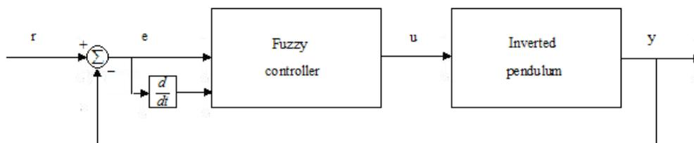
**Figure 4.3 Fuzzy controller for an inverted pendulum on a cart**
