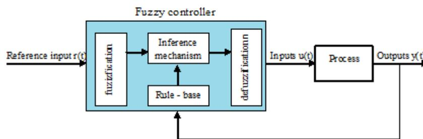
**Figure 4.1 Block diagram of a fuzzy controller**
