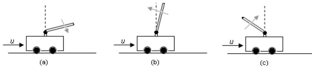
**Figure 4.4 Inverted pendulum on a cart in various positions**
