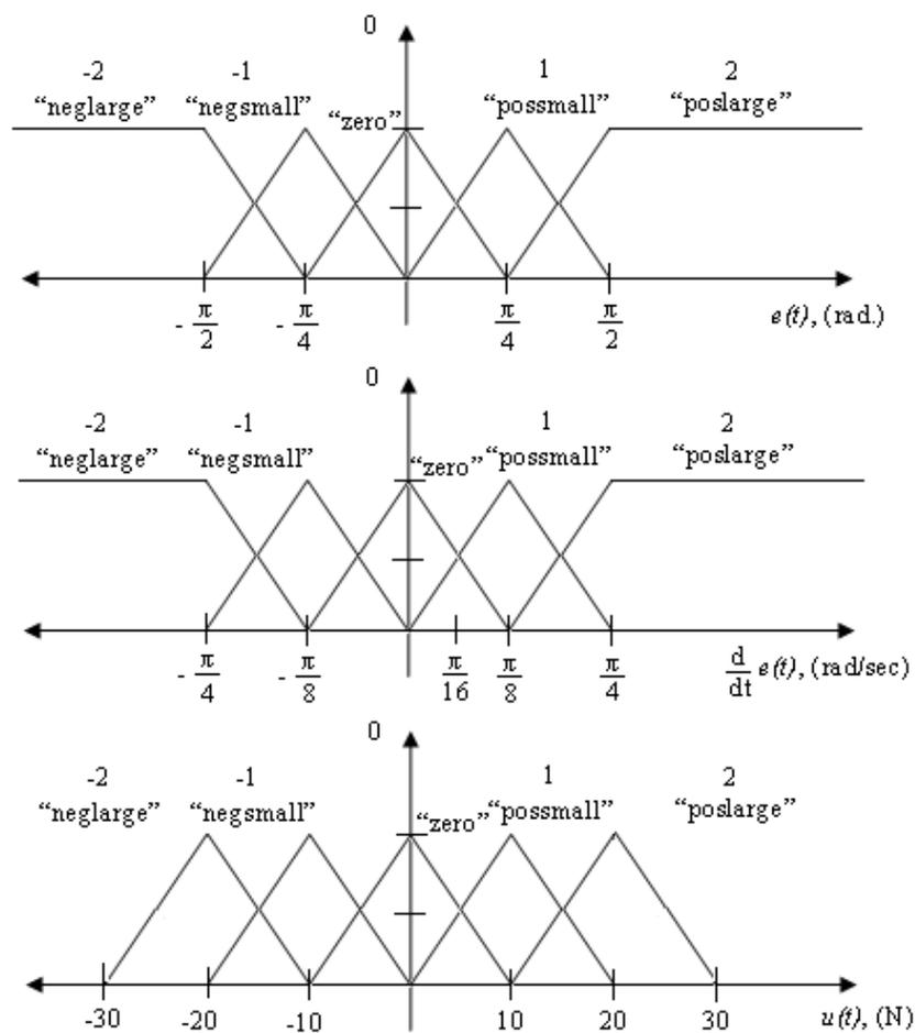
**Figure 4.8 Membership functions for an inverted pendulum on a cart**
