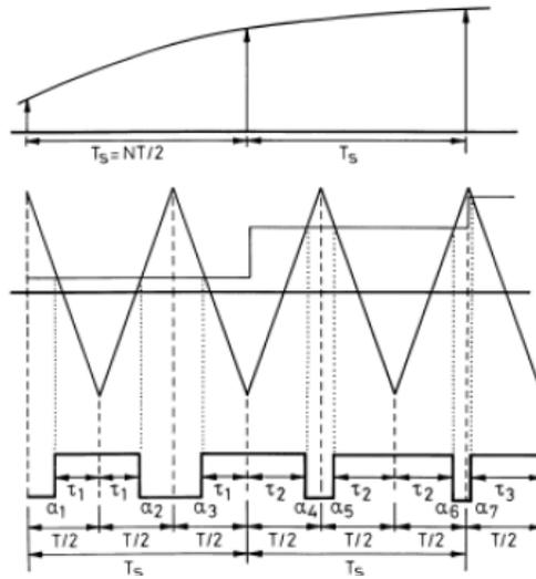
**Fig. 23.** High switching frequency, low sampling frequency SPWM generation method. Sampling frequency =  $f_s$ , sampling period =  $T_s$ , carrier frequency =  $f_c$ , carrier period =  $T$ ,  $f_s = 2f_c/N$ ,  $T_s = NT/2$ .
