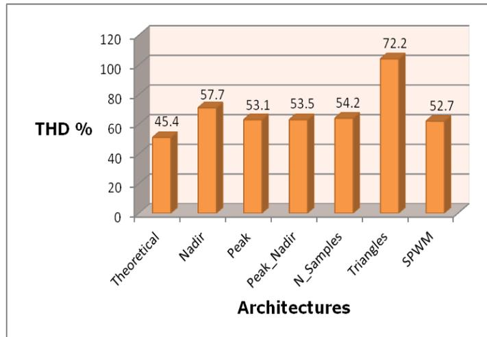
**Fig. 87.** THD for all SPWM generation architectures for  $f_c = 1$  kHz and  $M = 0.9$ .
