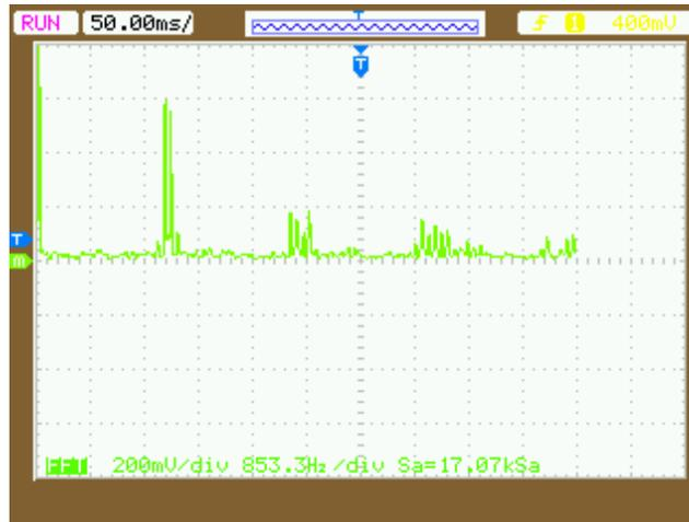
Fig. 54. The FFT of the SPWM signal in case that  $M = 0.5$  and  $f_c = 1$  kHz.
