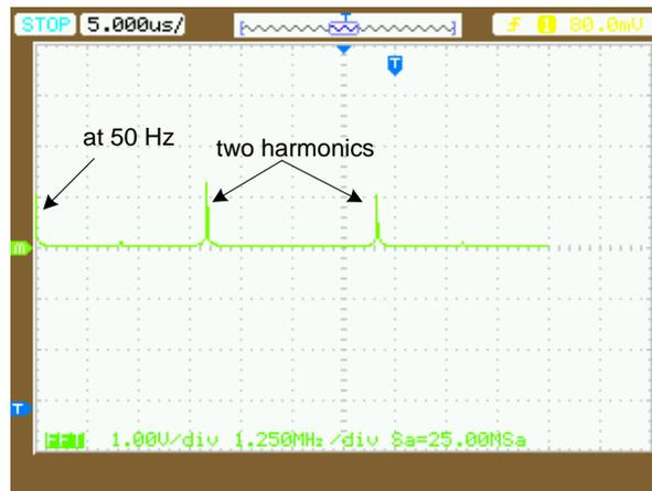
Fig. 64. FFT pattern in case that  $M = 0.5$  and  $f_c = 2 \text{ MHz}$ .
