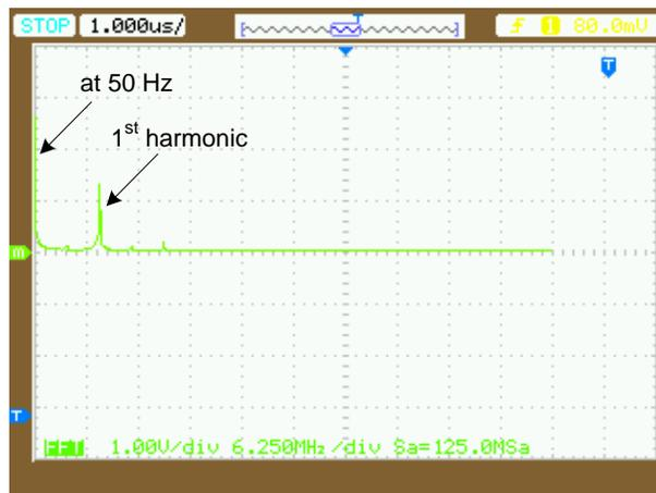
Fig. 65. FFT pattern in case that  $M = 0.5$  and  $f_c = 4 \text{ MHz}$ .
