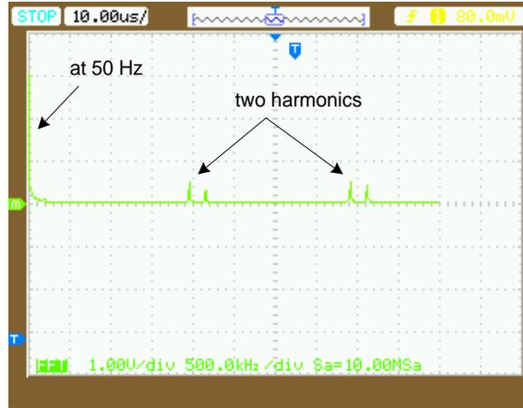
**Fig. 70.** FFT pattern for the triangles architecture ( $f_c$  max = 1 MHz,  $M = 0.5$ ).
