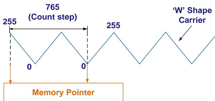
Fig. 40. Sampling at  $NxT/2$  time instants.
