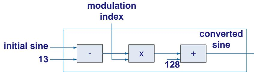
Fig. 33. Sine conversion subsystem.
