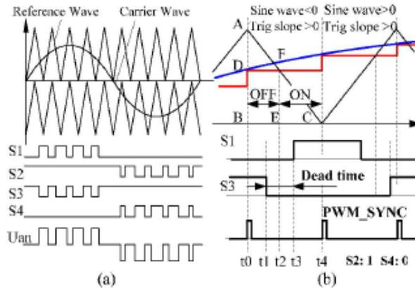
Fig. 24. SPWM generator implemented for a three-level NPC inverter.
