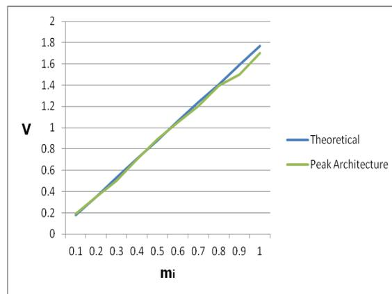
**Fig.72.** Experimental and theoretical output voltage at 50 Hz for the peak architecture in case that  $M = 0.1-1$  and  $f_c = 10$  kHz ( $d$  ranges from 0-5.7%).
