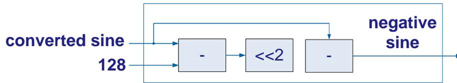
**Fig. 34.** Negative sine subsystem.
