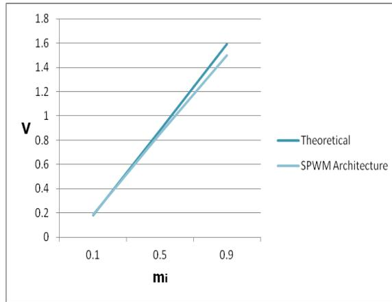
**Fig.82.** Experimental and theoretical output voltage at 50 Hz for the newly proposed architecture in case that  $M = 0.1$ , 0.5 and 0.9, respectively and  $f_c = 100$  kHz ( $d = 5.6\%$ , 3.4% and 5.7%, respectively).
