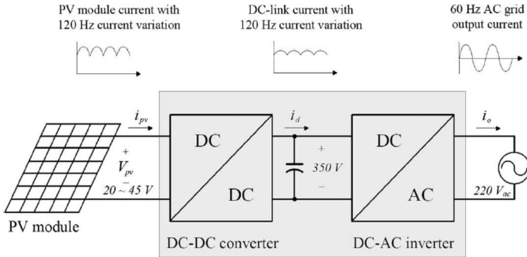
Fig. 3. Block diagram of a single-phase grid-connected PV MIC system.
