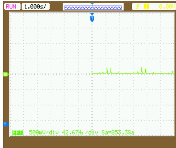
**Fig. 51.** FFT of the SPWM signal in case that  $M = 0.1$  and  $f_c = 500$  Hz.
