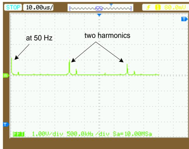
Fig. 57. FFT pattern in case that  $M = 0.5$  and  $f_c = 1$  MHz.
