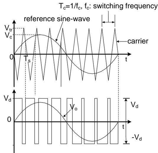
Fig. 12. Bipolar sinusoidal pulse width modulation.
