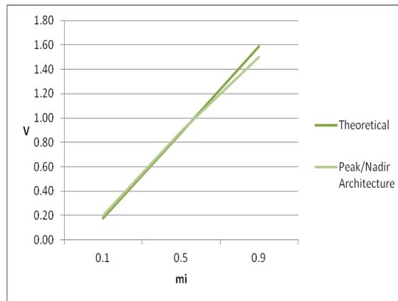
**Fig.84.** Experimental and theoretical output voltage at 50 Hz for the peak/nadir architecture in case that  $M = 0.1$ , 0.5 and 0.9, respectively and  $f_c = 250$  kHz. ( $d = 11.1\%$ , 1.1% and 5.7%, respectively).
