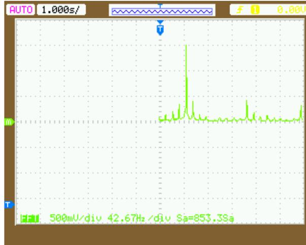
**Fig. 50.** FFT of the SPWM signal in case that  $M = 0.9$  and  $f_c = 500$  Hz.
