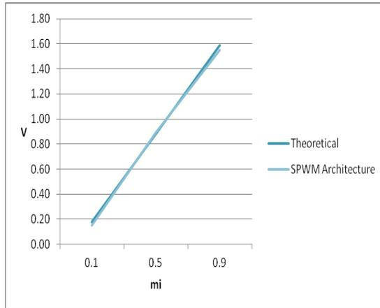
**Fig.86.** Experimental and theoretical output voltage at 50 Hz for the newly proposed architecture in case that  $M = 0.1, 0.5$  and  $0.9$ , respectively and  $f_c = 250$  kHz ( $d = 11.1\%, 1.1\%$  and  $2.5\%$ , respectively).
