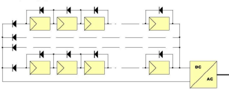
**Fig. 6.** The PV array configuration in the centralized inverter topology.
