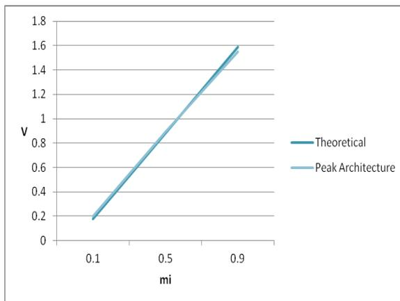
**Fig.78.** Experimental and theoretical output voltage at 50 Hz for the peak architecture in case that  $M = 0.1, 0.5$  and  $0.9$ , respectively and  $f_c = 100$  kHz ( $d = 11.1\%, 1.1\%$  and  $2.5\%$ , respectively).
