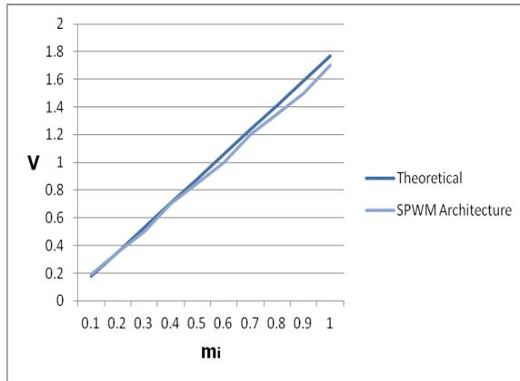
**Fig.76.** Experimental and theoretical output voltage at 50 Hz for the newly proposed architecture in case that  $M = 0.1-1$  and  $f_c = 10$  kHz ( $d$  ranges from 0-5.6%).
