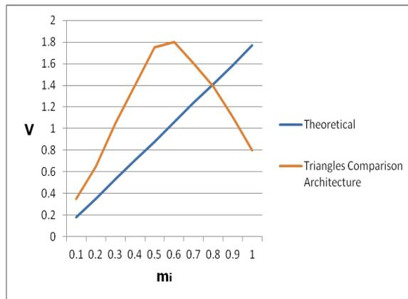
**Fig.75.** Experimental and theoretical output voltage at 50 Hz for the triangles architecture in case that  $M = 0.1-1$  and  $f_c = 10$  kHz ( $d$  ranges from 1.4-98.9%).
