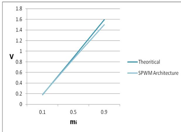
**Fig.62.** Experimental and theoretical output voltage at 50 Hz for  $M = 0.1, 0.5, 0.9$  and  $f_c = 100$  kHz ( $d = 5.6\%, 1.1\%$  and  $5.6\%$ , respectively).
