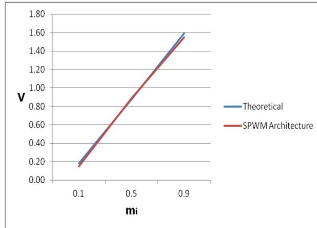
**Fig. 63.** Experimental and theoretical output voltage at 50 Hz for  $M = 0.1, 0.5, 0.9$  and  $f_c = 1$  MHz ( $d = 16.7\%, 13.13\%$  and  $2.5\%$ , respectively).
