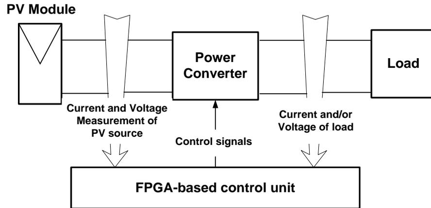
**Fig. 10.** Block diagram of a PV power production system with an FPGA-based control unit.
