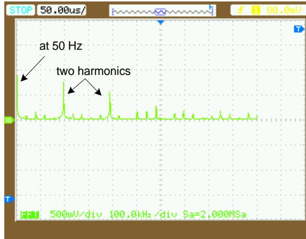
Fig. 56. FFT pattern in case that  $M = 0.5$  and  $f_c = 100$  kHz.
