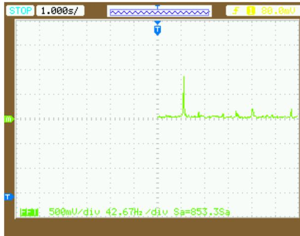
**Fig. 59.** FFT of the SPWM signal in case that  $M = 0.5$  and  $f_c = 100$  kHz.
