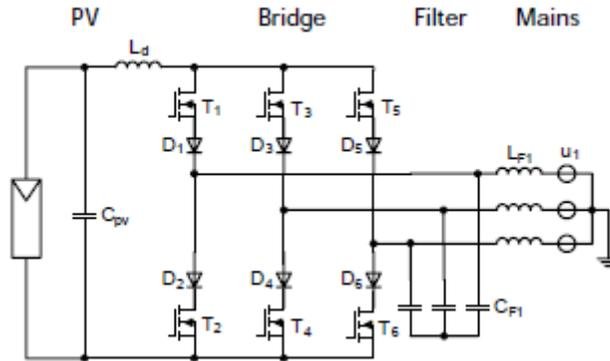
**Fig. 2.** Topology of Module Integrated Converter (MIC) based on a Current Source Inverter with a choke in the DC-link and the required series-diodes in each leg.
