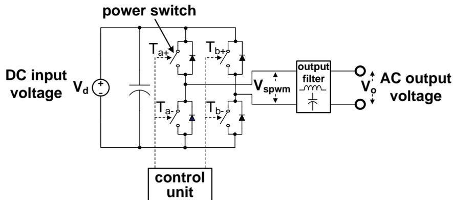
Fig. 9. DC/AC power converter (inverter) block diagram.
