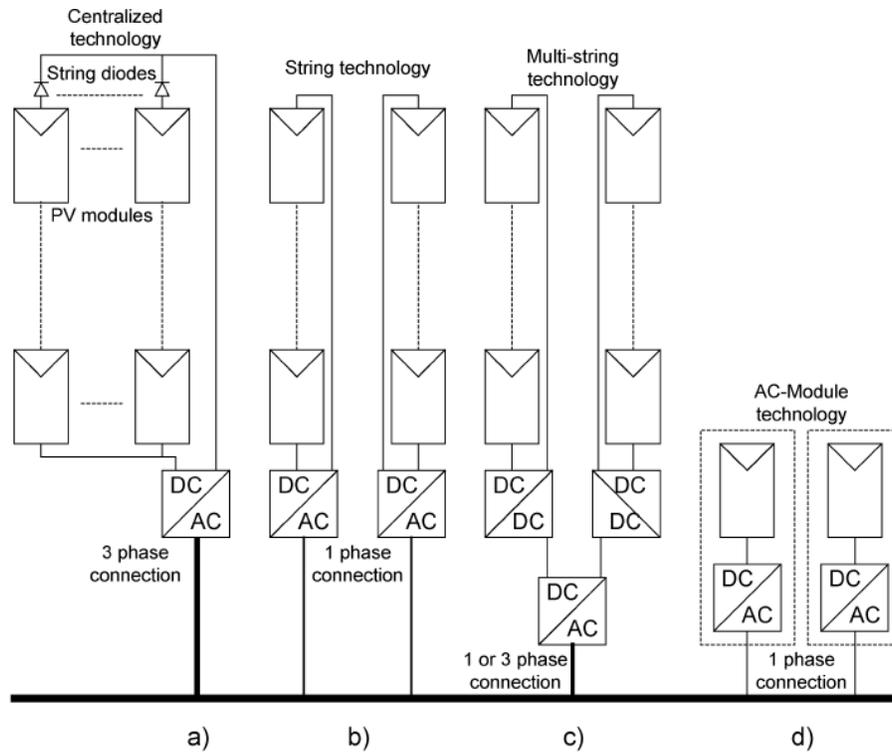
**Fig. 5.** Historical overview of PV inverters. (a) Centralized technology. (b) String technology. (c) Multi-string topology. (d) Future AC-module topology.
