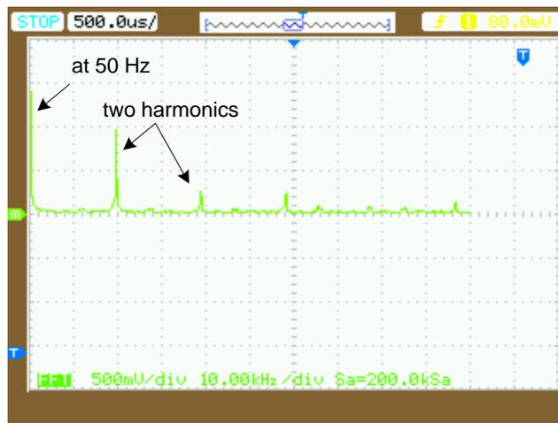
Fig. 55. FFT pattern in case that  $M = 0.5$  and  $f_c = 10$  kHz.
