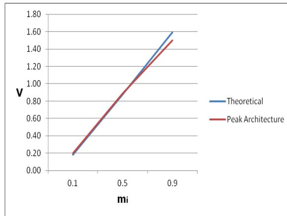
**Fig.83.** Experimental and theoretical output voltage at 50 Hz for the peak architecture in case that  $M = 0.1$ , 0.5 and 0.9, respectively and  $f_c = 250$  kHz ( $d = 11.1\%$ , 1.1% and 5.7%, respectively).
