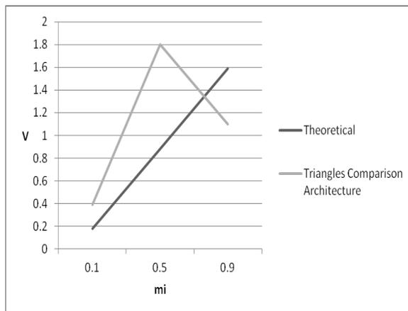
**Fig.81.** Experimental and theoretical output voltage at 50 Hz for the triangles architecture in case that  $M = 0.1$ , 0.5 and 0.9, respectively and  $f_c = 100$  kHz ( $d = 116.7\%$ , 104.8% and 30.8%, respectively).
