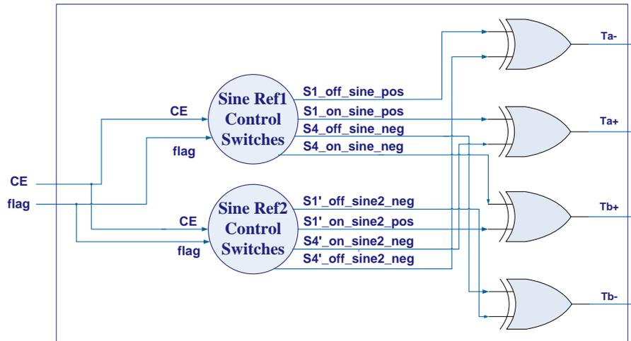
**Fig. 45.** Control units for the unipolar SPWM generator.
