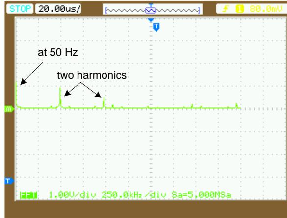
**Fig. 67.** FFT pattern for the peak architecture ( $f_c$  max = 250 kHz,  $M = 0.5$ ).
