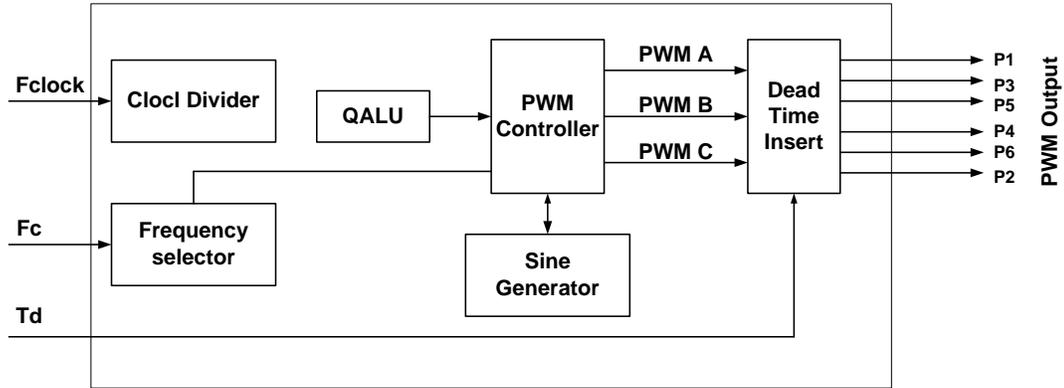
Fig. 22. Block diagram of the SPWM generator proposed in [32].
