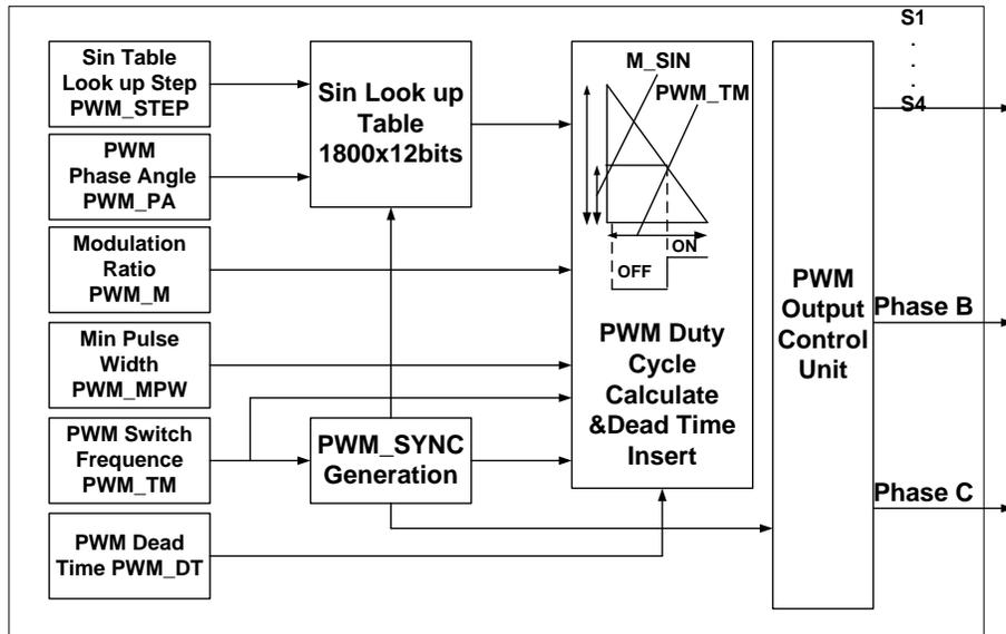
Fig. 26. Block diagram of digital SPWM generation unit.
