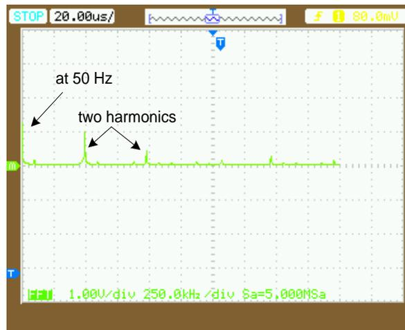
**Fig. 68.** FFT pattern for the peak/nadir architecture, ( $f_c$  max = 250 kHz,  $M = 0.5$ ).
