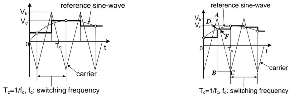
**Fig. 14.** The reference sine-wave digital representation in past-proposed SPWM generator design methods.
