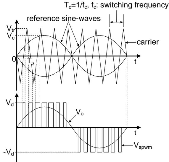
**Fig. 13.** Unipolar sinusoidal pulse width modulation.
