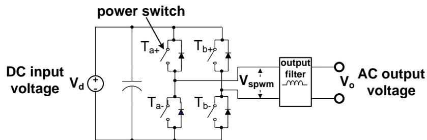
Fig. 11. Single-phase full-bridge inverter.
