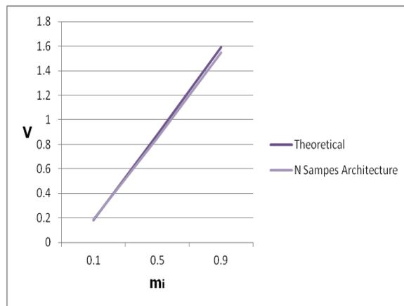
**Fig.80.** Experimental and theoretical output voltage at 50 Hz for the n samples architecture in case that  $M = 0.1$ , 0.5 and 0.9, respectively and  $f_c = 100$  kHz ( $d = 5.6\%$ , 3.4% and 2.5%, respectively).
