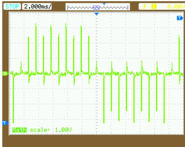
**Fig. 52.** SPWM for  $M = 0.1$  and  $f_c = 500$  Hz.
