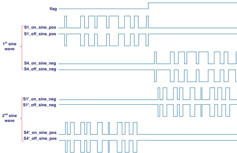
**Fig. 44.** Switch operation for a sinusoidal period.
