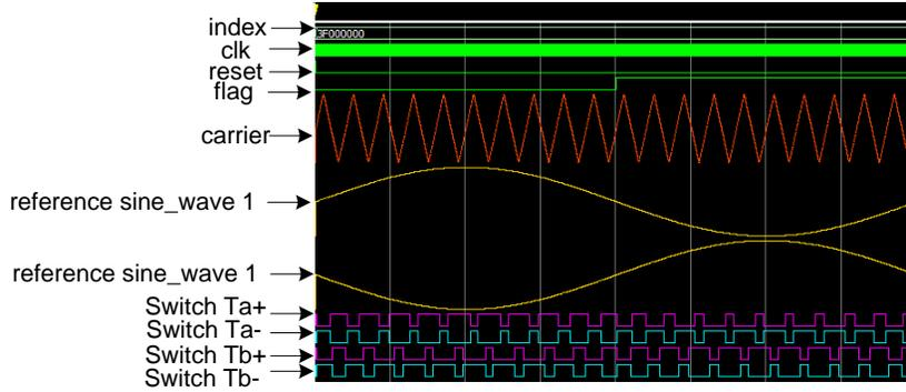
**Fig. 46.** The major internal signals of the proposed system and the SPWM outputs in case that  $f_c = 1$  kHz,  $f_s = 4$  MHz and  $M = 0.5$ .
