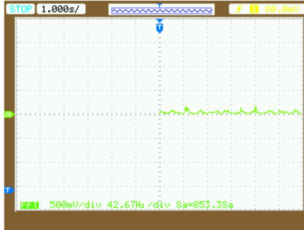
**Fig. 58.** FFT of the SPWM signal in case that  $M = 0.1$  and  $f_c = 100$  kHz.
