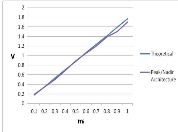
**Fig. 73.** Experimental and theoretical output voltage at 50 Hz for the peak/nadir architecture in case that  $M = 0.1-1$  and  $f_c = 10$  kHz ( $d$  ranges from 0-5.7%).
