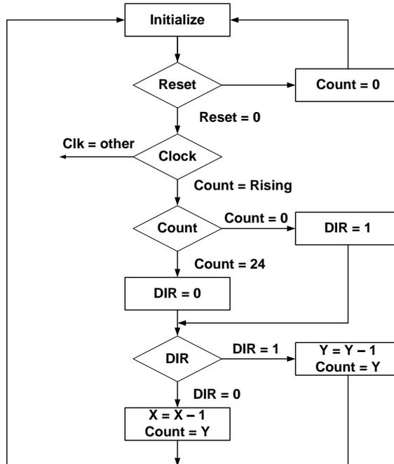
Fig. 18. The flowchart of the algorithm which produces sine-wave by a quarter of a cycle .
