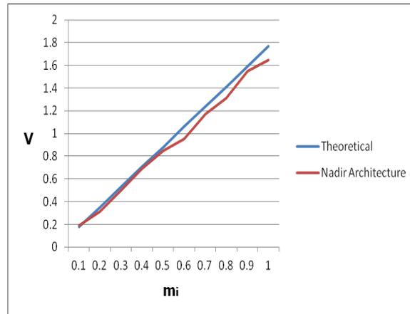
**Fig.71.** Experimental and theoretical output voltage at 50 Hz for the nadir architecture in case that  $M = 0.1-1$  and  $f_c = 10$  kHz ( $d$  ranges from 2.5-11.4%).
