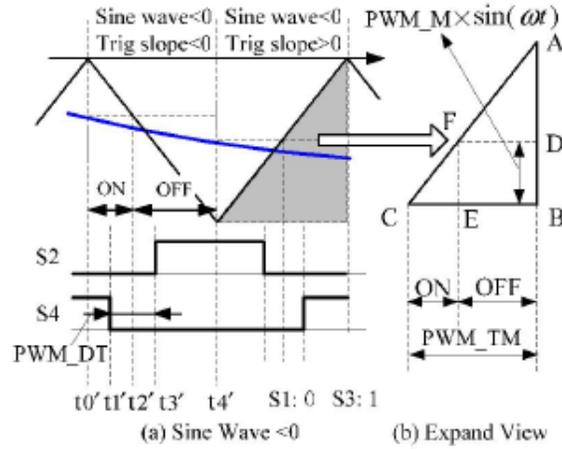
Fig. 25. Calculation of PWM duty cycle.
