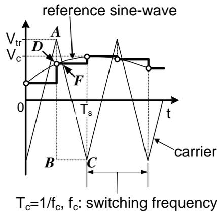
Fig. 15. The triangles ABC and ADF formed between the carrier and sinusoidal waveforms.
