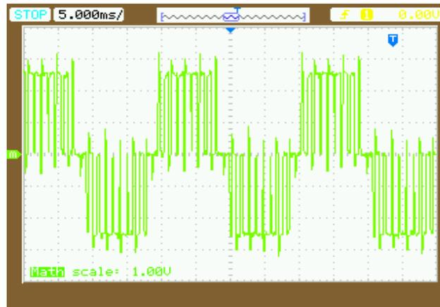
**Fig. 47.** Oscilloscope measurement of the SPWM waveform for  $f_c = 500$  Hz,  $f_s = 4$  MHz and  $M = 0.9$ .
