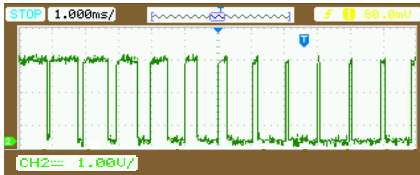
**Fig. 53.** The control signal  $T_{a+}$  ( $T_{b+}$  is produced similarly) in case that  $f_c = 1$  kHz and  $M = 0.5$ .
