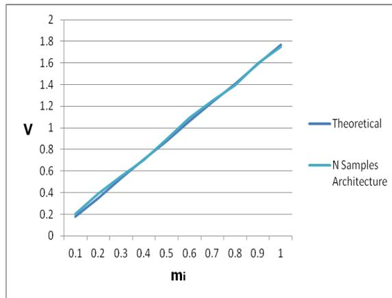
**Fig.74.** Experimental and theoretical output voltage at 50 Hz for the n samples architecture in case that  $M = 0.1-1$  and  $f_c = 10$  kHz ( $d$  ranges from 0-11.4%).
