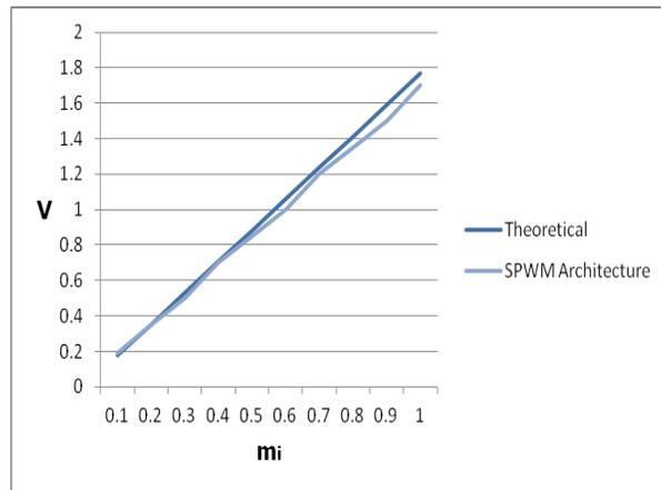
**Fig.61.** Experimental and theoretical output voltage at 50 Hz for  $M = 0.1-1$  and  $f_c = 10$  kHz ( $d$  ranges from 0-5.6%).
