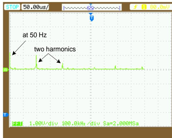
**Fig. 66.** FFT pattern for the nadir architecture ( $f_c$  max = 100 kHz,  $M = 0.5$ ).
