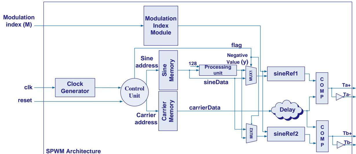
Fig. 27. The proposed SPWM generation unit architecture.
