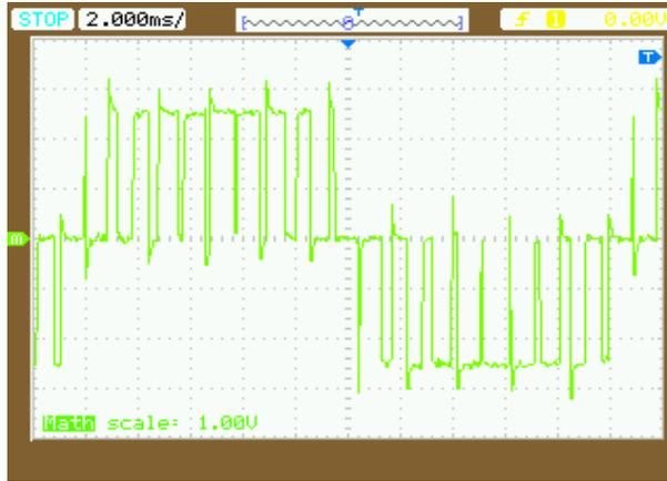
**Fig. 48.** Zoom-in oscilloscope measurement of the SPWM waveform for  $f_c = 500$  Hz,  $f_s = 4$  MHz and  $M = 0.9$ .
