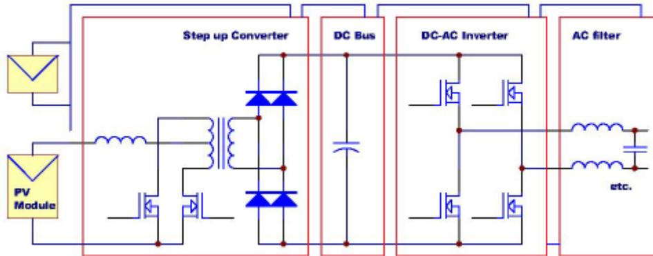
Fig. 8. Main circuit configuration of the Module Integrated Converter (MIC) topology.
