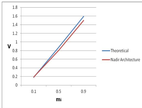
**Fig.77.** Experimental and theoretical output voltage at 50 Hz for the nadir architecture in case that  $M = 0.1, 0.5$  and  $0.9$ , respectively and  $f_c = 100$  kHz ( $d = 5.6\%, 8\%$  and  $5.7\%$ , respectively).
