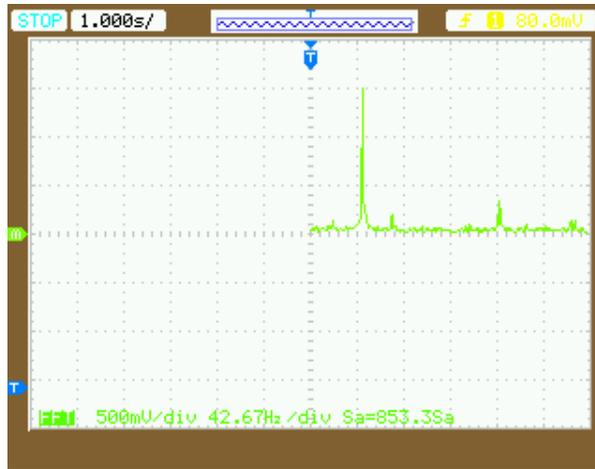
**Fig. 60.** FFT of the SPWM signal in case that  $M = 0.9$  and  $f_c = 100$  kHz.
