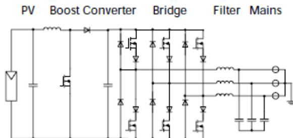
**Fig. 1.** Topology of Module Integrated Converter (MIC) with boost stage and voltage source inverter with external diodes for improved switching.
