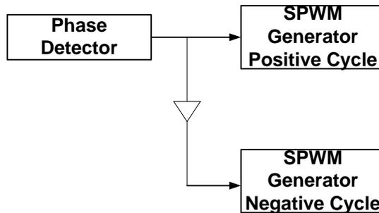
Fig. 20. Basic block diagram to generate SPWM in both cycles.
