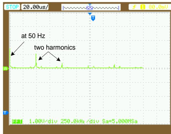
**Fig. 69.** FFT pattern for the N-samples architecture ( $f_c$  max = 250 kHz,  $M = 0.5$ ).
