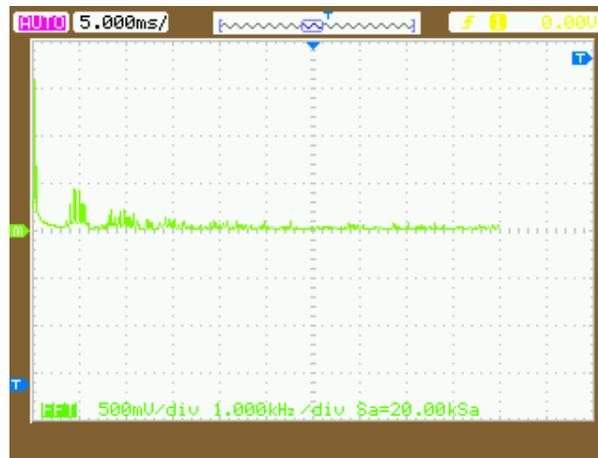
**Fig. 49.** The FFT of the SPWM signal presented in Figs. 47 & 48.
