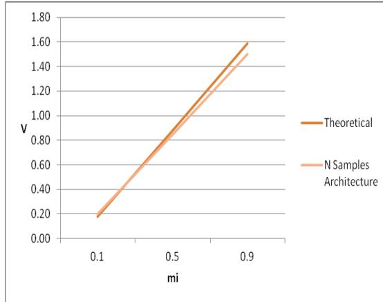
**Fig.85.** Experimental and theoretical output voltage at 50 Hz for the N-samples architecture in case that  $M = 0.1, 0.5$  and  $0.9$ , respectively and  $f_c = 250$  kHz ( $d = 11.1\%, 3.4\%$  and  $5.7\%$ , respectively).
