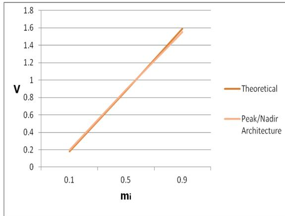
**Fig.79.** Experimental and theoretical output voltage at 50 Hz for the newly proposed architecture in case that  $M = 0.1$ , 0.5 and 0.9, respectively and  $f_c = 100$  kHz ( $d = 5.6\%$ , 8% and 5.7%, respectively).
