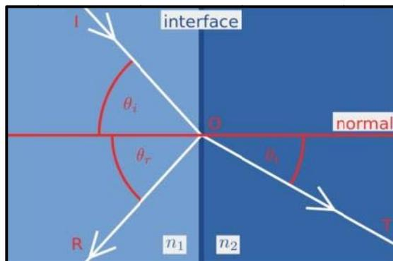
Fig. A.1. Variables used in the Fresnel equations.
