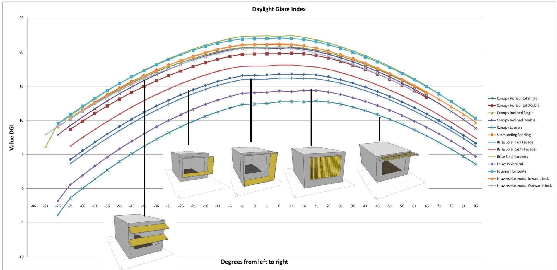
Fig. 4.15. DGI values for the 21 December at 12:00 o'clock for all examined systems in relation to the angle of view for the camera away from window
