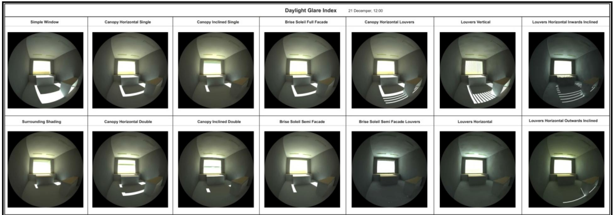
Fig. 4.17. Fish eye camera for the 21 December at 12:00 o'clock for all examined systems in relation to the angle of view for the camera away from window
