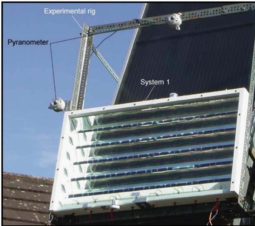
**Fig. 5.7.** Asymmetric compound parabolic PV concentrator under outdoor experimental characterization at the University of Ulster. (Mallic et al., 2004)
