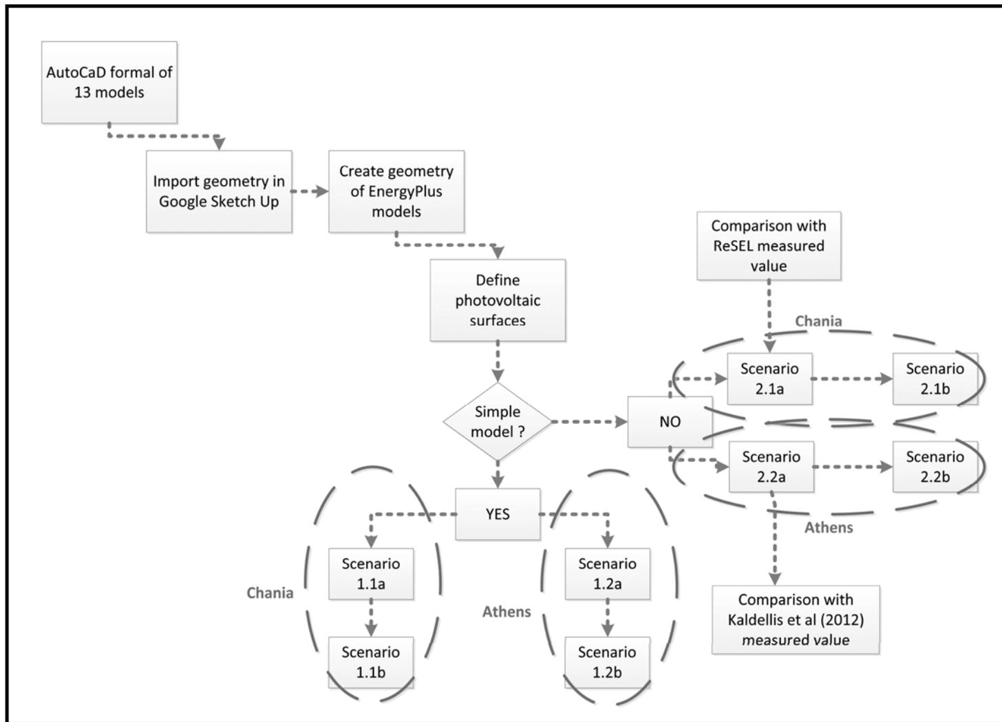
Fig.5.11. Methodological diagram of method used for evaluating the performance PV integrated shading system
