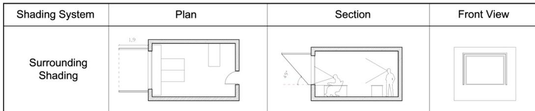
Fig.3.33. Plan, section and Front view of Surrounding shading System
