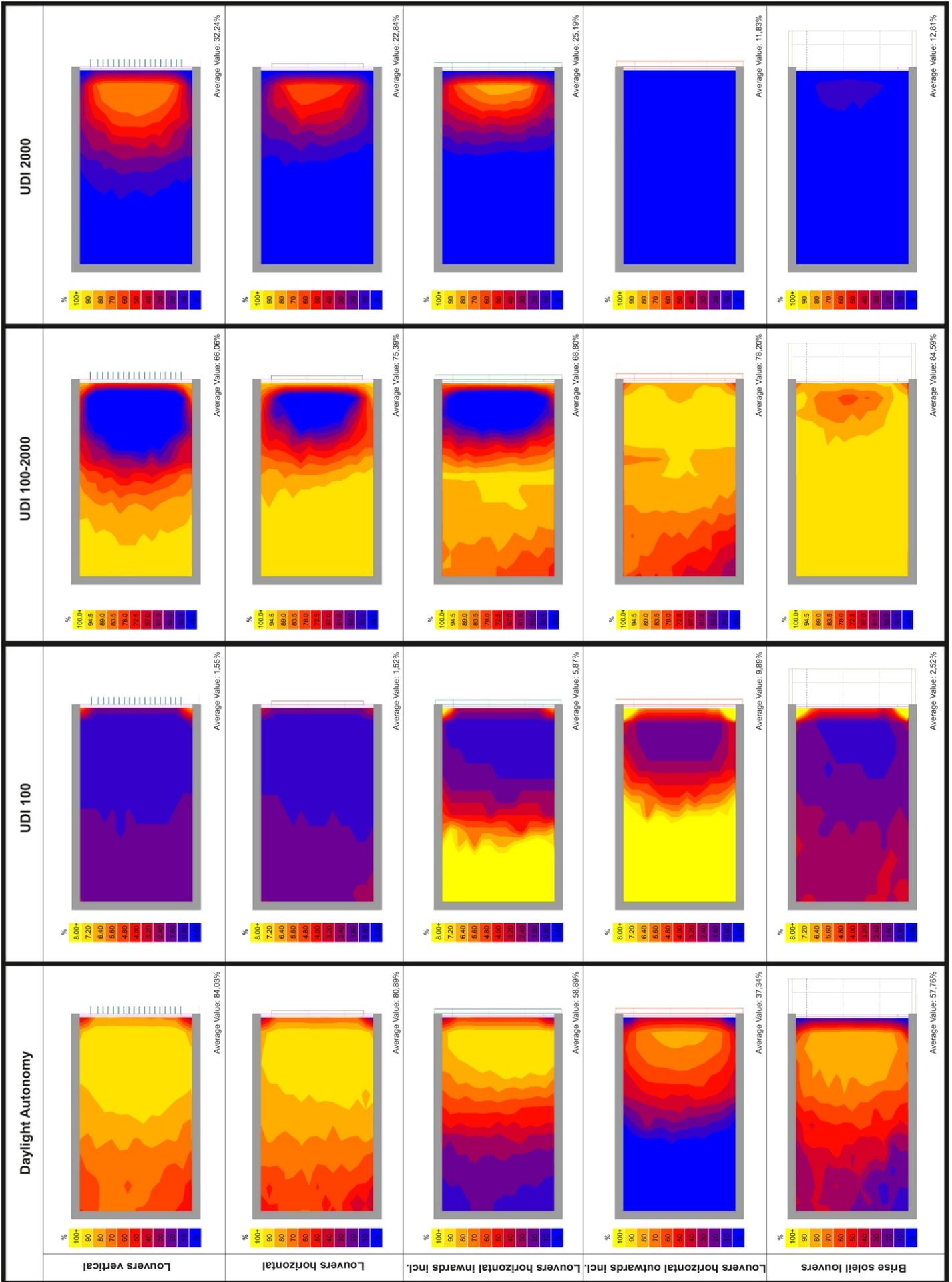
Simulations with Daysim for louver systems of 1.5 cm thick
