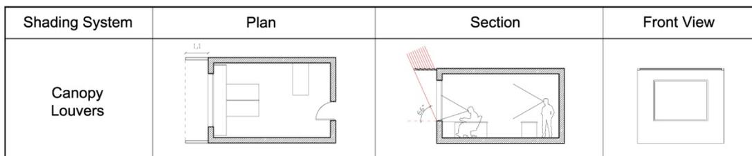
Fig.3.34. Plan, section and Front view of Canopy Louvers shading System
