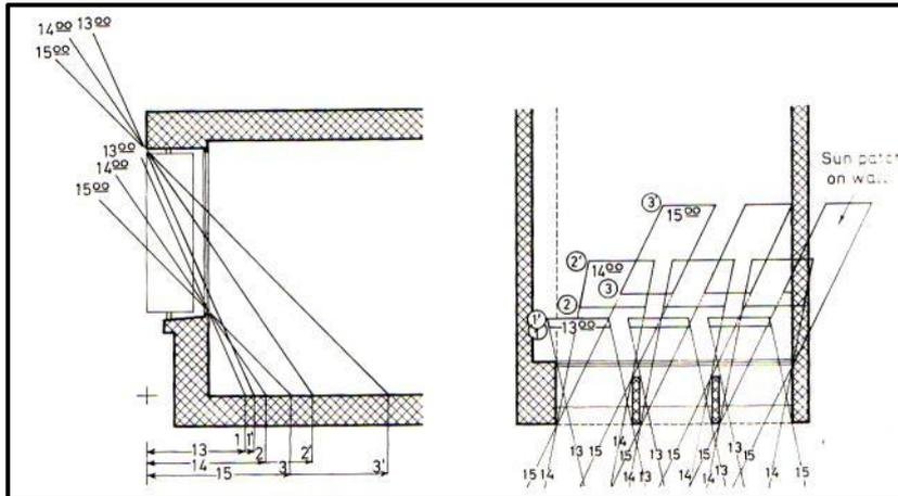
**Fig.2.10.** Graphical determination of solar radiation penetration through a window and a fixed shading device as proposed by B. Givoni (1969, p. 228)
