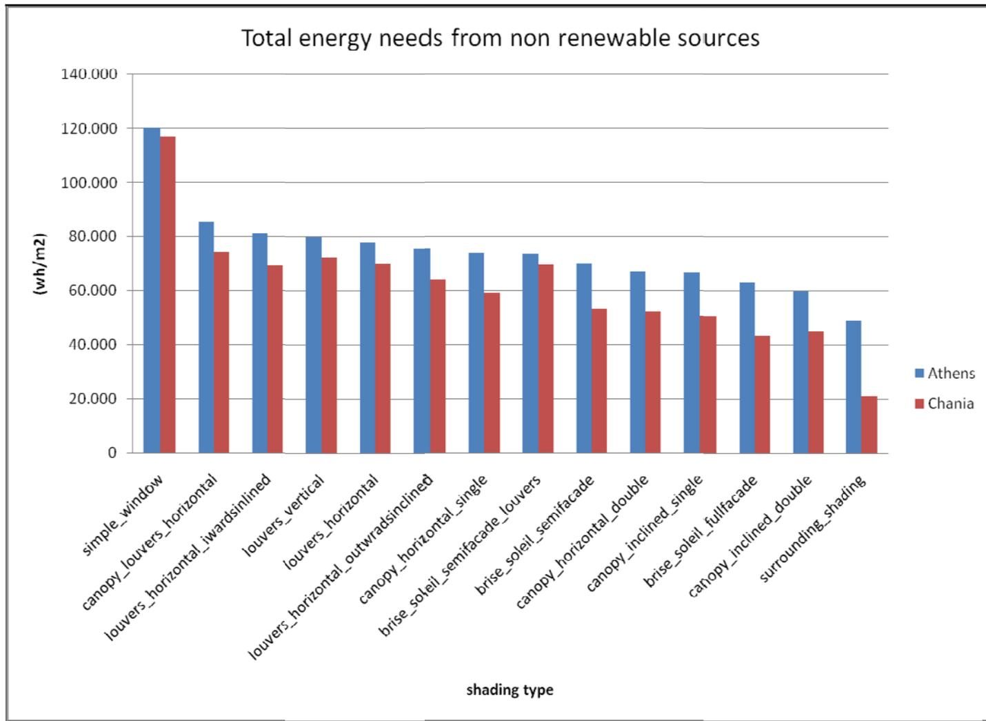
Fig.6.4. Total energy needs (heating, cooling, and lighting) for Athens and Chania
