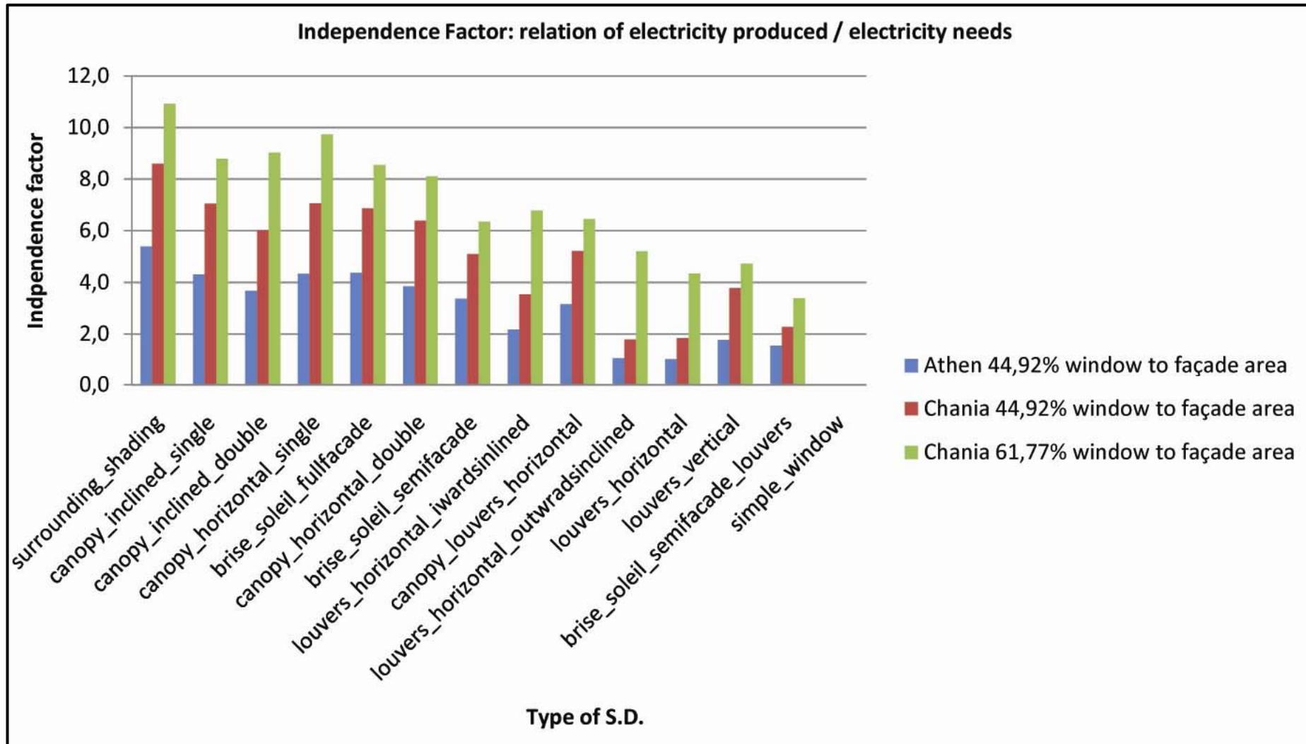
Fig. 6.3. Relation of electricity produced to electricity needs
