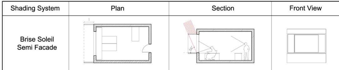
Fig.3.32. Plan, section and Front view of Brise Soleil Semi Facade shading System
