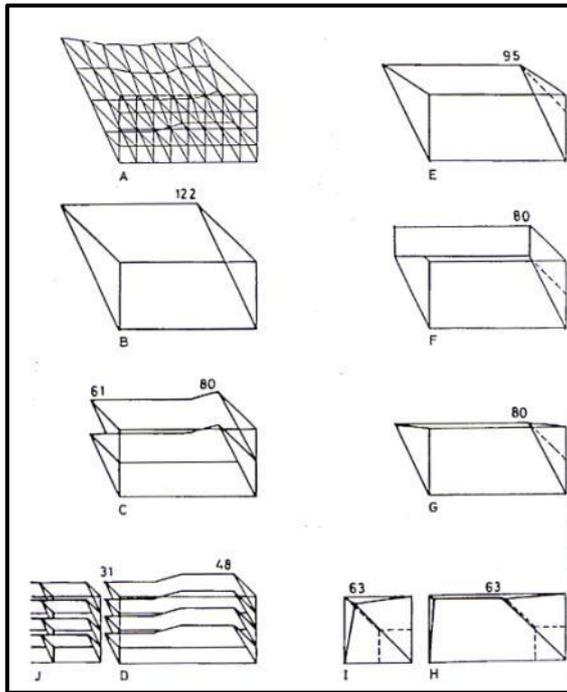
**Fig.2.11.** Axonometric projection of  $L_{max}$  for a southern window and shading for the period March 21 till October 21, for hours 08.00 – 16.00 in Tel Aviv (Latitude 32°N) – and alternatives for different geometrical configurations of Sun shades. (Shaviv, 1975, p. 140)
