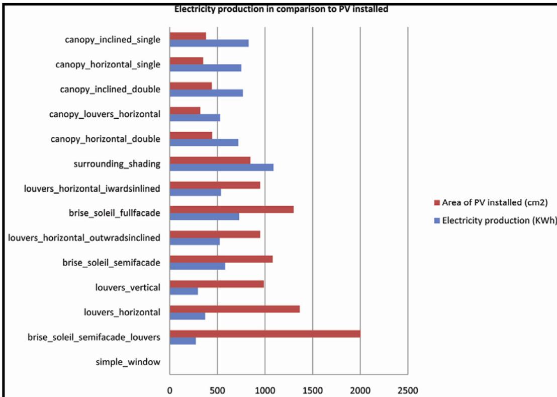
Fig.5.14. Electricity production in comparison to area of PV installed for Chania with window 44.92% of facade area.
