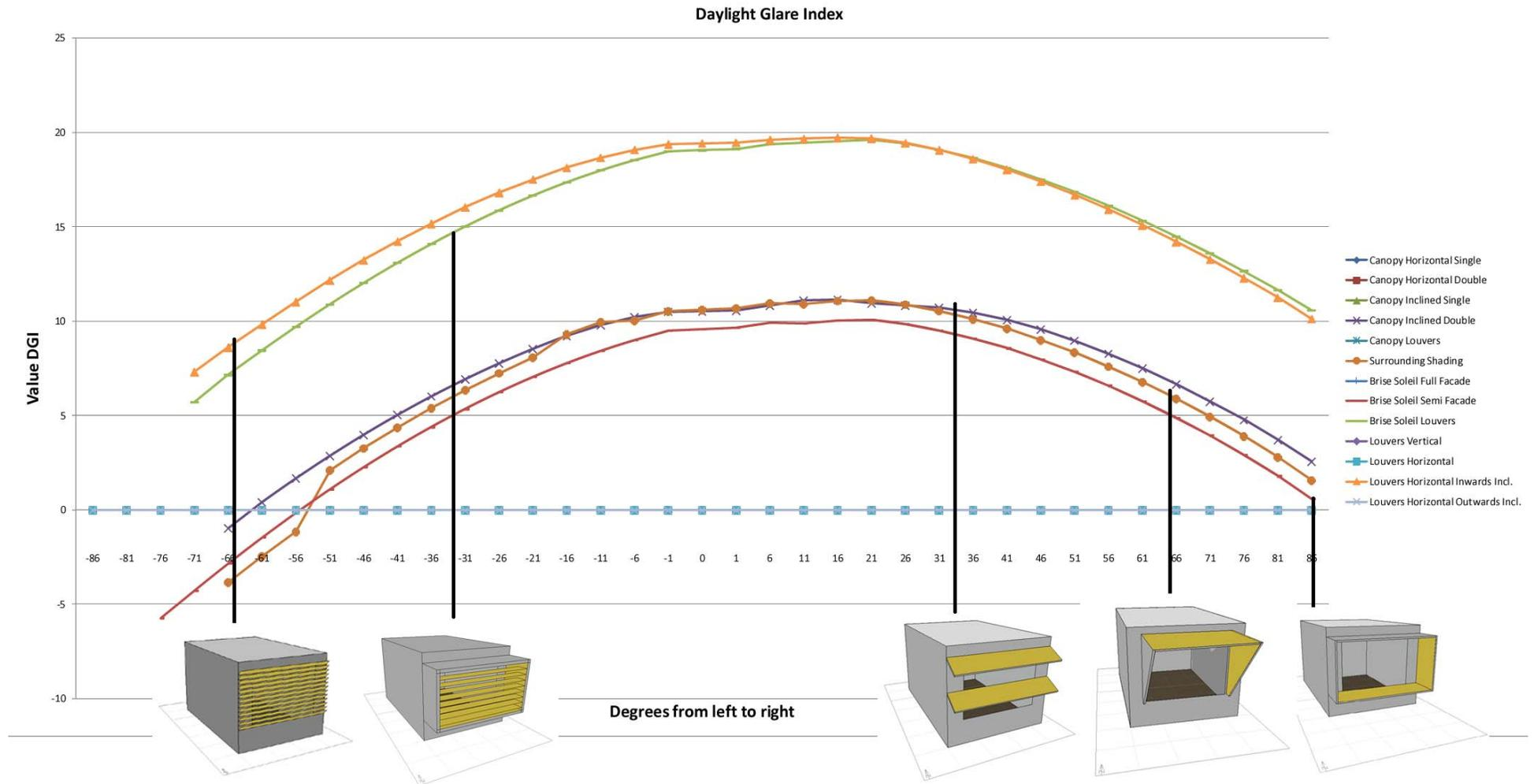
Fig.4.19. DGI values for the 21 December at 12:00 o'clock for all examined systems in relation to the angle of view for camera near the window.
