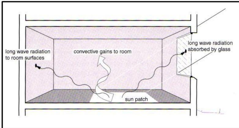
**Fig.2.2.** *The mechanism of solar heat gain: short wave radiation transmitted through the glass and absorbed by the surfaces in the room, where it is converted to heat. The glass is opaque to long wave radiation from warm surfaces. The rooms' surfaces also lose heat to the air by convection. The process is called "the greenhouse effect".*
