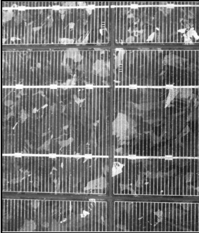
**Fig. 5.5.** Blue Pattern Polycrystalline silicon cells (Lechner, 2001)
