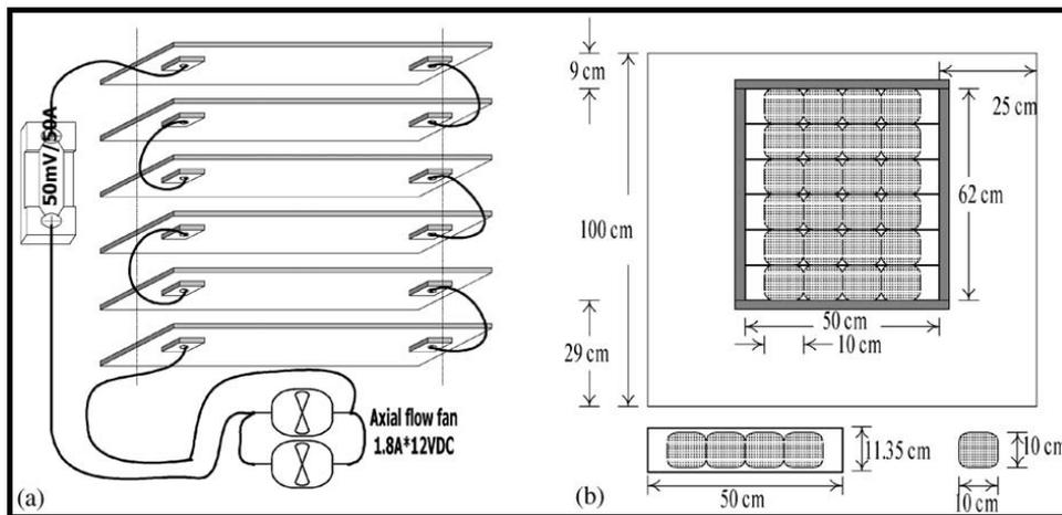
**Fig. 5.9.** (a) The PV-slats window configuration and (b) the southern wall of lab-scale testing room with the PV-SW (Khedaria, J., Waewsakb,J., Suphengc, W., Hirunlabha, J., 2004)
