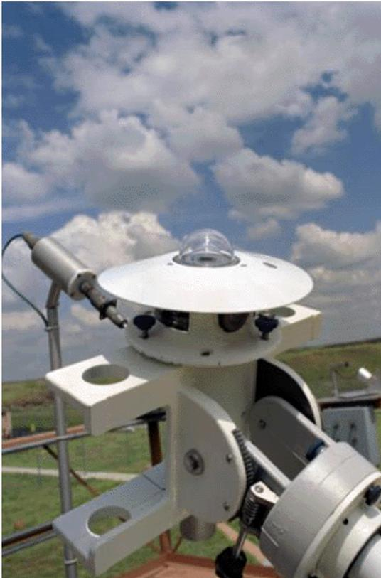
**Fig.3.14.** Instrument for solar irradiance measurements) via NREL information exchange (<http://pveducation.org/pvcdrom/properties-of-sunlight/measurement-of-solar-radiation>)
