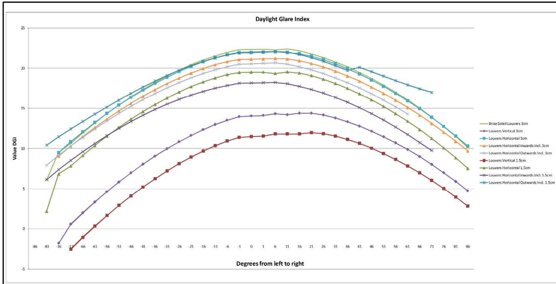
Fig. 6.9. Comparison of DGI values for the case of thickness 1.5 and 3 cm for camera away from the window for the 21<sup>st</sup> December at 12.00 o'clock
