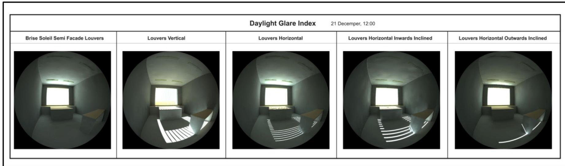
Fig. 6.10. Fish – eye camera for 1.5 cm thickness systems for December 21<sup>st</sup> at 12:00
