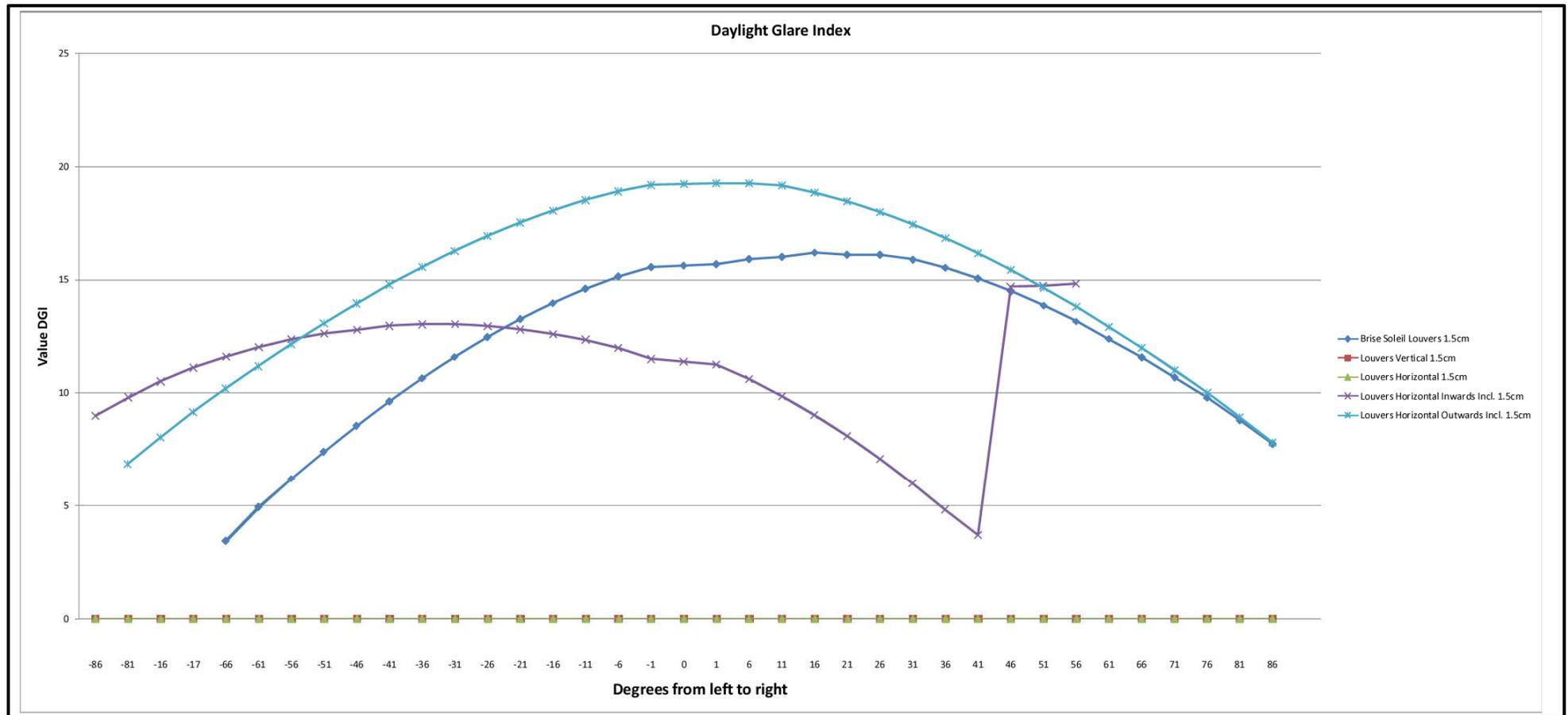
Fig. 6.11. DGI values for SDs for the case of thickness 1.5 and 3 cm for camera near the window for the 21<sup>st</sup> December at 12.00 o'clock
