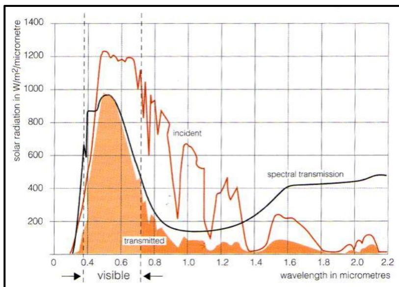
**Fig.2.1.** The radiation spectrum of sunlight: about one half of the energy is in the visible region, the remainder is found in the infrared and ultraviolet zone. The transmission curve of the clear glass shows that some of the invisible radiation is absorbed by the glass. (Baker & Steemers, 2001, p. 110)
