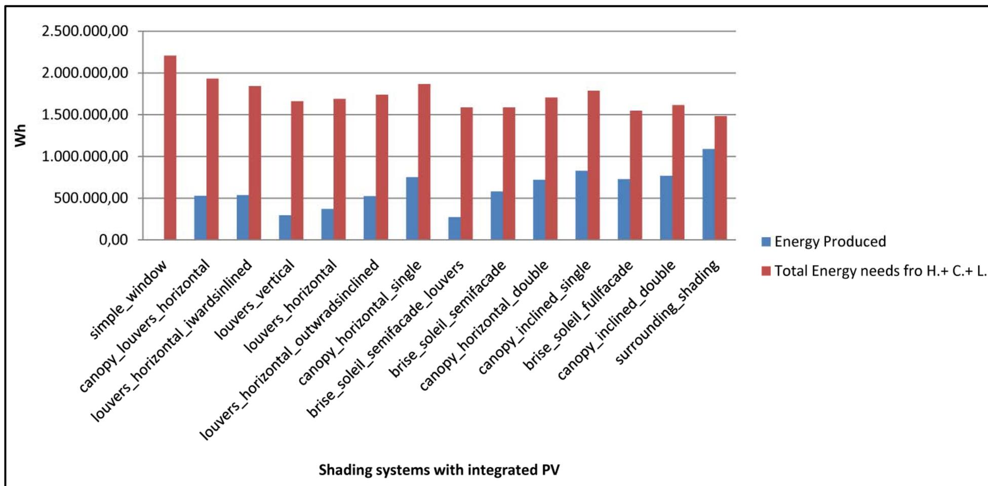
Fig.7.2. Energy production and energy needs of the office unit with various shadings systems in the south façade
