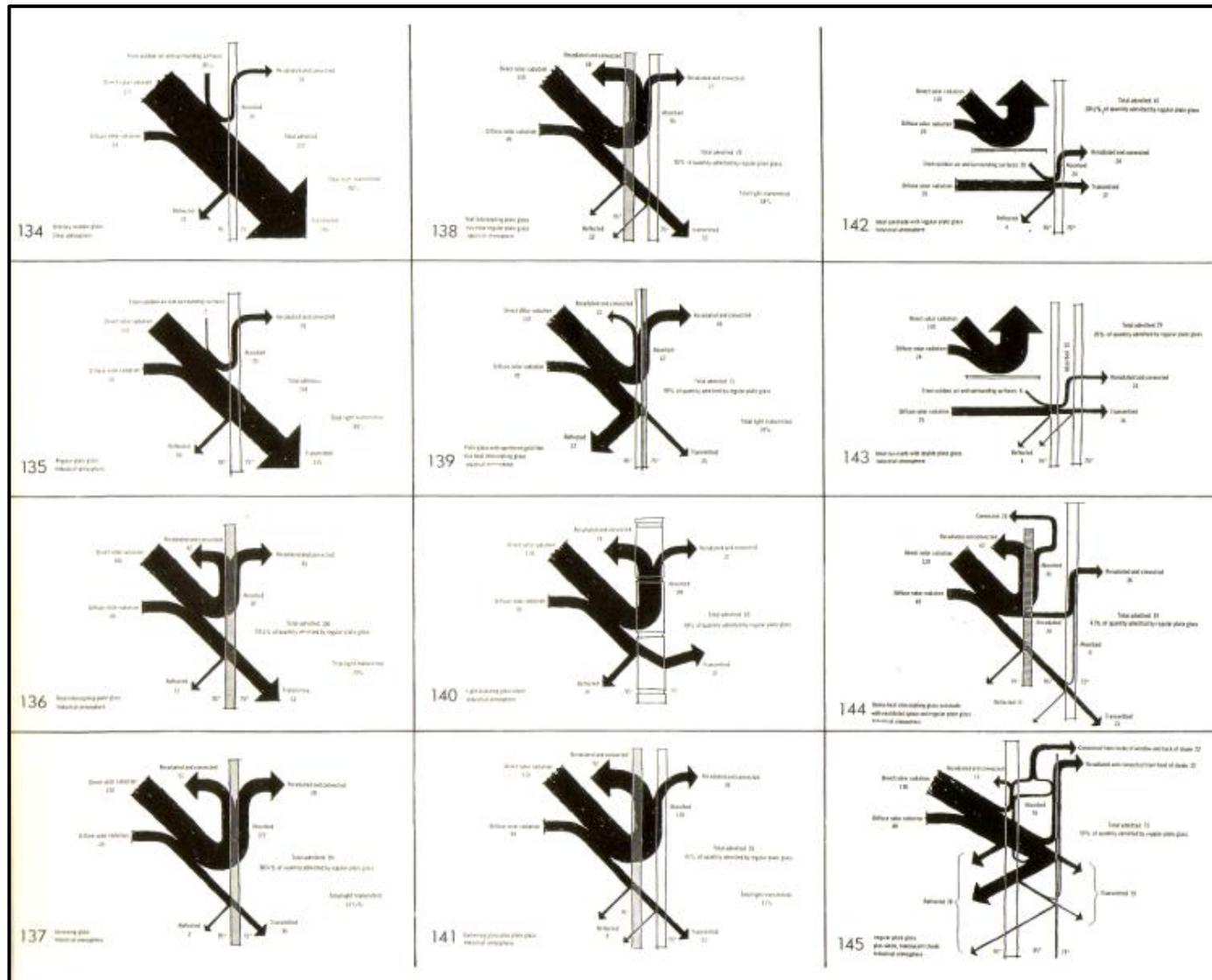
Fig.2.7. Heat gain through different types of glass and different types of shadings (Olgay, A. & V., 1957, p. 71)
