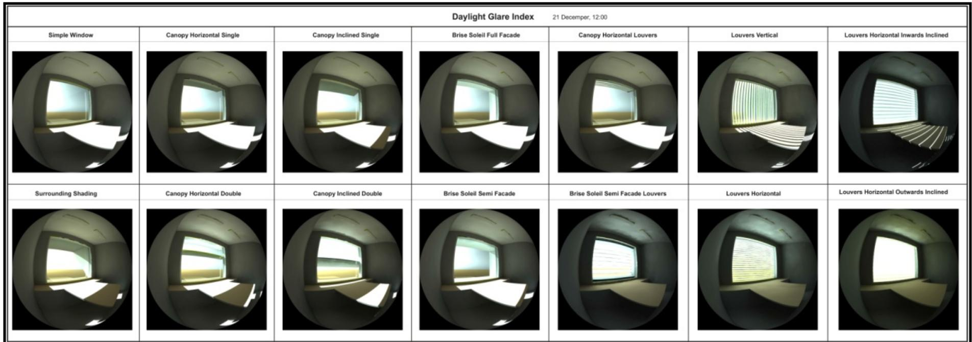
Fig. 4.20. Fish eye camera for the 21 December at 12:00 o'clock for all examined systems in relation to the angle of view for camera near the window
