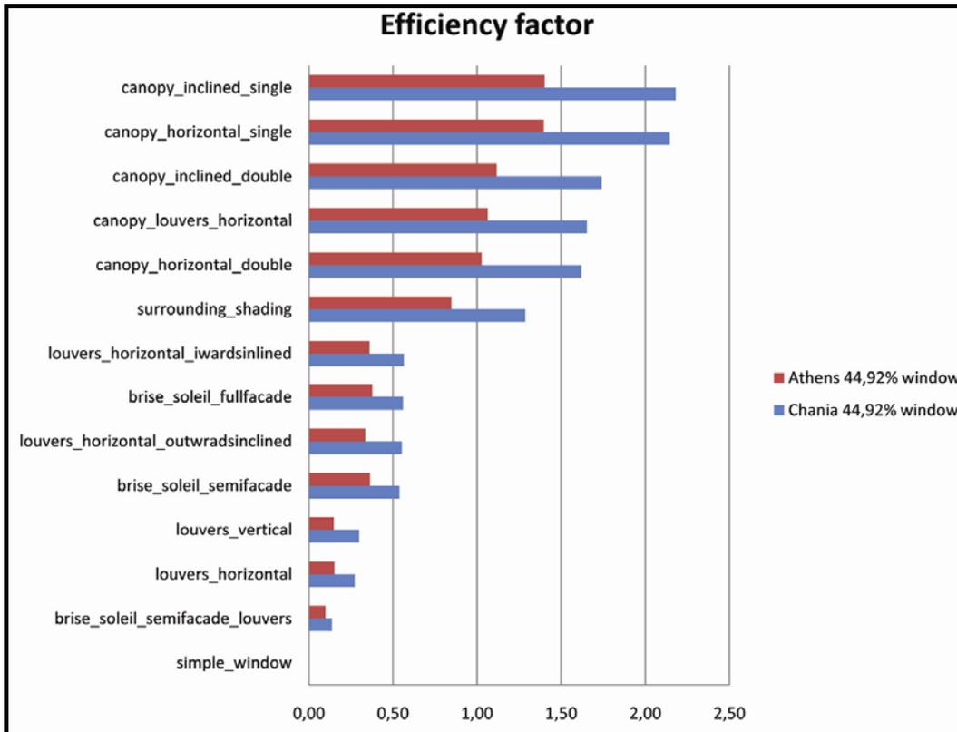
Fig. 5.13. Efficiency factor for Chania and Athens with window 44.92% of facade area
