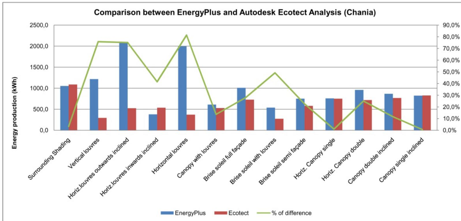
Fig.5.16. Comparison between EnergyPlus and Autodesk Ecotect Analysis (for the Area of Chania)
