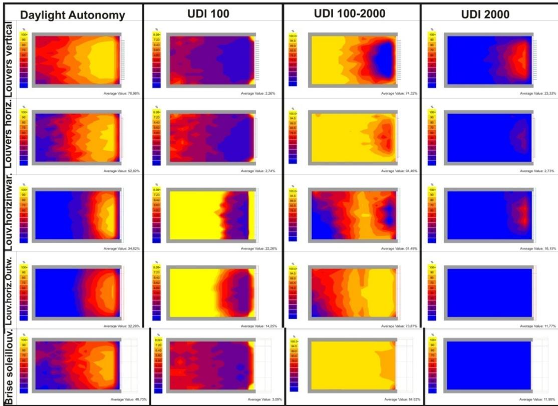
Fig. 6.12. DA and UDI values for Louver Systems with 3 cm thickness
