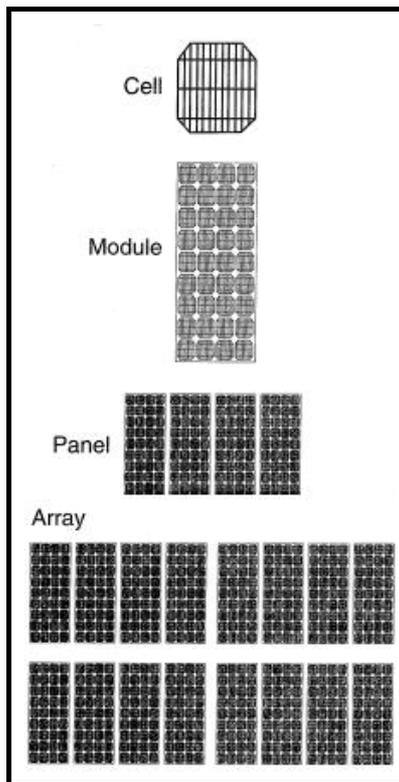
**Fig.5.1.** Cell combined to form modules, modules form panels, and panels combine to form an array (Lechner, 2001)
