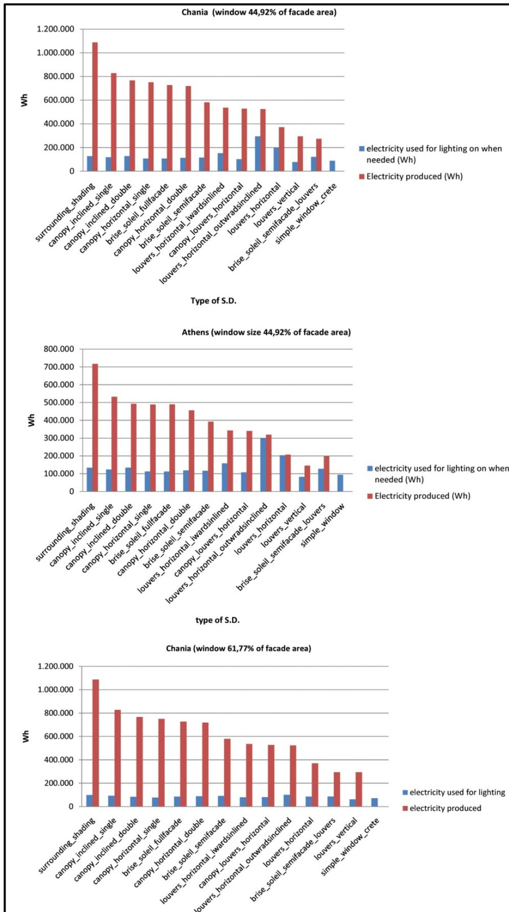
Fig. 6.2. Relation of electricity production to electricity needs
