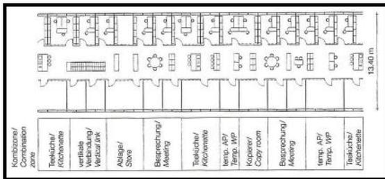
**Fig. 3.18.** Diagrammatic plan of combination offices (Stanier, B. & C., 2011)
