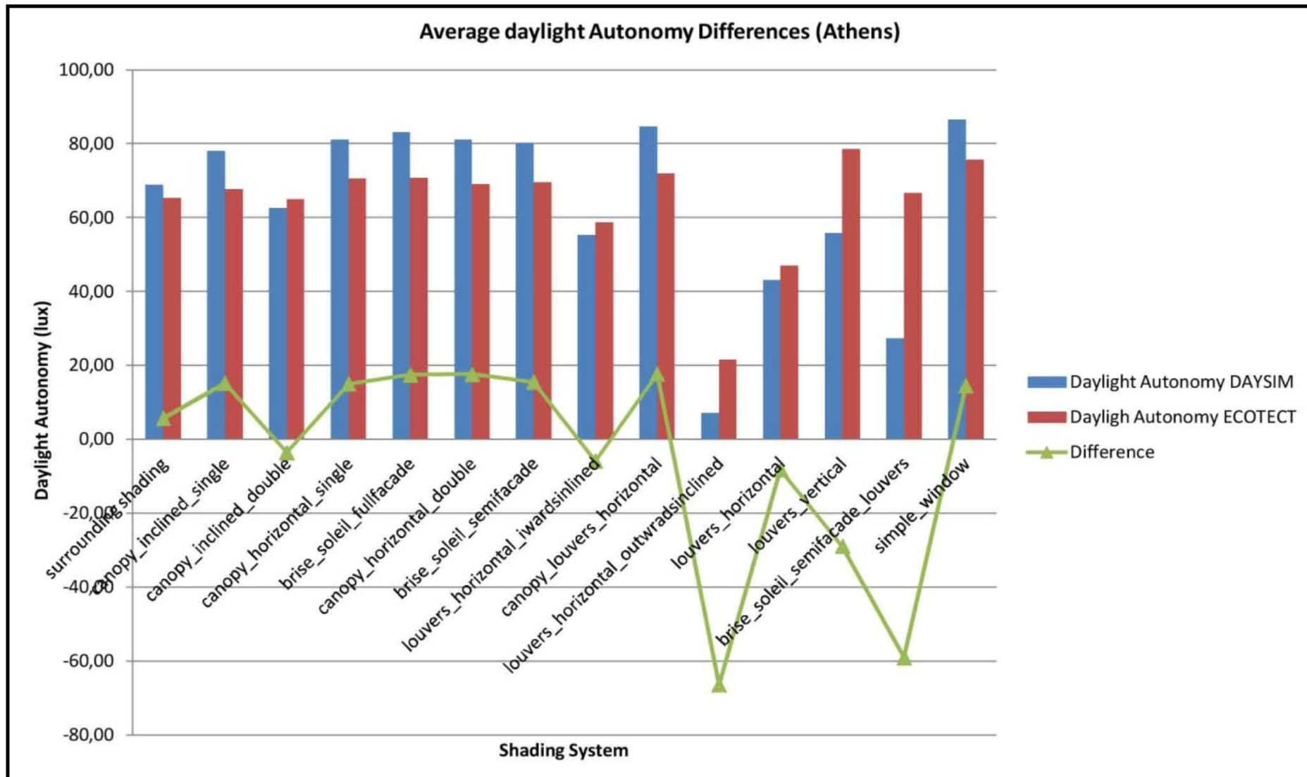
Fig. 4.11. Difference of calculated DA for Athens Latitude between Daysim and Ecotect application software
