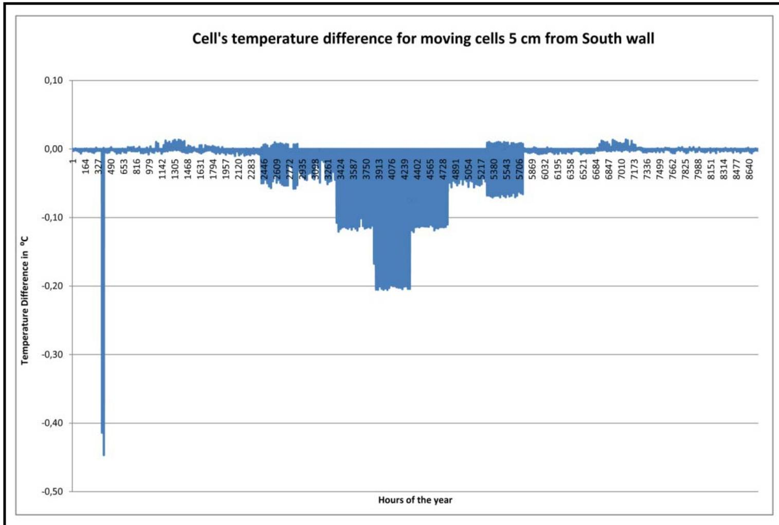
**Fig.5.21.** Cell's temperature difference when moving cells 5 cm from south wall for Canopy Inclined Double simulated with Sandia PV models for Chania
