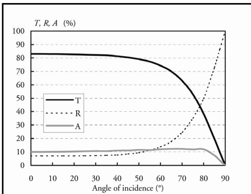
**Fig.3.7.** The angle dependence of transmittance, reflectance and absorption of clear float glass for incidence angle  $\theta$  (from the surface normal) (Bulow - Hube, 2001, p. 61)
