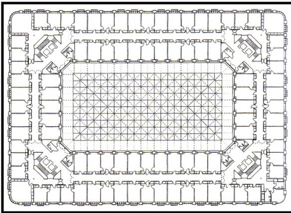
**Fig. 3.15.** Diagrammatic plan of office units
