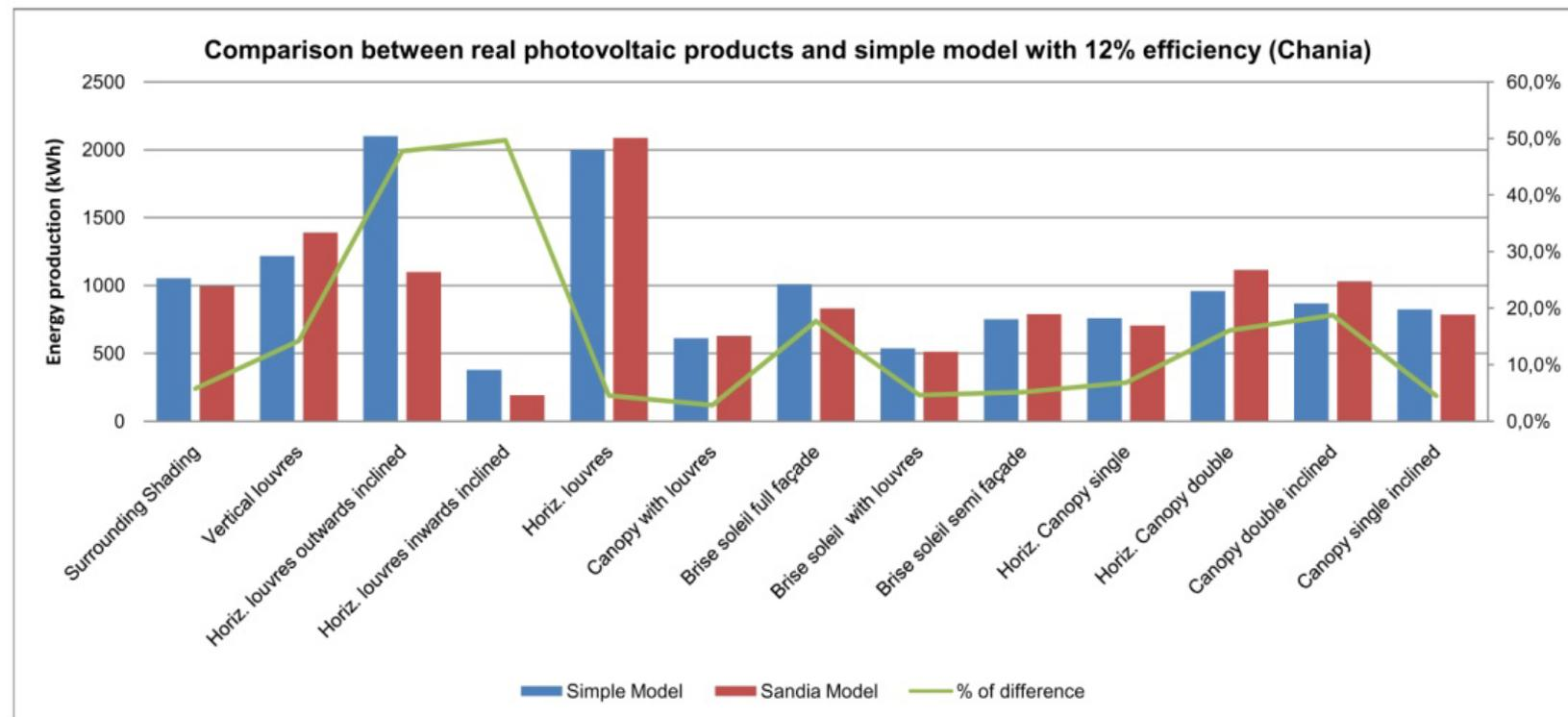
Fig. 5.17. Comparison between real PV products and a simple model with 12% efficiency (Chania)
