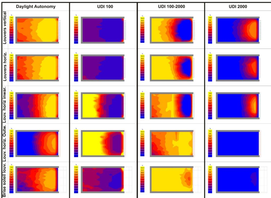
Fig. 6.13. DA and UDI values for Louver Systems with 1.5 cm thickness
