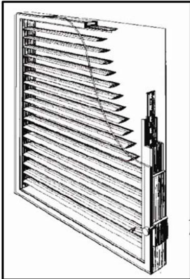
**Fig.2.9.** Isometric view of an Inter-pane venetian blind system (Olbina, 2005, p. 96)
