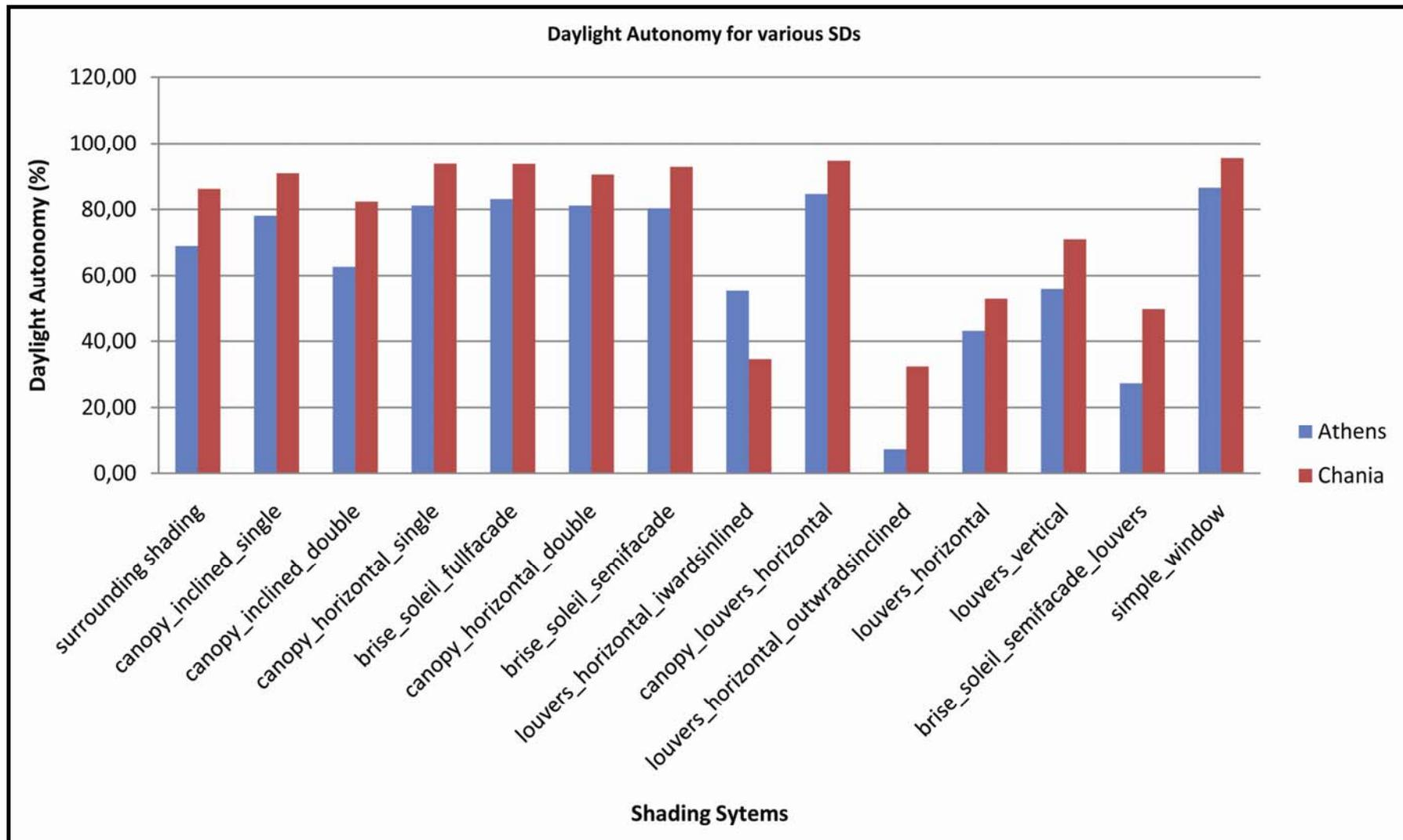
Fig.4.10. Comparison of Daylight Autonomy for Athens and Chania
