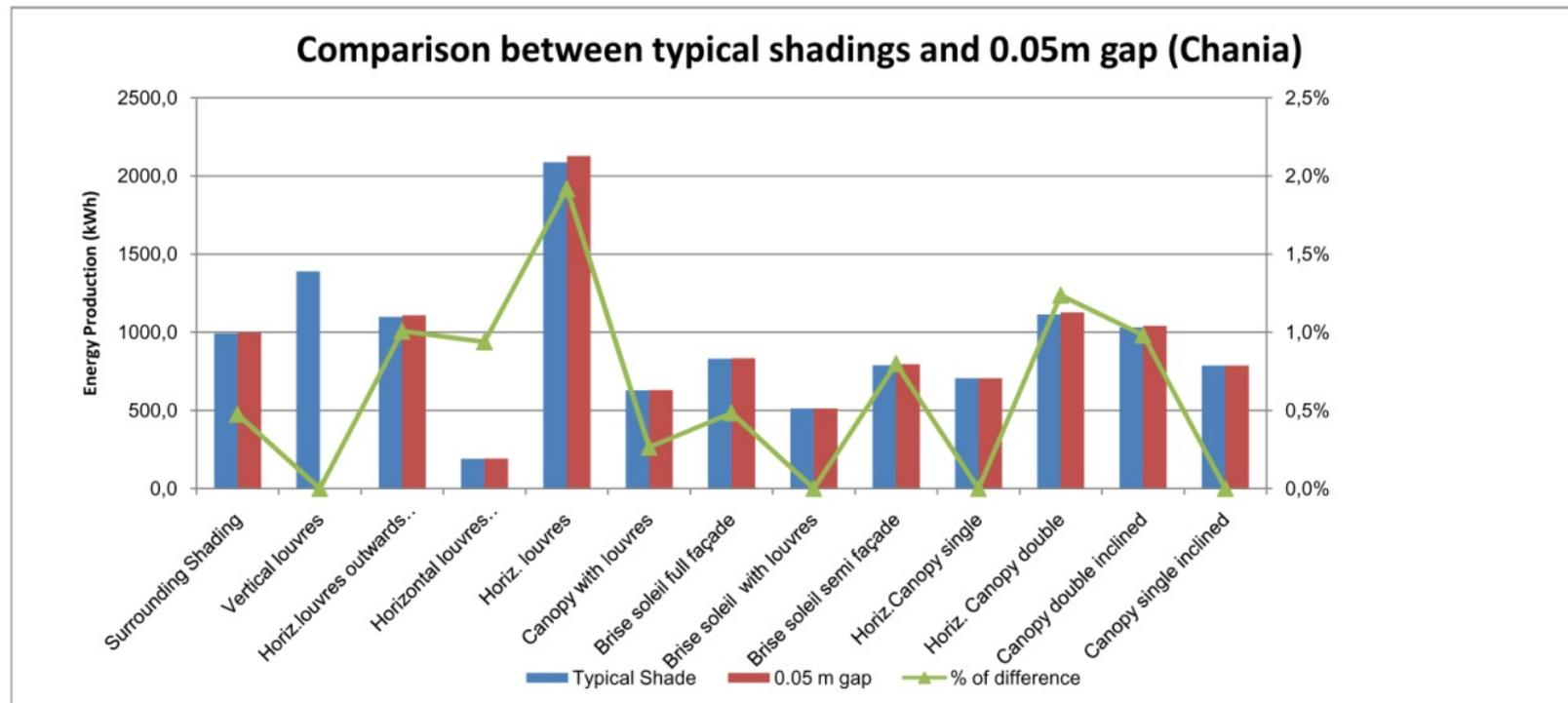
Fig.5.19. Comparison between typical shadings and 0.05m gap (Chania)
