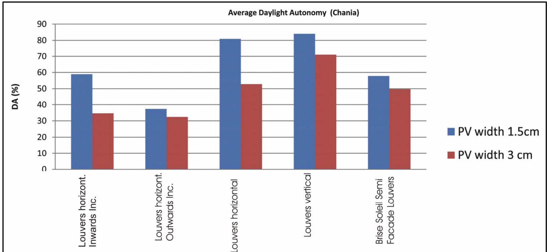
Fig. 6.8. Comparison of DA for two PVs' thickness (1.5 and 3 cm)
