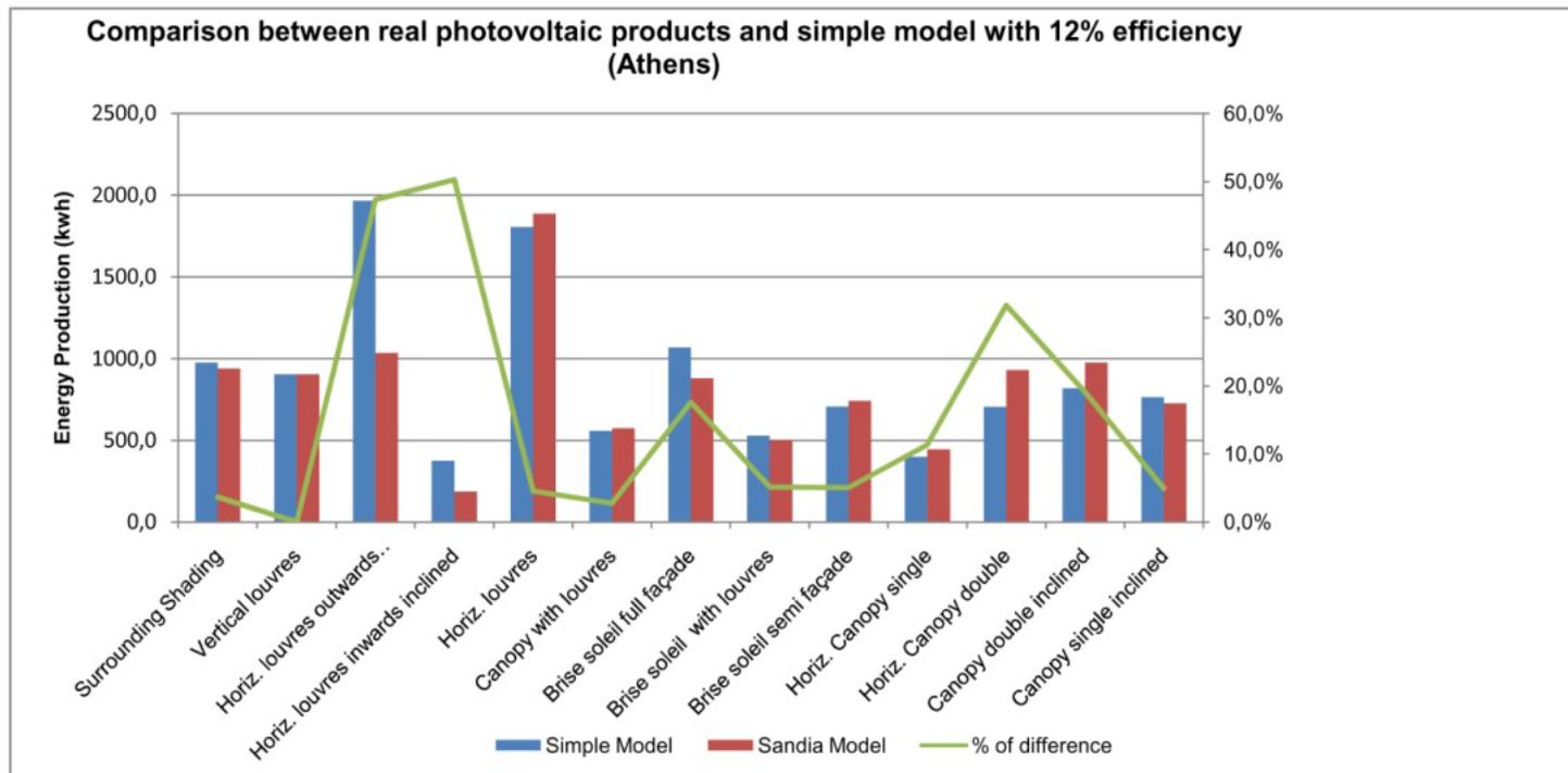
Fig. 5.18. Comparison between real PV products and a simple model with 12% efficiency (Athens)
