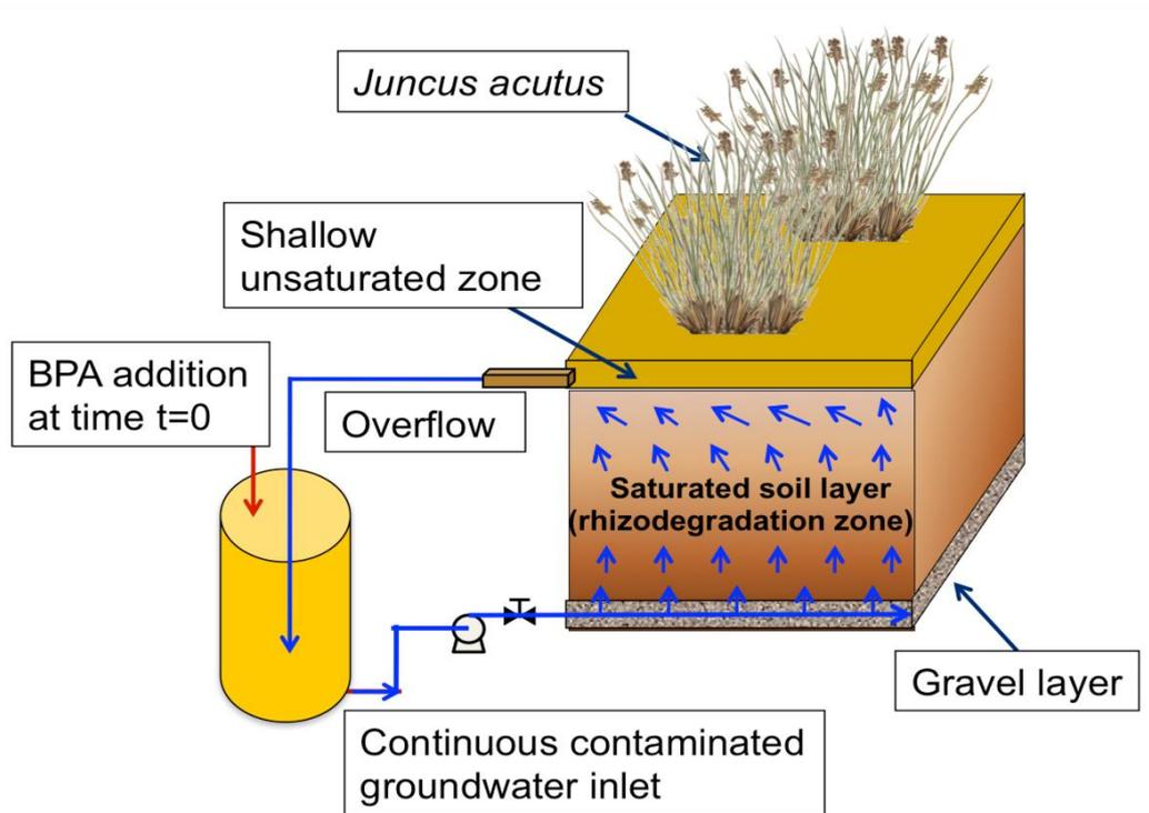
Figure 3. Schematic representation of the Shallow Aquifer Phytoremediation Pilot, planted with two *Juncus acutus* plants.
