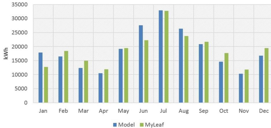
**Figure 12: HVAC system validation based on monthly electrical energy consumption**
