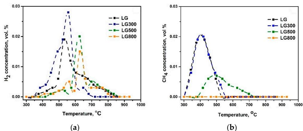
**Figure 9.**  $\text{H}_2$  (a) and  $\text{CH}_4$  (b) evolution profiles for raw lignite and chars during non-isothermal  $\text{CO}_2$  gasification. Fuel: 100 mg, Flowrate:  $30 \text{ cm}^3/\text{min}$ .
