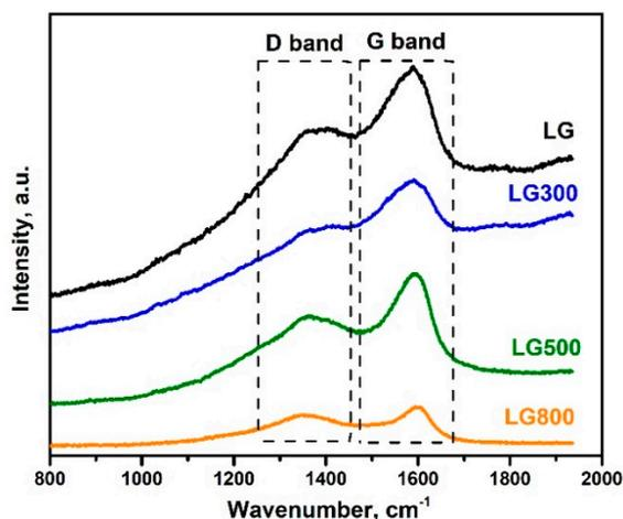
**Figure 2.** Raman spectra of raw lignite and as-produced chars.
