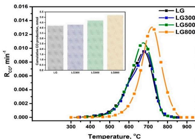
**Figure 7.** Effect of temperature on the instant CO production rate,  $R_{CO}$ , and the cumulative CO production (inset) for raw lignite and chars during non-isothermal  $CO_2$  gasification. Fuel: 100 mg, Flowrate:  $30 \text{ cm}^3/\text{min}$ .
