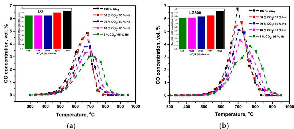
**Figure 10.** Effect of CO<sub>2</sub> feed concentration on CO evolution profiles and overall CO production (inset) for raw lignite (a), and LG800 (b) samples. Fuel: 100 mg, Flowrate: 30 cm<sup>3</sup>/min.
