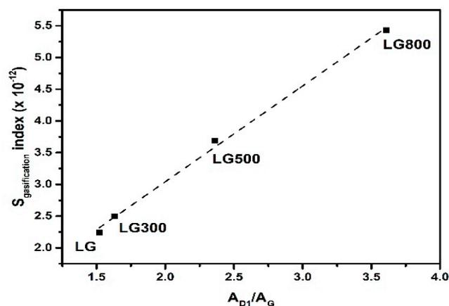
**Figure 6.** Relationship between the comprehensive characteristic gasification index ( $S$ ) and  $A_{D1}/A_G$  ratio.
