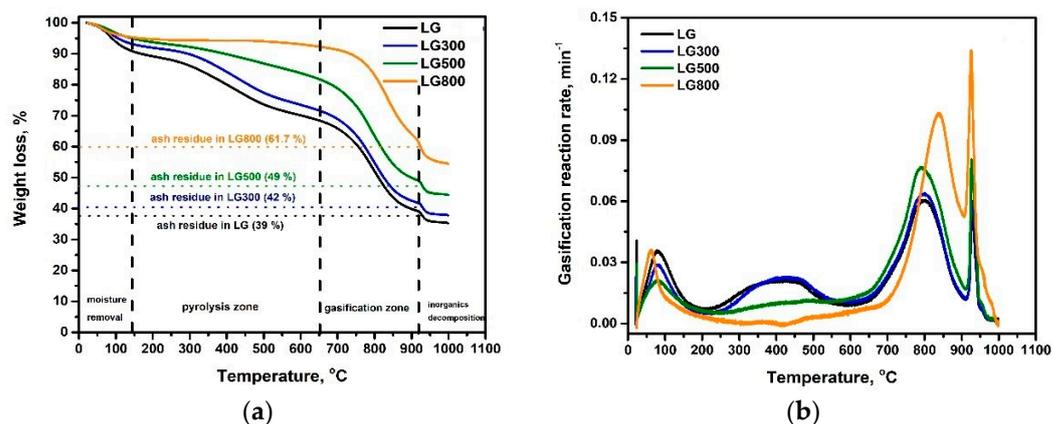
**Figure 5.** Non-isothermal thermogravimetric analysis (a), and instant gasification rate (b), for raw lignite and chars under pure CO<sub>2</sub> atmosphere.
