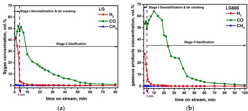
**Figure 11.** Syngas composition with time on stream for LG (a) and LG800 (b)  $CO_2$  gasification at 800 °C. Fuel: 500 mg, Flowrate: 30  $cm^3/min$ .
