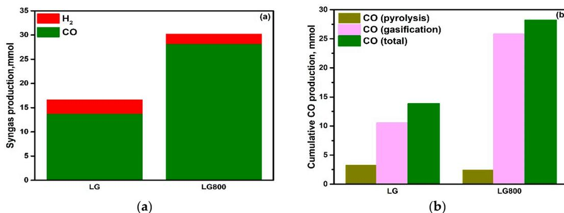
**Figure 12.** Syngas production (a), and shares of pyrolysis and gasification steps to the overall CO production for LG and LG800 (b) during isothermal CO<sub>2</sub> gasification tests at 800 °C. Fuel: 500 mg, Flowrate: 30 cm<sup>3</sup>/min.
