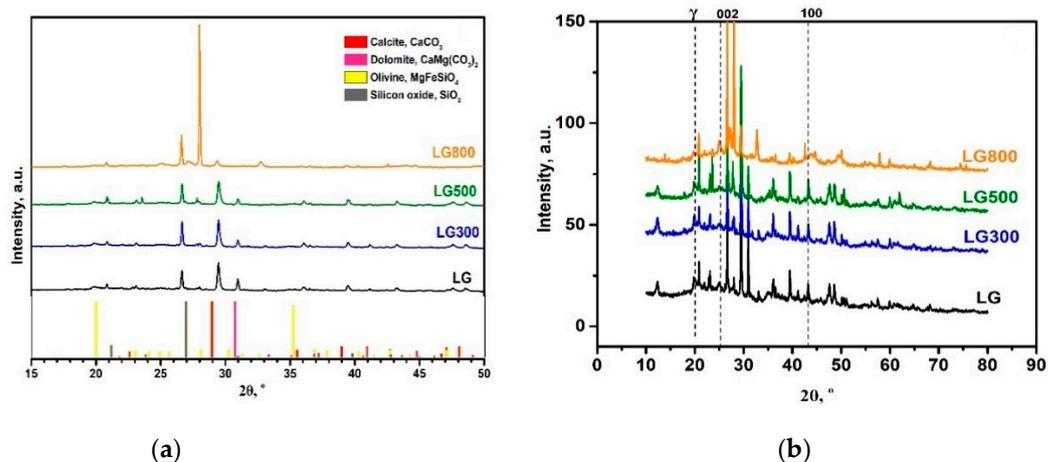
**Figure 1.** XRD patterns of pristine lignite and as-produced chars (a), closer inspection of XRD patterns (b).
