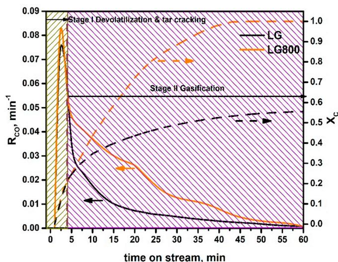
**Figure 13.** Instant CO production rate and the corresponding carbon conversion vs. time on stream for LG and LG800 samples under isothermal CO<sub>2</sub> gasification at 800 °C. Fuel: 500 mg, Flowrate: 30 cm<sup>3</sup>/min.
