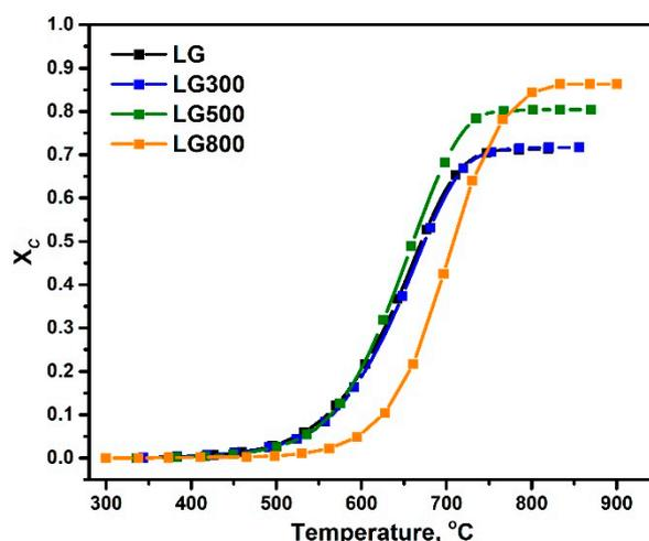
**Figure 8.** Effect of temperature on carbon conversion for raw lignite and chars during non-isothermal  $\text{CO}_2$  gasification. Fuel: 100 mg, Flowrate:  $30 \text{ cm}^3/\text{min}$ .
