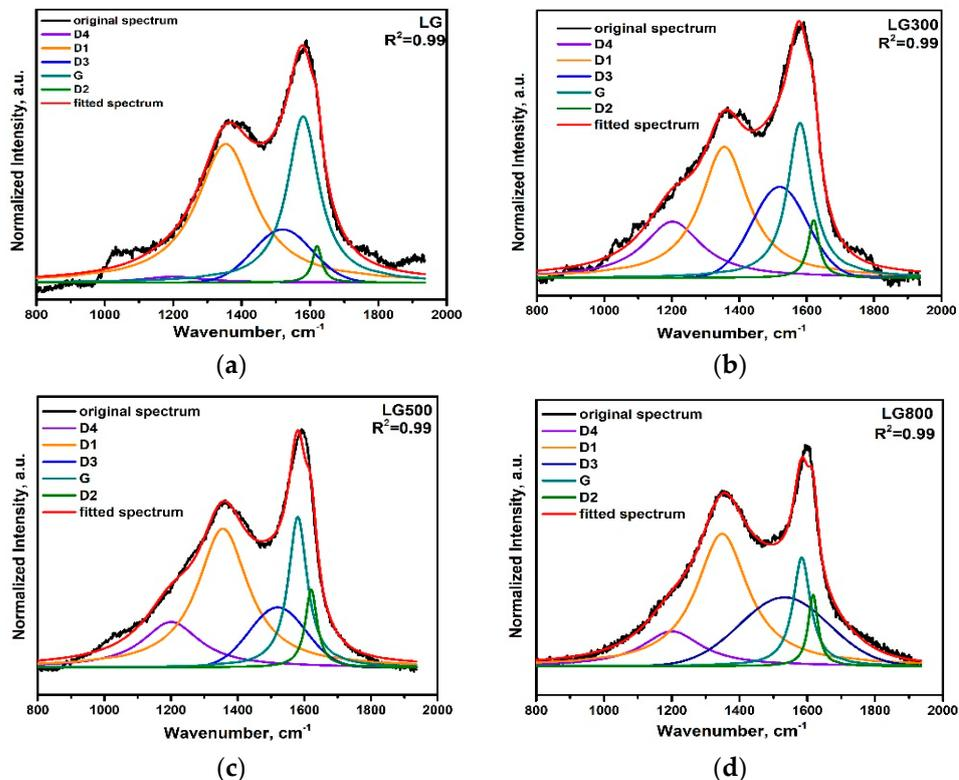
Figure 3. Curve fitting of Raman spectra for raw lignite and as-produced chars.
