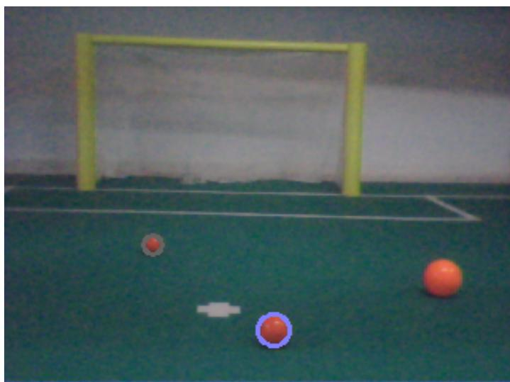
(b) Three balls seen, two correct, nearest selected. Posts erroneously rejected.
