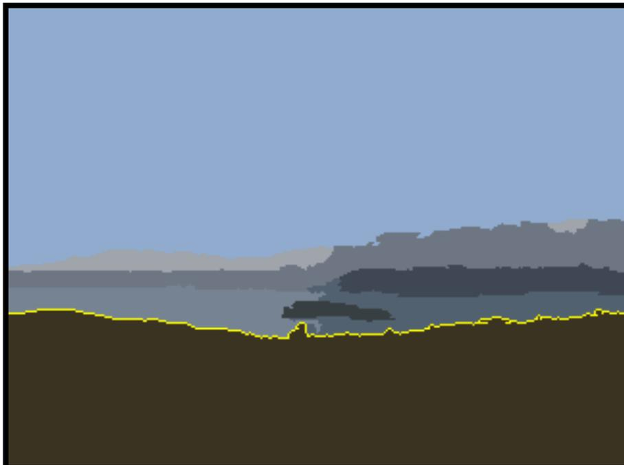
**FIGURE 24: DETECTION OF A SINGLE LAND REGION AND EXTRACTION OF THE COASTLINE**
