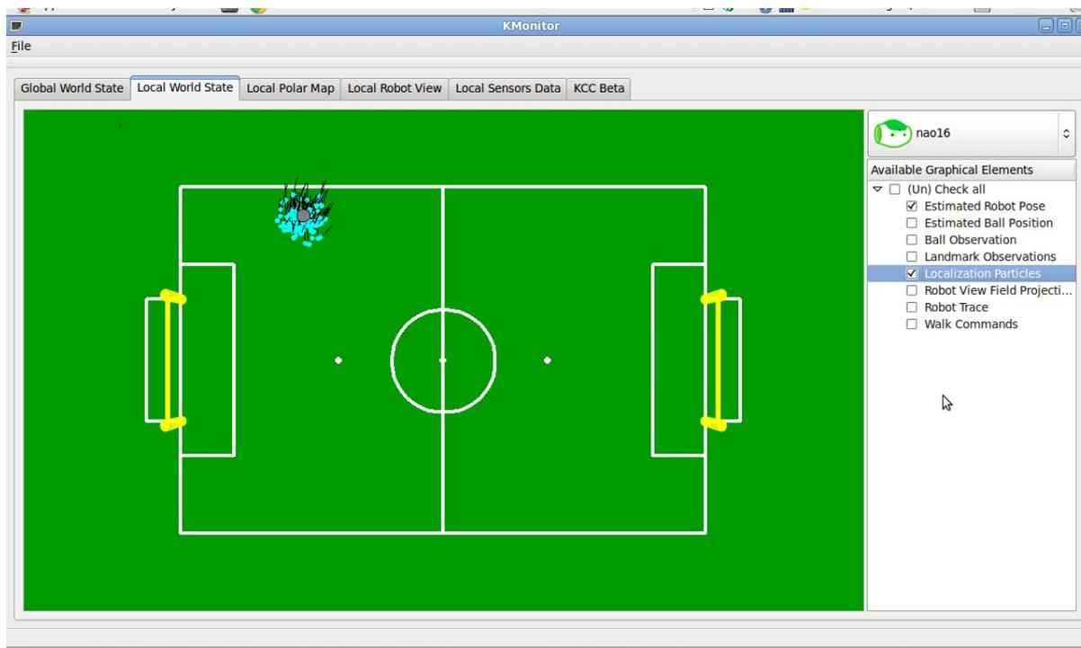
Figure 5.14: Visualization of the localization particles
