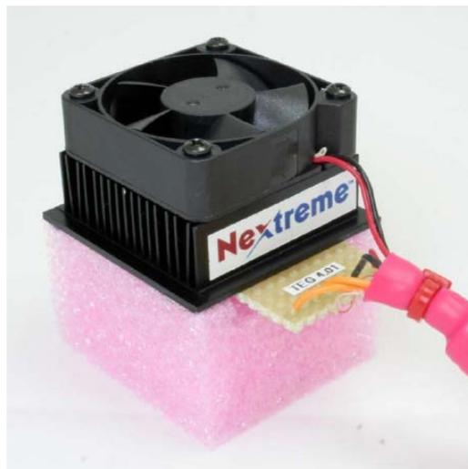
**Fig. 4.4** The Nextreme eTEG HV56 power generator evaluation kit [20].
