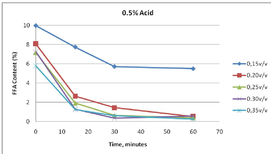
Fig 6. 2- Effect of reaction time and methanol quantity on reduction of FFA value of palm oil for 0.5% v/v, acid-to-oil ratios during pretreatment for biodiesel production (initial FFA value = 8.28%)
