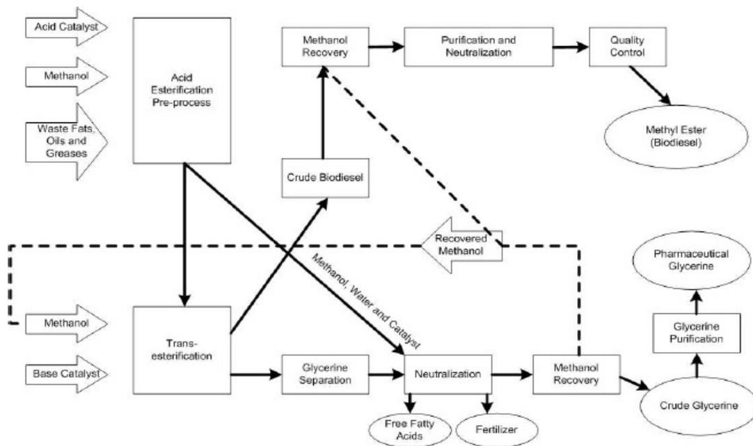
**Fig 4.8 Biodiesel process flow diagram using low-high FFAs feedstock**
