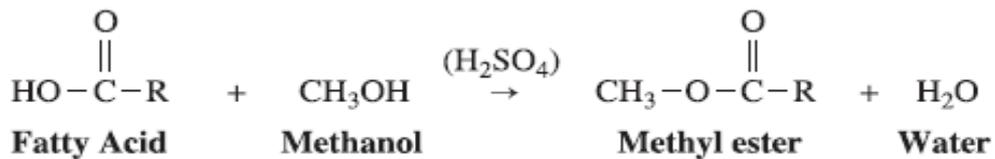
Fig 6.1- Esterification of FFAs (Van Gerpen, 2005)
