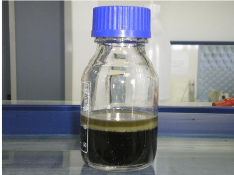
Fig 6. 1 - COPO mixture after pretreatment (upper layer is methanol, acid and impurities mixture while lower layer is pretreated oil)
