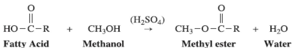
Fig 4.7- Esterification of FFAs [Van Gerpen, 2005]
