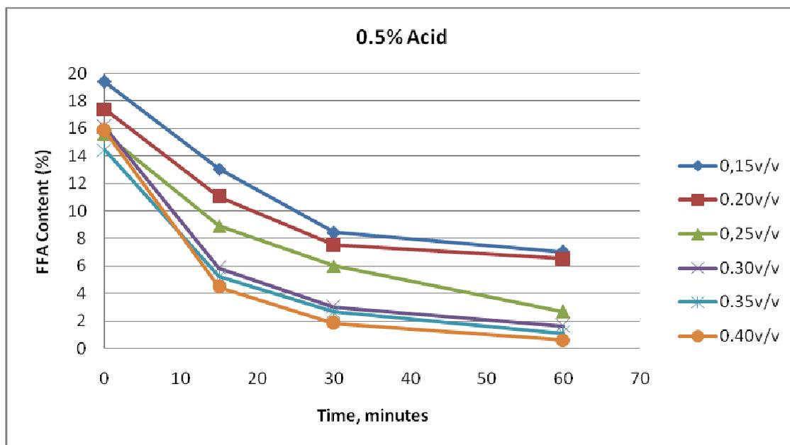
Fig 6. 4 - Effect of reaction time and methanol quantity on reduction of FFA value of palm oil for 0.5% v/v, acid-to-oil ratios during pretreatment for biodiesel production(initial FFA value = 19.80%)
