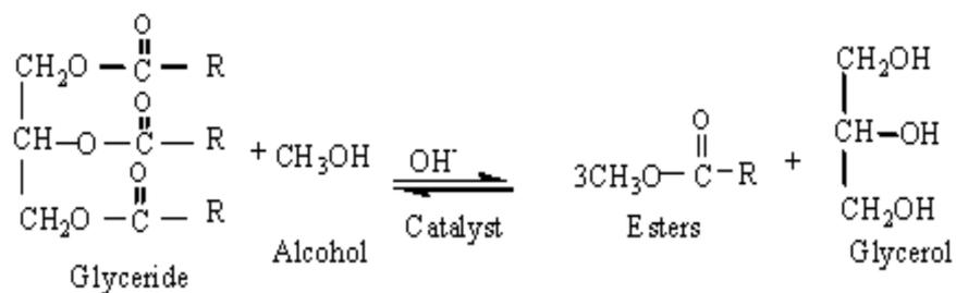
Fig 4.2 - Esterification process (Shay, 1993)
