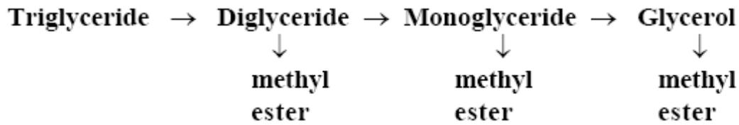
Fig 4.5 - Sequence of events of the transesterification reaction (Van Gerpen, 2005)
