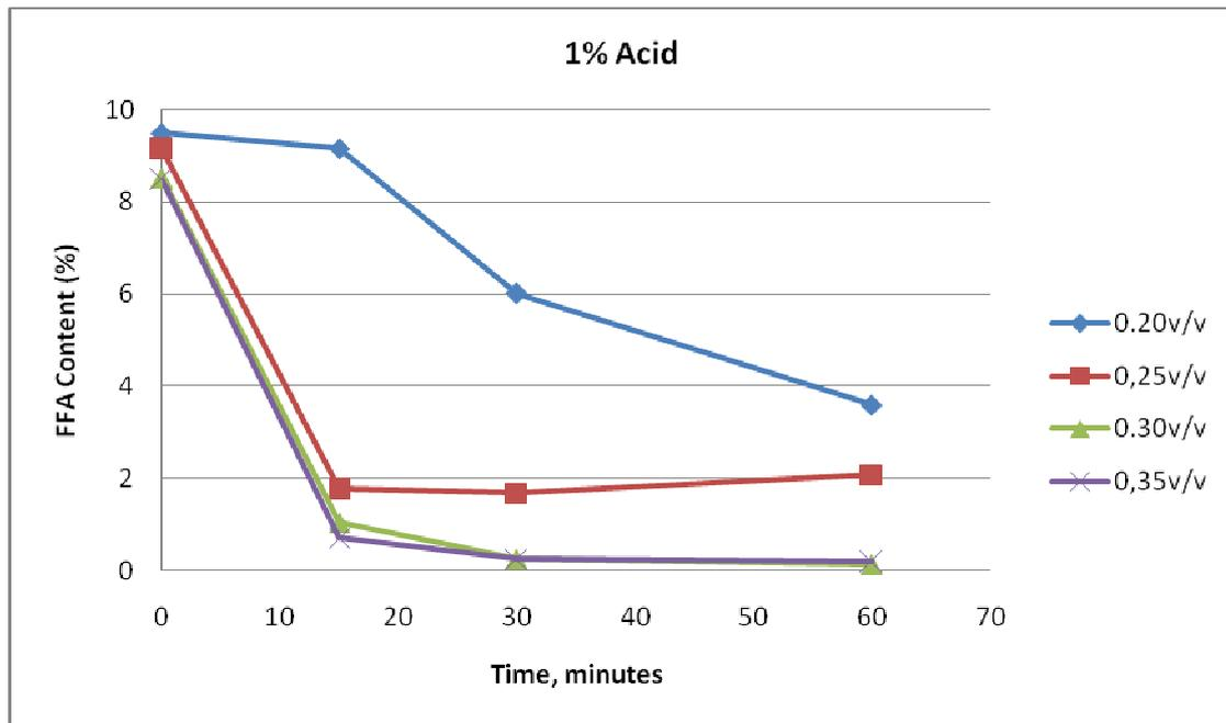
Fig 6. 3- Effect of reaction time and methanol quantity on reduction of FFA value of palm oil for 1.0 % v/v, acid-to-oil ratios during pretreatment for biodiesel production (initial FFA value = 8.28%)
