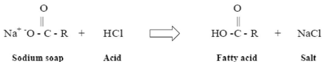
Fig 4.4- Reaction of soaps with the acid
