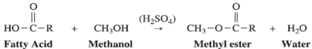
Fig 1 - Esterification of FFAs (Van Gerpen, 2005)
