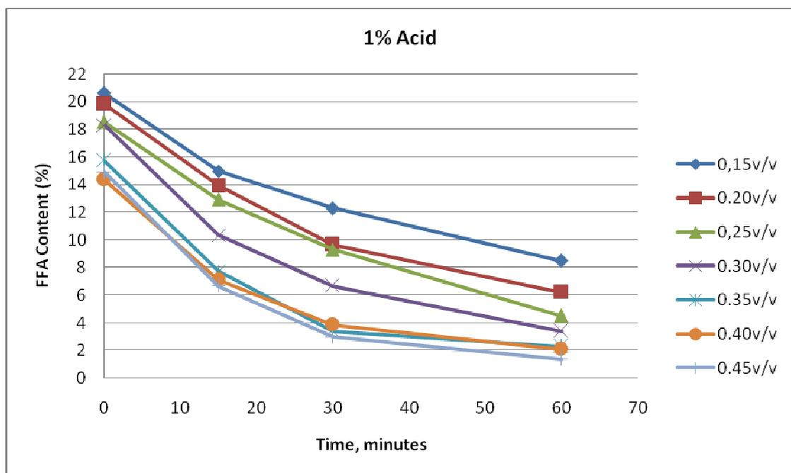
Fig 6.7 - Effect of reaction time and methanol quantity on reduction of FFA value of palm oil for 1.0 % v/v, acid-to-oil ratios during pretreatment for biodiesel production (initial FFA value = 22.11%)
