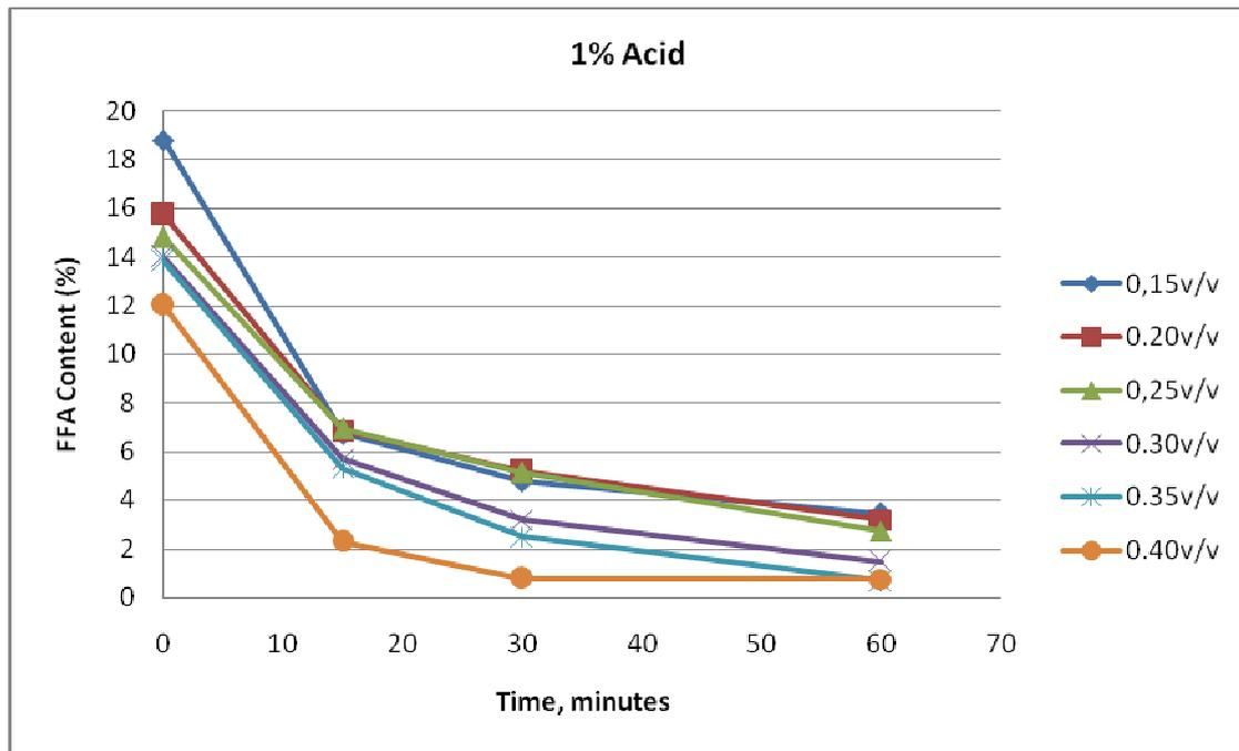
Fig 6. 5 - Effect of reaction time and methanol quantity on reduction of FFA value of palm oil for 1.0 % v/v, acid-to-oil ratios during pretreatment for biodiesel production(initial FFA value = 19.80%)
