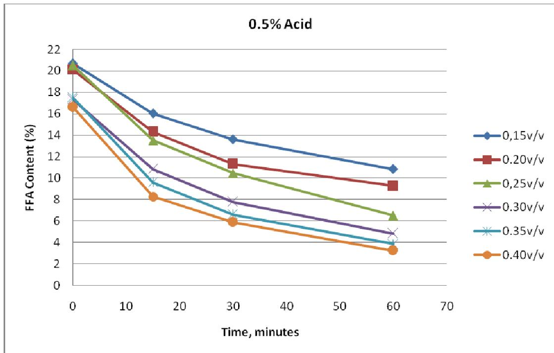
Fig 6.6 - Effect of reaction time and methanol quantity on reduction of FFA value of palm oil for 0.5% v/v, acid-to-oil ratios during pretreatment for biodiesel production (initial FFA value = 22.11%)
