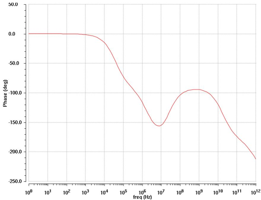
Fig. 5.36: Phase vs. frequency (0.5V OTA)
