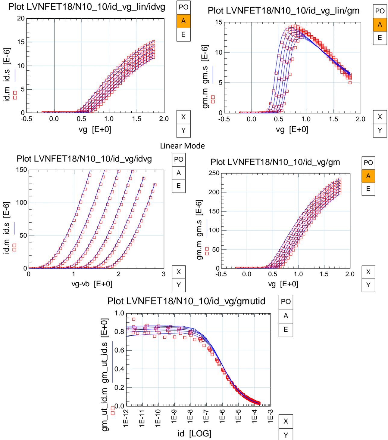
Fig. 1.48: Output Characteristics  $I_{D,S}-V_{GS}$ ,  $g_m-V_{GS}$ ,  $g_m/I_{D,S}$  (NMOS W/L=10um/10um)
