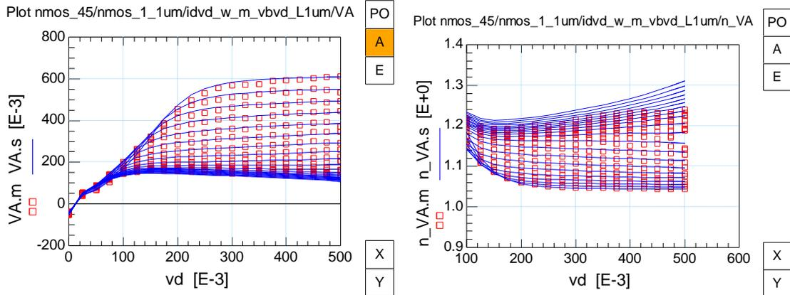
Fig. 1.38:  $V_A$ , and  $n$  vs.  $V_{DS}$  characteristics for the Drain-Bulk connected NMOS device ( $W/L=1\mu\text{m}/1\mu\text{m}$ )
