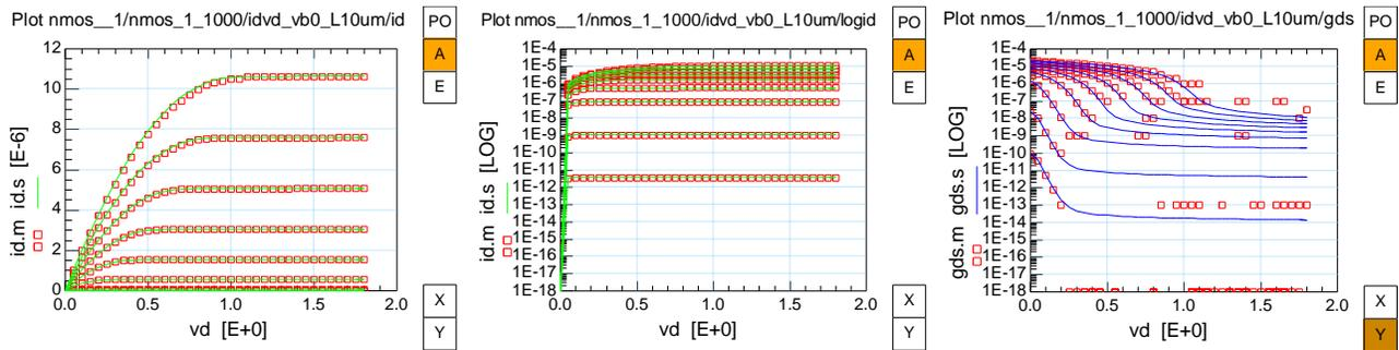
Fig. 1.20: NMOS Source-Bulk output characteristics  $I_{DS}$ ,  $g_{DS}$  vs.  $V_{DS}$  ( $W/L=1\mu m/10\mu m$ )
