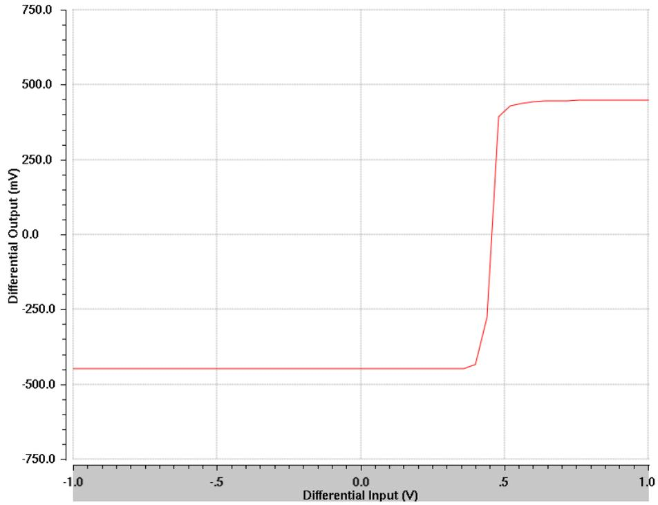
Fig. 5.34: DC input-output characteristics of 0.5V gate-input OTA
