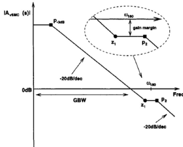
Fig. 3.9: Frequency response of a SMC amplifier
