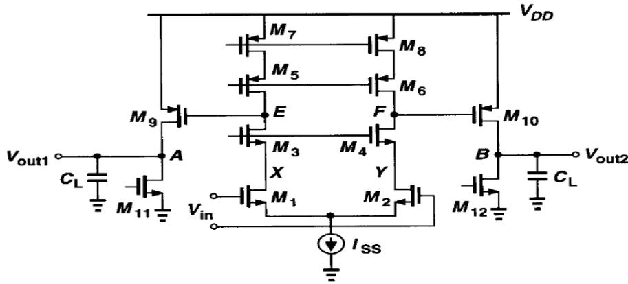
Fig. 3.11: Two-stage op-amp.
