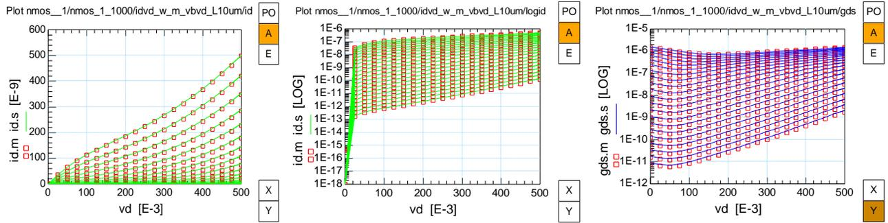
Fig. 1.21: NMOS Drain-Bulk output characteristics  $I_{DS}$ ,  $g_{DS}$  vs.  $V_{DS}$  ( $W/L=1\mu\text{m}/10\mu\text{m}$ )
