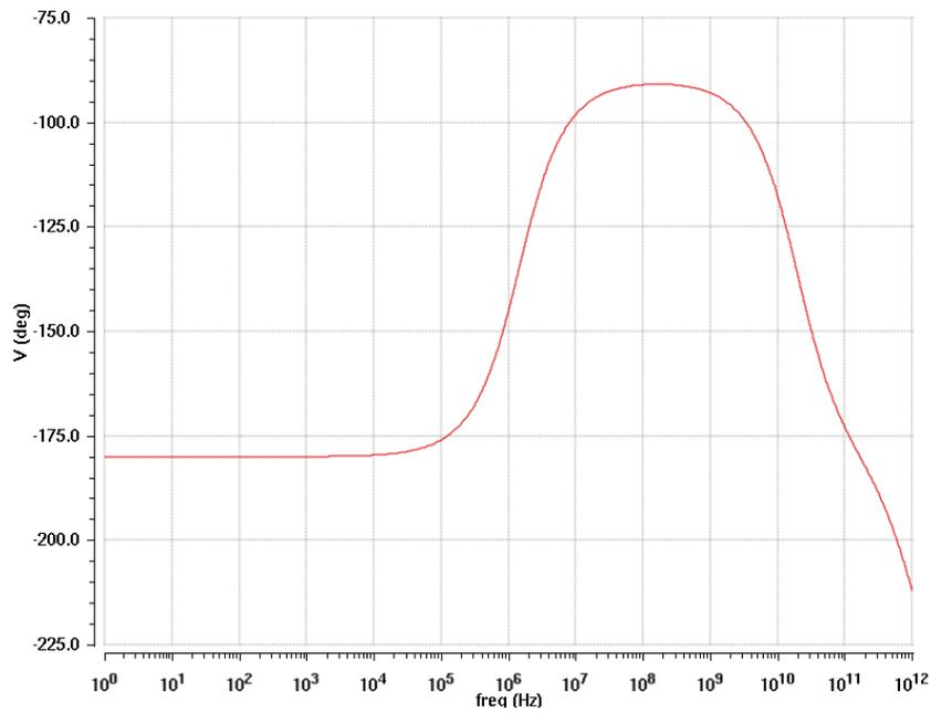
Fig. 5.22: Phase vs. Frequency (one stage OTA)
