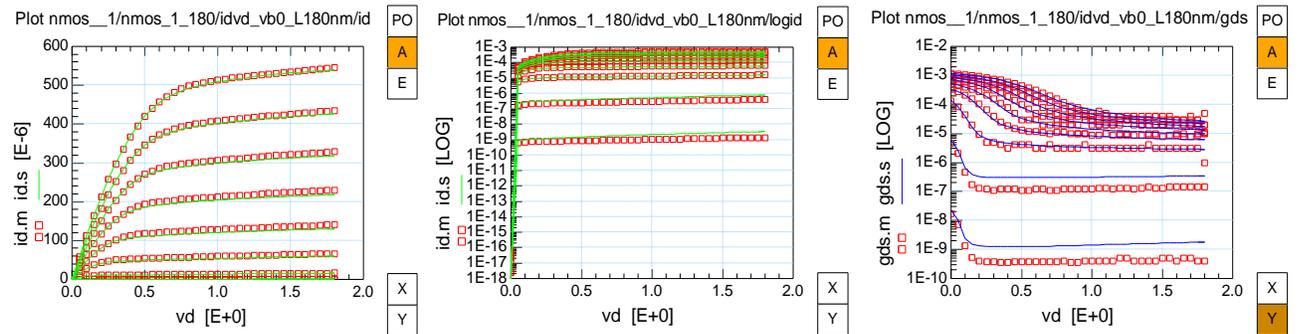
Fig. 1.24: NMOS Source-Bulk output characteristics  $I_{DS}$ ,  $g_{DS}$  vs.  $V_{DS}$  ( $W/L=1\mu m/180nm$ )
