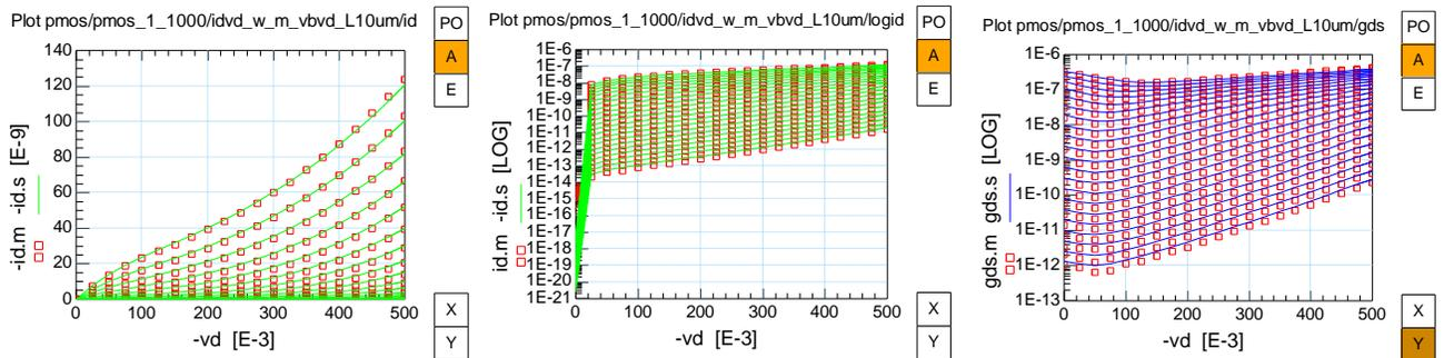
Fig. 1.29: PMOS Drain-Bulk output characteristics  $I_{DS}$ ,  $g_{DS}$  vs.  $V_{DS}$  ( $W/L=1\mu m/10\mu m$ )
