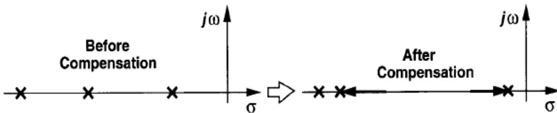
Fig. 3.14: Pole splitting as a result of Miller compensation.
