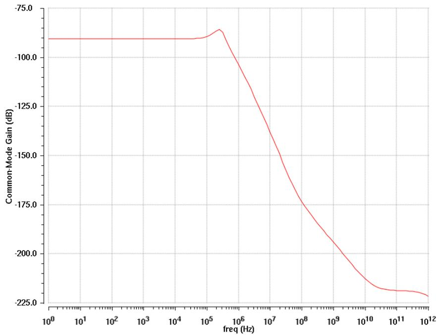
Fig. 5.38: Common-Mode gain response (0.5V OTA)
