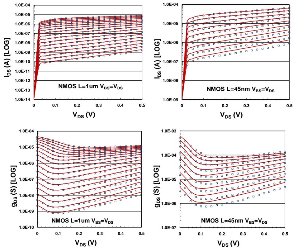
Fig. 1.46: Drain-bulk connected NMOS transistor, with respective output characteristics,  $W/L=1\mu\text{m}/1\mu\text{m}$  (left) and  $W/L=1\mu\text{m}/45\text{nm}$ .  $I_{DS}$ ,  $g_{DS}$  vs.  $V_{DS}$  are shown for various values of  $V_{GS}$  (markers: TCAD simulation data, lines: EKV3 model).
