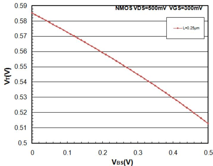
Fig. 2.7: Simulated device  $V_T$  as a function of  $V_{BS}$
