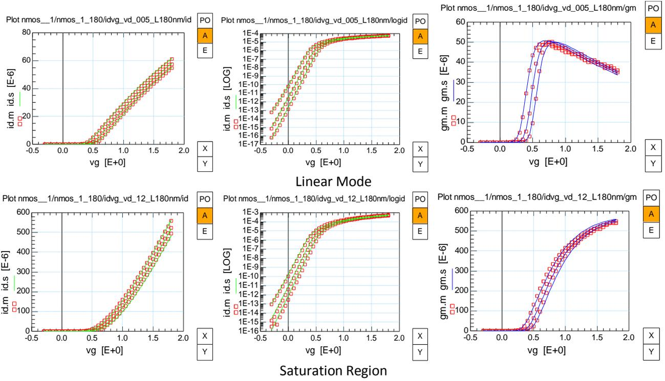
Fig. 1.23: NMOS Source-Bulk output characteristics  $I_{DS}$ ,  $g_m$  vs.  $V_{GS}$  ( $W/L=1\mu m/180nm$ ), linear region (up) and saturation region (down)
