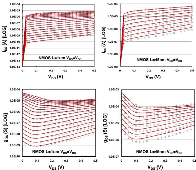
Figure 5: Drain-bulk connected NMOS transistor, with respective output characteristics,  $W/L=1\mu\text{m}/1\mu\text{m}$  (left) and  $W/L=1\mu\text{m}/45\text{nm}$ .  $I_{DS}$ ,  $g_{DS}$  vs.  $V_{DS}$  are shown for various values of  $V_{GS}$  (markers: TCAD simulation data, lines: EKV3 model).
