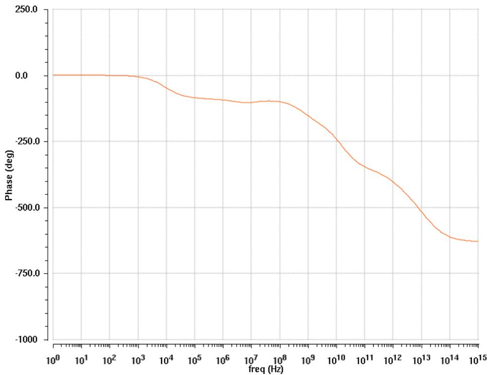
Fig. 5.29: Phase vs. frequency (two-stage OTA)
