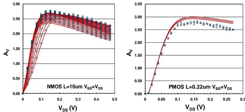
Fig. 1.45: Intrinsic Gain  $A_V$  of drain-bulk connected NMOS (left) and PMOS (right) devices (markers: TCAD/measured data, lines: EKV3/analytical model).
