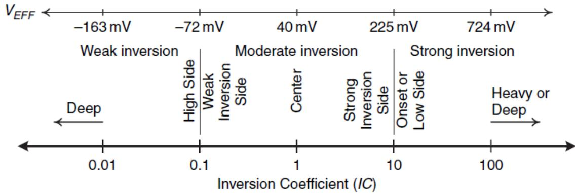
Fig. 4.2: The inversion coefficient presented as a number line showing the regions and sub-regions of MOS inversion with corresponding effective gate–source voltage,  $V_{EFF} = V_{GS} - V_T$ . The effective gate–source voltage is for room temperature ( $T = 300\text{K}$ ) and an average substrate factor of  $n = 1.4$ . It is higher than values shown for short-channel devices operating in strong inversion due to velocity saturation.
