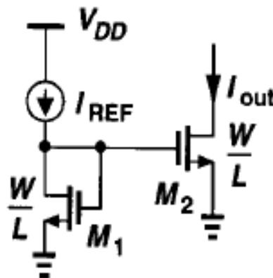
Fig. 3.1: Simple current mirror
