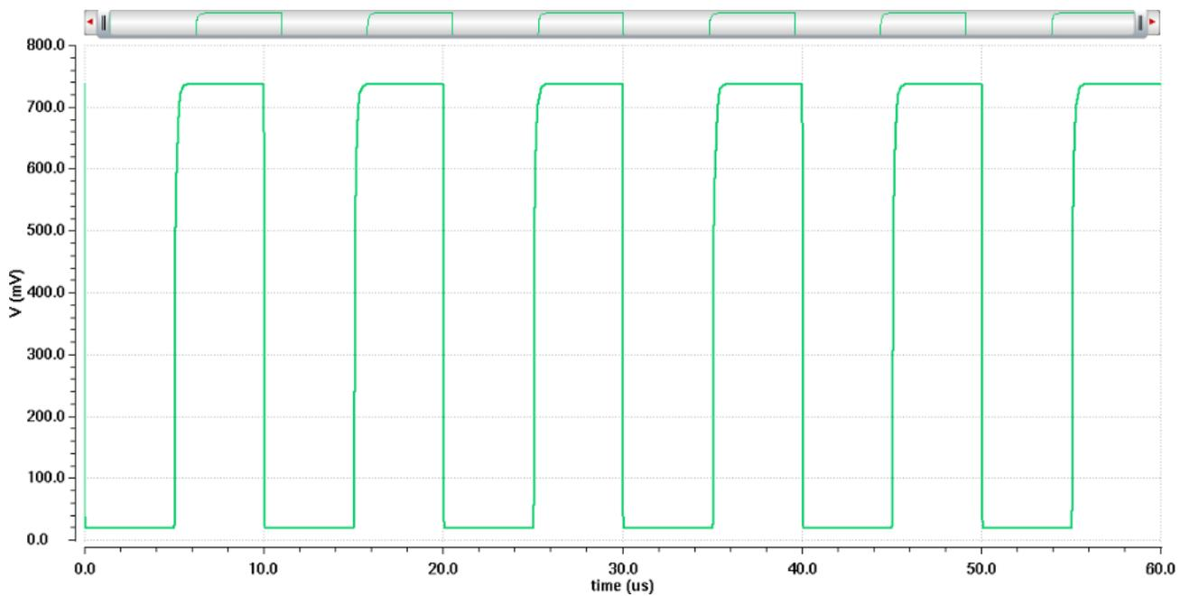
Fig. 5.18: Output signal for simulating Slew Rate
