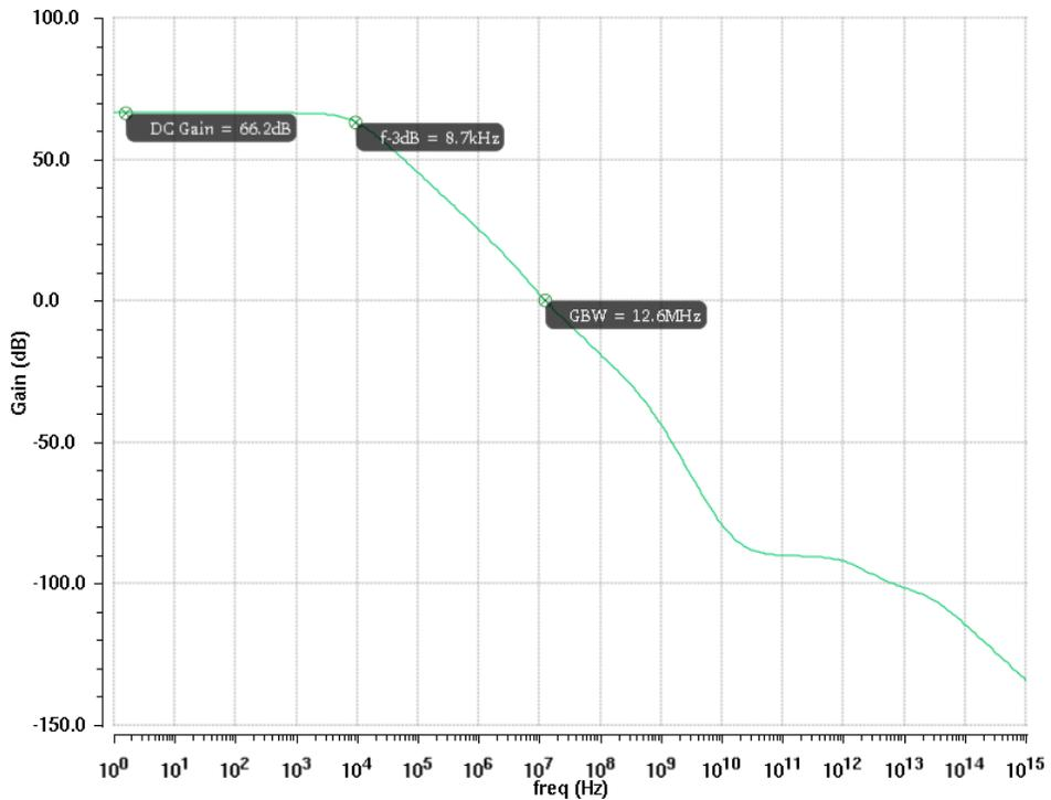
Fig. 5.27: Gain vs. frequency (two stage OTA)
