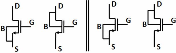
Figure 1: NMOS (left) and PMOS (right) transistors, with their local substrate (or well) connected to either source or drain.
