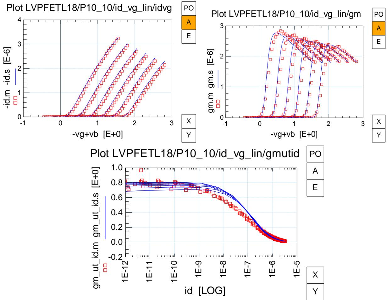
Fig. 1.56: Output Characteristics  $I_{DS}$ - $V_{GS}$   $g_m$ - $V_{GS}$ ,  $g_m/I_{DS}$  Linear Mode(PMOS W/L=10um/10um)
