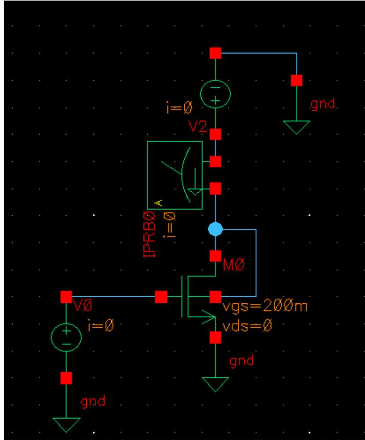
Fig. 5.4: Drain-Bulk NMOS simulation setup
