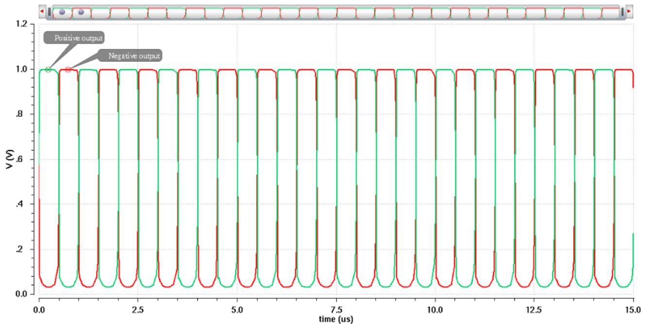
Fig. 5.15: Output signals in time domain
