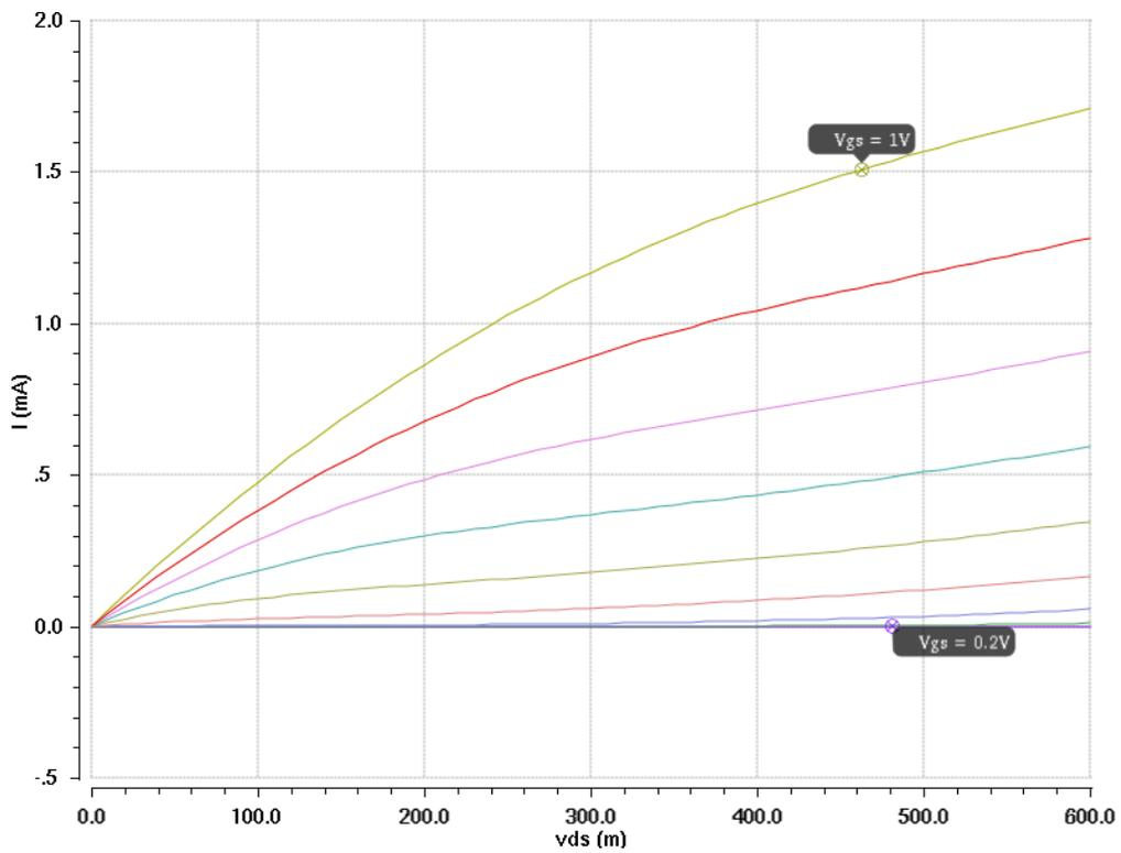
Fig. 5.6:  $I_{DS}$ - $V_{DS}$ , Drain-Bulk connected NMOS ( $W/L=10\mu\text{m}/280\text{nm}$ )
