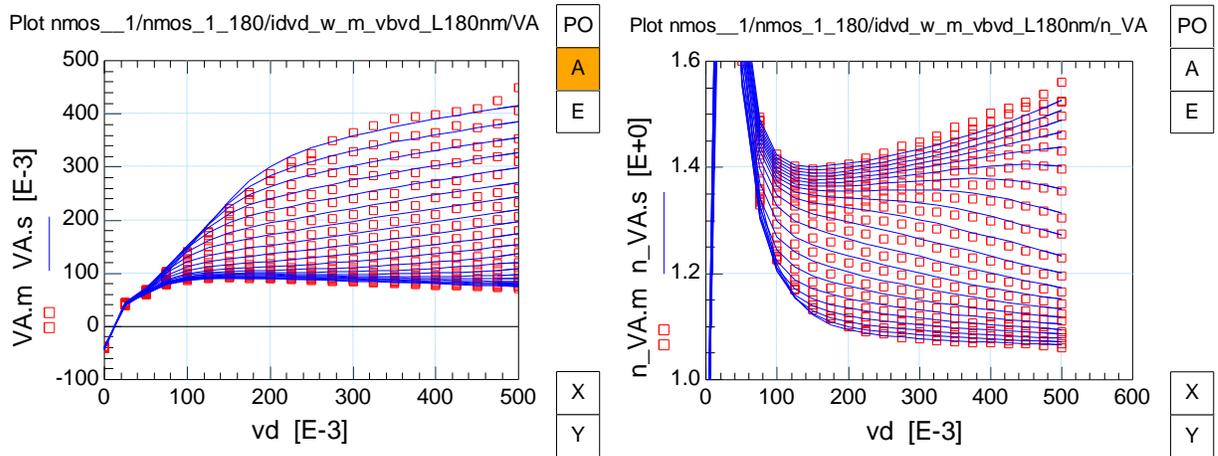
Fig. 1.26:  $V_A$ , and  $n$  vs.  $V_{DS}$  characteristics for the Drain-Bulk connected NMOS device ( $W/L=1\mu\text{m}/180\text{nm}$ )
