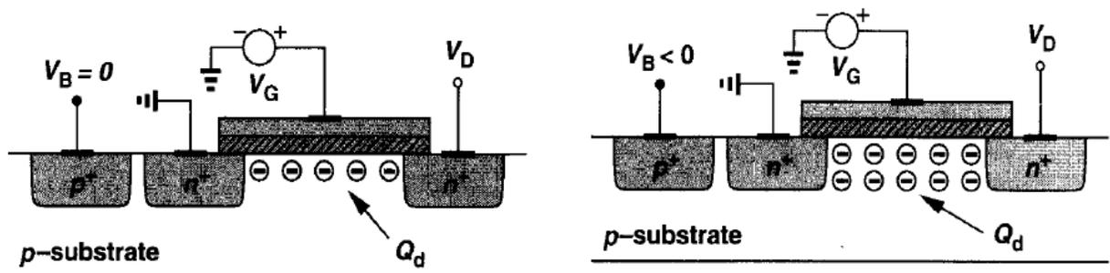
Fig. 2.5: Variation of depletion region charge with bulk voltage
