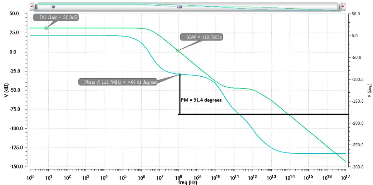
Fig. 5.13: AC response of gate-input operational transconductance amplifier
