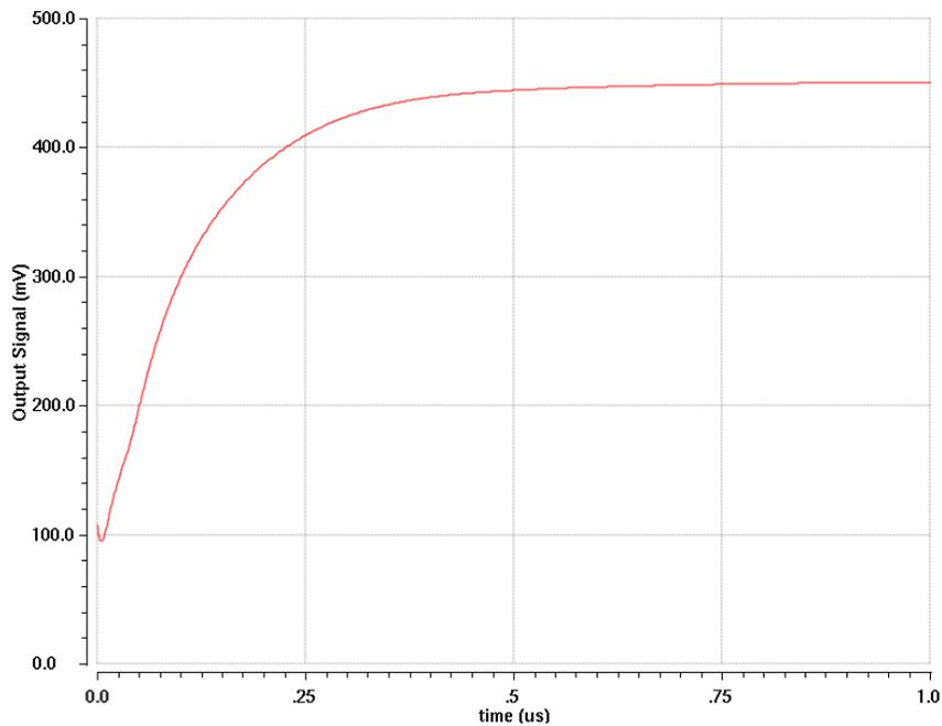
Fig. 5.41: Output Signal for Slew Rate simulation (0.5V OTA)
