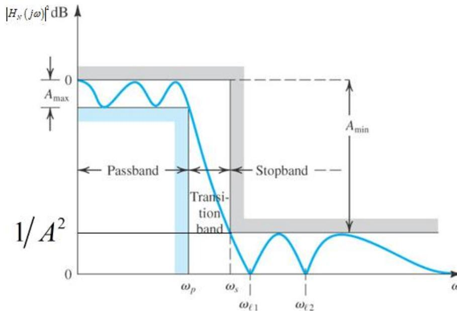
Fig. 6.1: Frequency response of a low-pass filter
