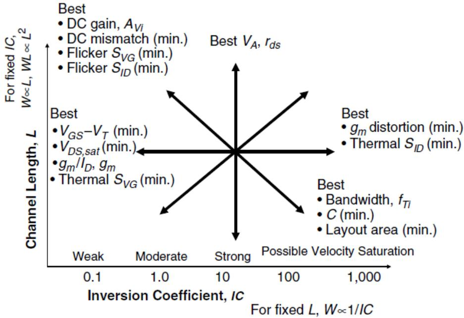
Fig. 4.1: *MOSFET Operating Plane* illustrating MOS analog performance tradeoffs versus selected inversion coefficient and channel length for a fixed drain current. Each MOSFET in an analog circuit operates at some inversion coefficient and channel length defining a point on the operating plane
