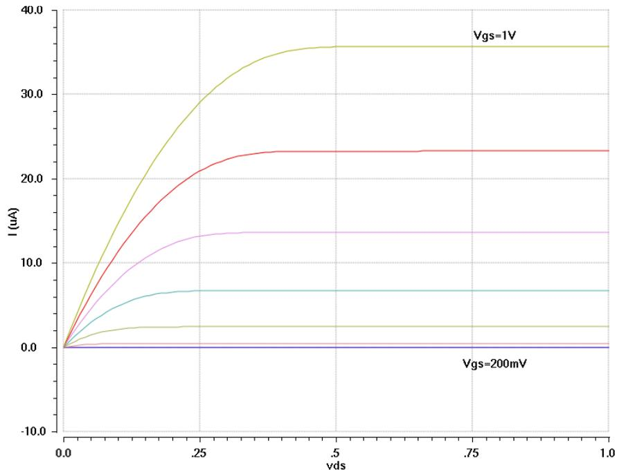
Fig. 5.2:  $I_{DS}-V_{DS}$ , Conventional NMOS ( $W/L=10\mu\text{m}/10\mu\text{m}$ )
