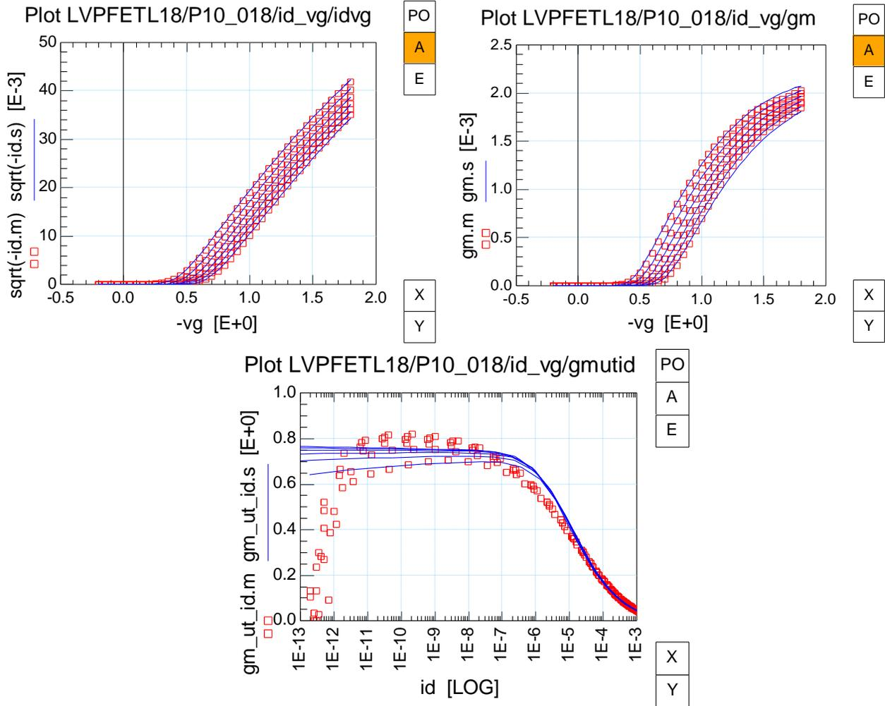
Fig. 1.62: Output Characteristics  $I_{DS}$ - $V_{GS}$ ,  $g_m$ - $V_{GS}$ ,  $g_m/I_{DS}$ , Saturation Region (PMOS W/L=10um/0.18um)
