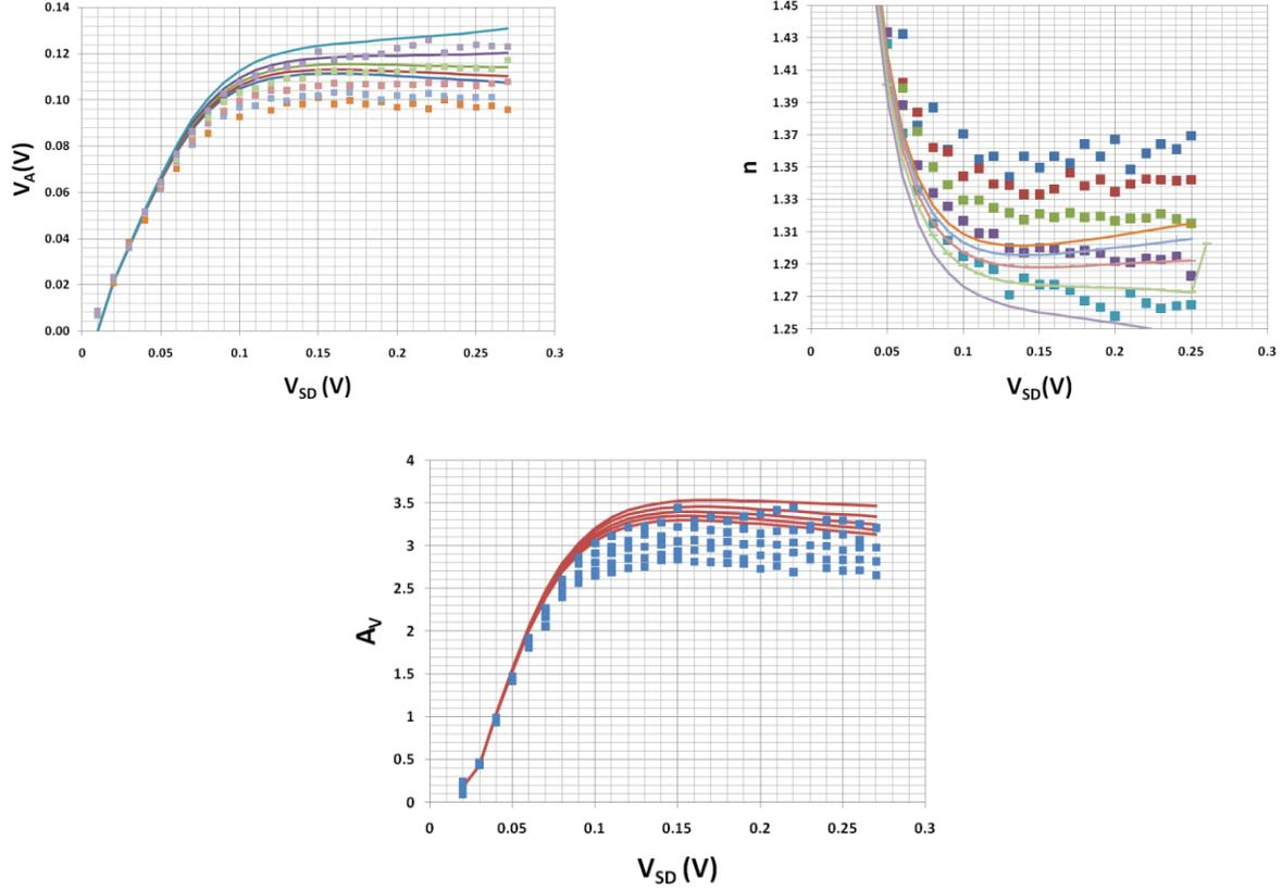
Fig. 1.13: Early Voltage  $V_A$ , Slope Factor  $n$  extracted from Equation (1.19) and Intrinsic Gain  $A_v$  of drain-bulk connected PMOS devices (markers: measured data, lines: analytical model).
