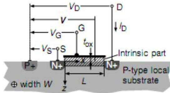
Fig. 1.7: Cross section of a MOS transistor
