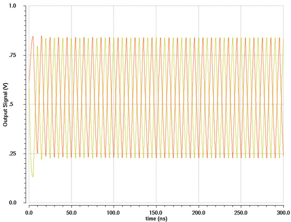
Fig. 5.32: Output Signals in time domain of two-stage OTA
