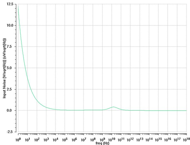
Fig. : Input – referred white noise spectral density
