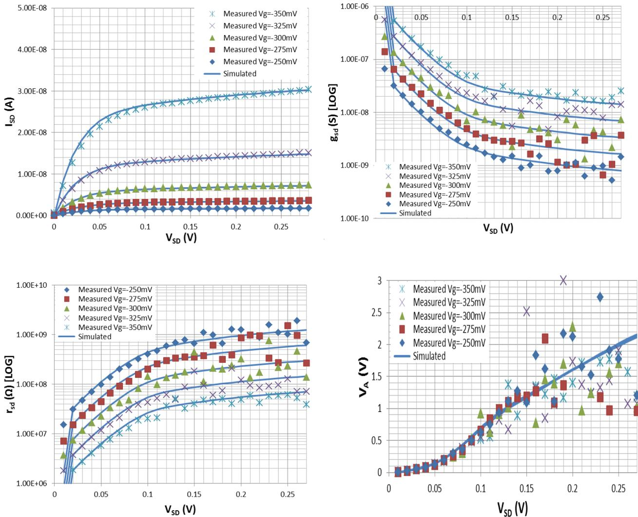
Fig. 1.15: Source-Bulk Connected PMOS W/L=10um/0.18um
