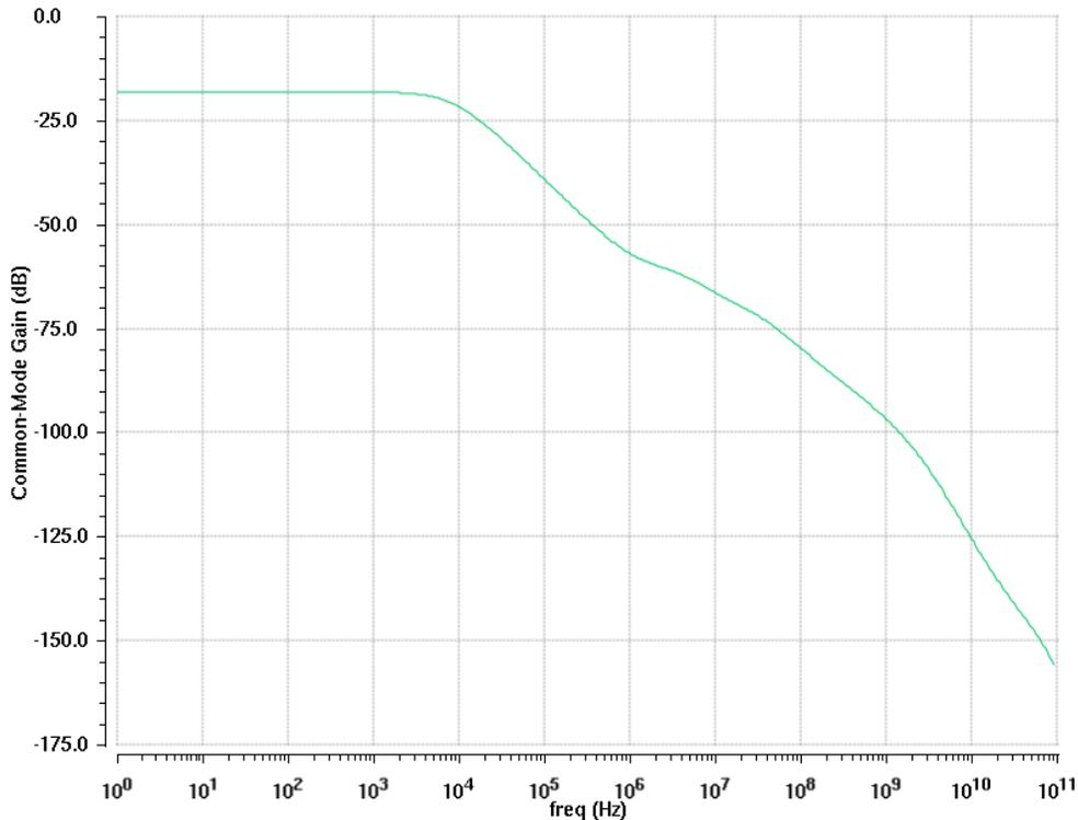
Fig. 5.30: Common-Mode gain response of two stage OTA
