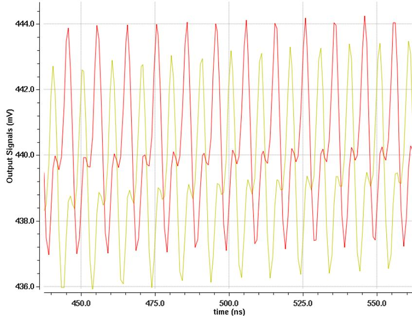
Fig. 5.40: Output signals in time domain (0.5V OTA)
