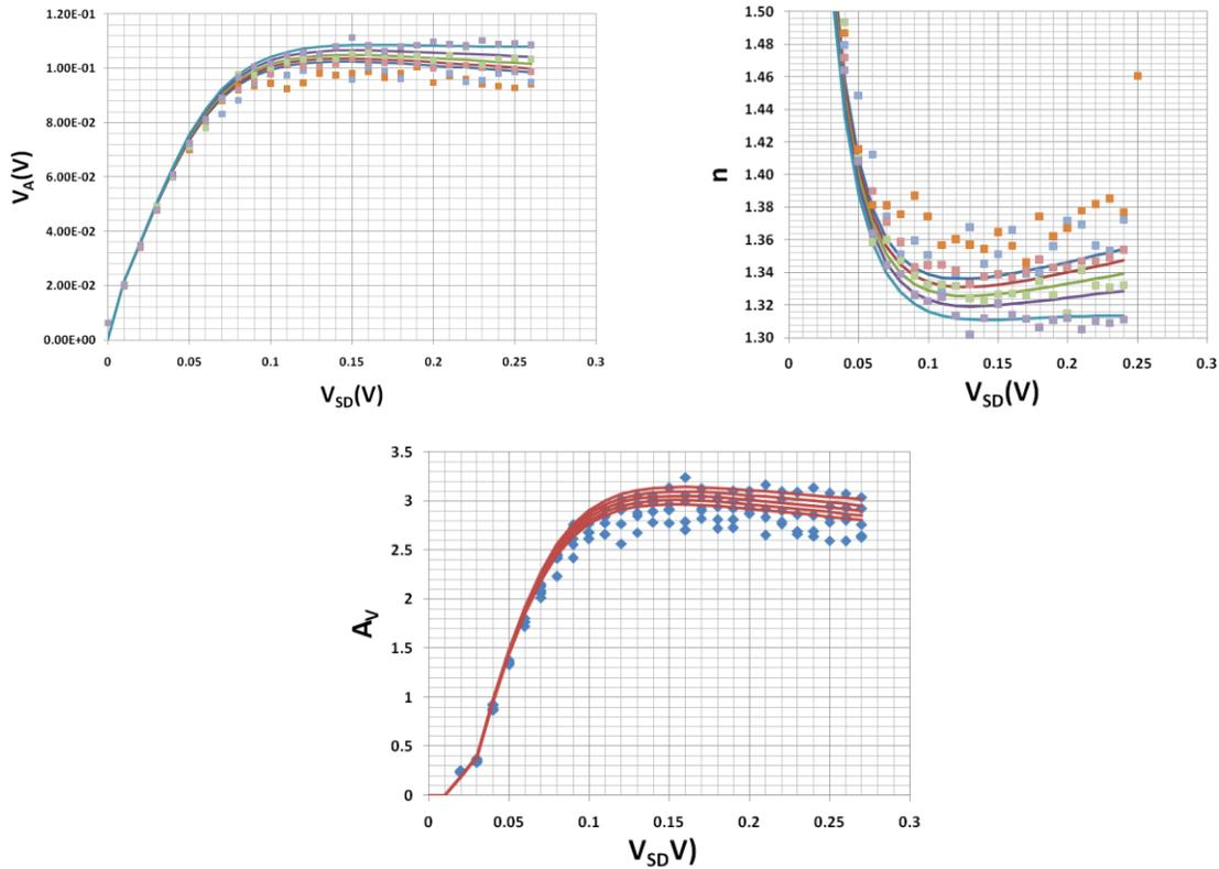
Fig. 1.11: Early Voltage  $V_A$ , Slope Factor  $n$  extracted from Equation (1.19) and Intrinsic Gain  $A_V$  of drain-bulk connected PMOS devices (markers: measured data, lines: analytical model).
