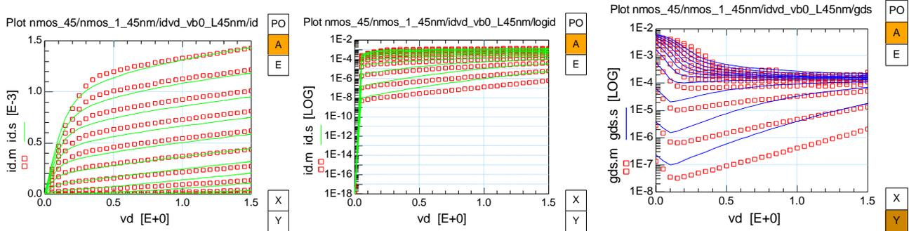
Fig. 1.40: NMOS Source-Bulk output characteristics  $I_{DS}$ ,  $g_{DS}$  vs.  $V_{DS}$  ( $W/L=1\mu\text{m}/45\text{nm}$ )
