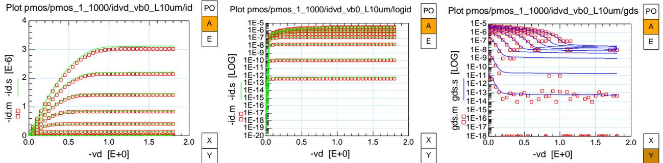
Fig. 1.28: PMOS Source-Bulk output characteristics  $I_{DS}$ ,  $g_{DS}$  vs.  $V_{DS}$  ( $W/L=1\mu m/10\mu m$ )
