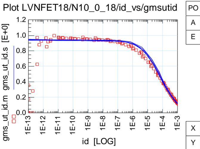
Fig. 1.54: Output Characteristics  $I_{DS}-V_S$ ,  $g_{ms}-V_S$ ,  $g_{ms}/I_{DS}$  (NMOS W/L=10um/0.18um)
