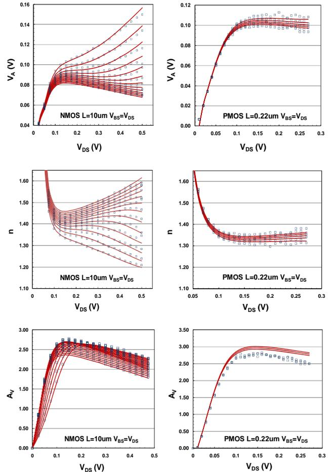
Fig. 3: Early Voltage  $V_A$ , Slope Factor  $n$  extracted from Equation (13) and Intrinsic Gain  $A_V$  of drain-bulk connected NMOS (left) and PMOS (right) devices (markers: TCAD/measured data, lines: EKV3/analytical model).
