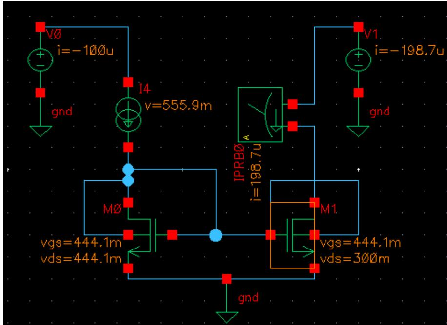
Fig. 5.7: Grounded-Gate NMOS current mirror
