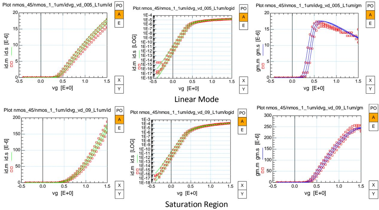
Fig. 1.35: NMOS Source-Bulk output characteristics  $I_{DS}$ ,  $g_m$  vs.  $V_{GS}$  ( $W/L=1\mu m/1\mu m$ )
