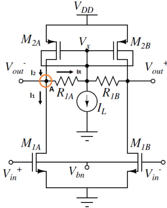
Fig. 5.9: Basic configuration of gate-input OTA
