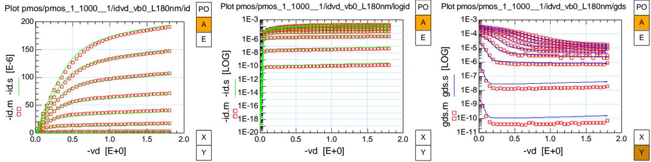
Fig. 1.32: PMOS Source-Bulk output characteristics  $I_{DS}$ ,  $g_{DS}$  vs.  $V_{DS}$  ( $W/L=1\mu\text{m}/180\text{nm}$ )
