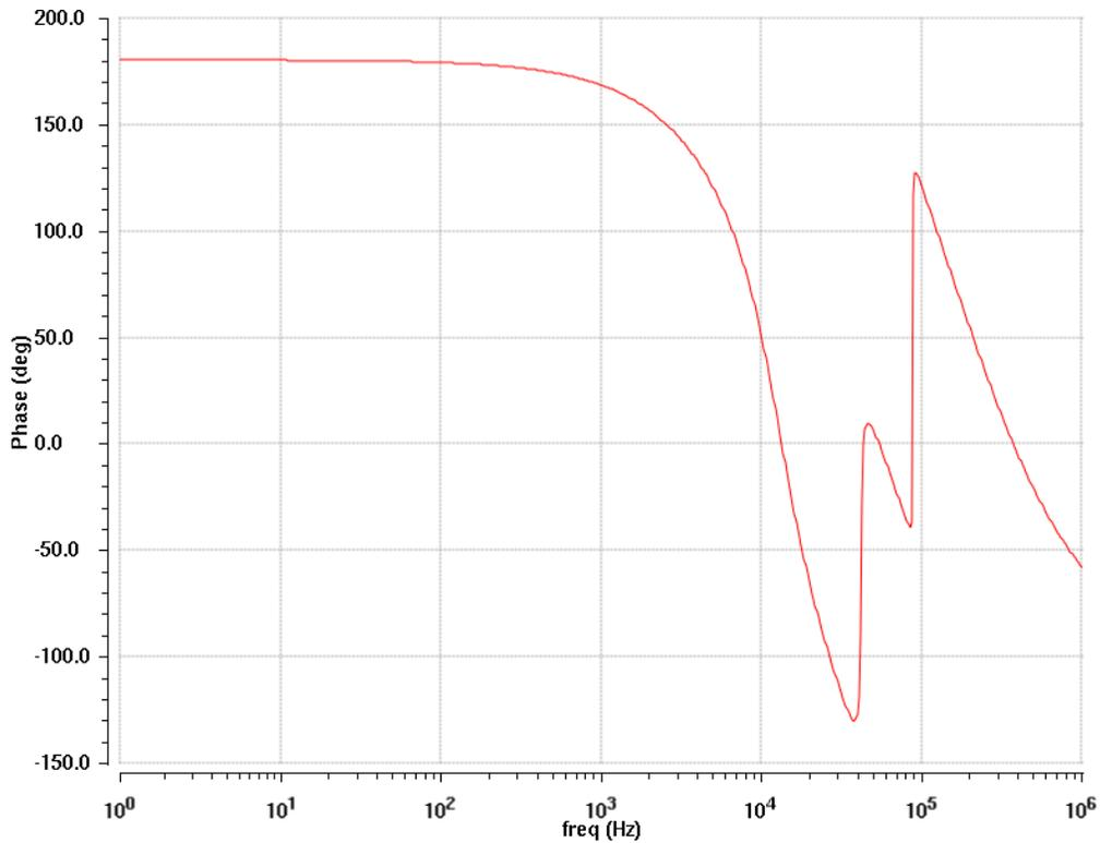
Fig. 6.4: Simulated filter characteristics, Phase vs. frequency ( $V_{DD}=1V$ )
