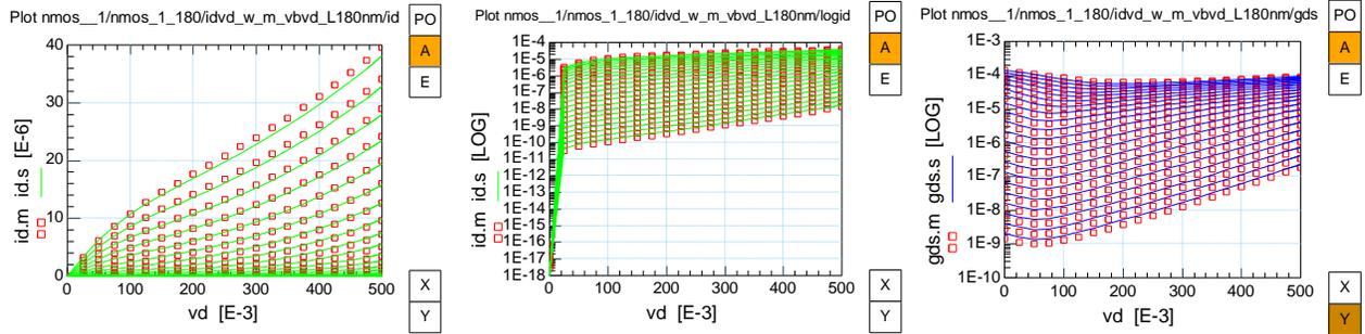
Fig. 1.25: NMOS Drain-Bulk output characteristics  $I_{DS}$ ,  $g_{DS}$  vs.  $V_{DS}$  ( $W/L=1\mu\text{m}/180\text{nm}$ )
