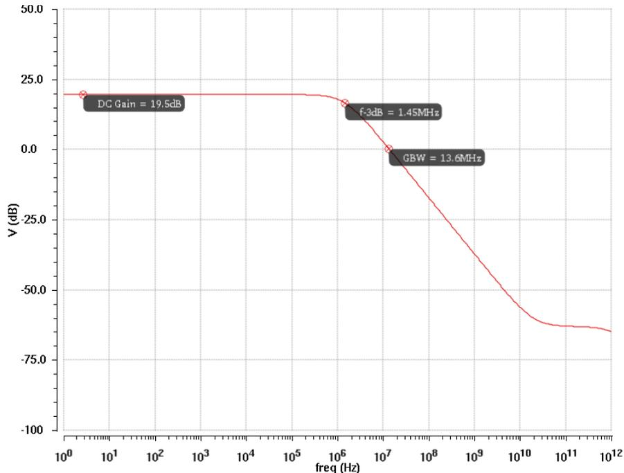
Fig. 5.21: Gain vs. Frequency (one stage OTA)
