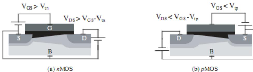
Fig. 1.6: Channel pinch-off for (a) NMOS and (b) PMOS transistor devices.
