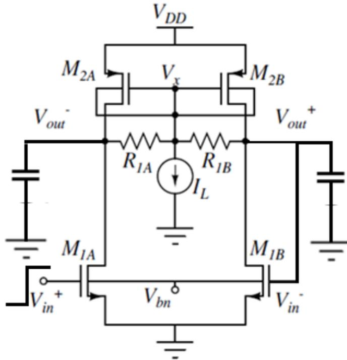
Fig. 5.16: Slew Rate simulation setup
