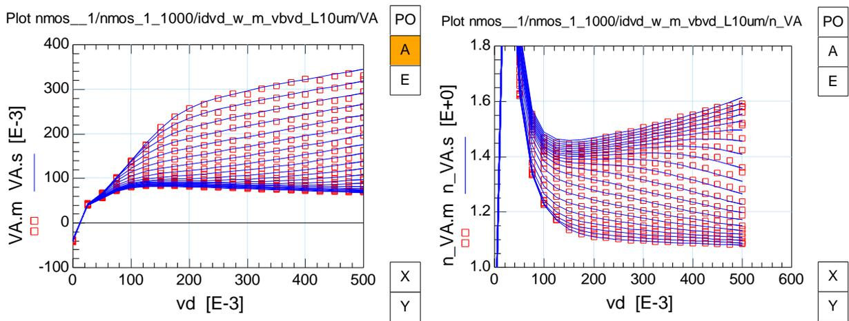
Fig. 1.22:  $V_A$ , and  $n$  vs.  $V_{DS}$  characteristics for the Drain-Bulk connected NMOS device ( $W/L=1\mu\text{m}/10\mu\text{m}$ )
