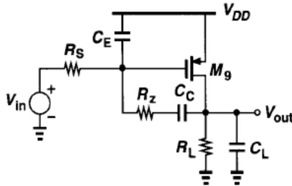
Fig. 3.15: Simplified circuit of two-stage opamp, with the addition of  $R_z$
