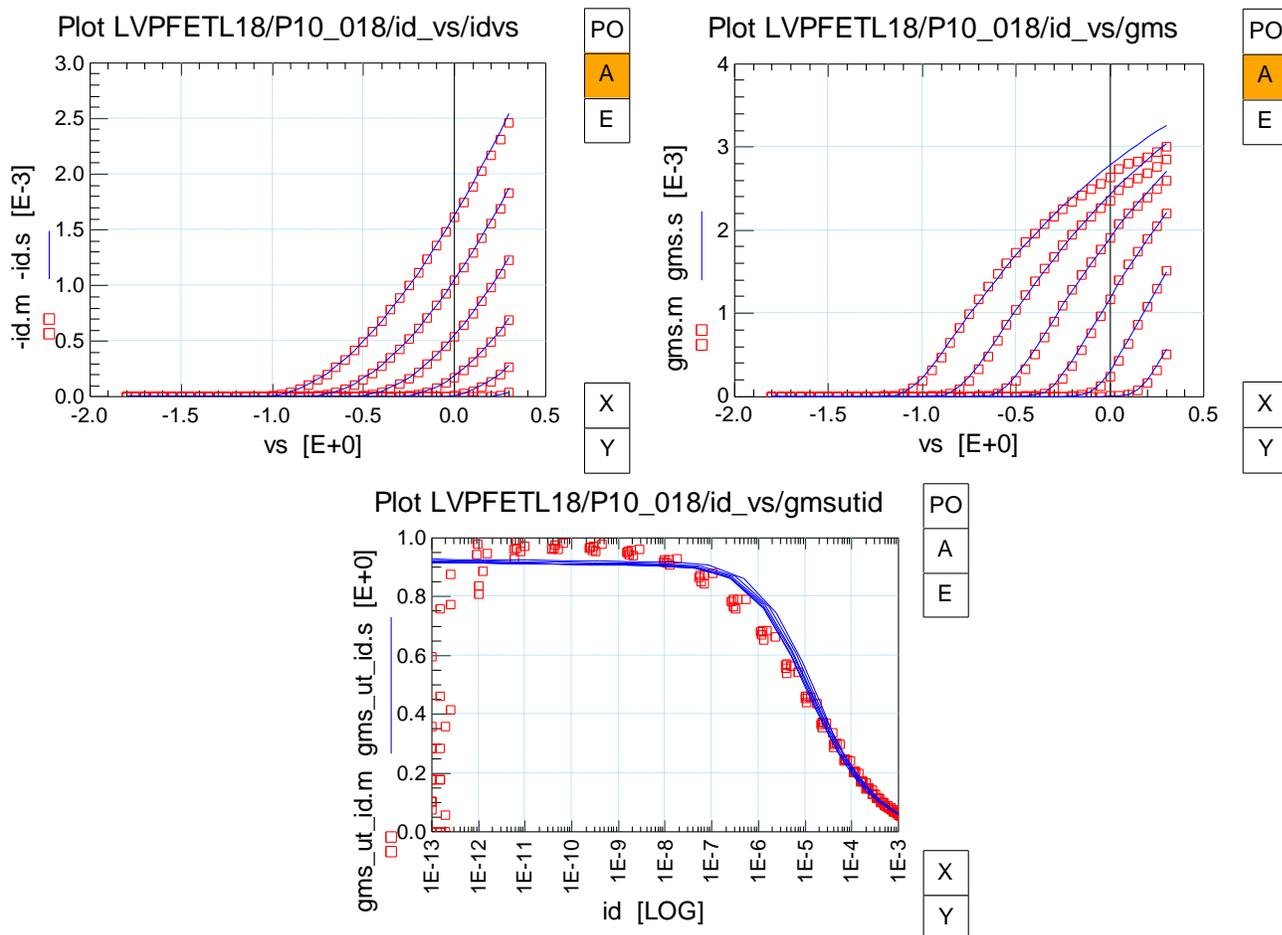
Fig. 1.63: Output Characteristics  $I_{DS}-V_S$ ,  $g_{ms}-V_{DS}$ ,  $g_{ms}/I_{DS}$  (PMOS  $W/L=10\mu\text{m}/0.18\mu\text{m}$ )
