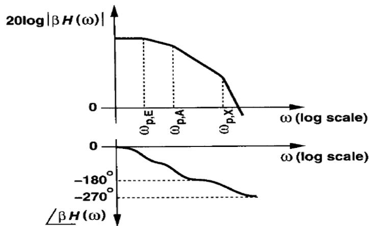
Fig. 3.12: Bode plots of loop gain of two-stage op amp.
