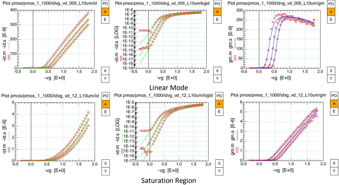
Fig. 1.27: PMOS Source-Bulk output characteristics  $I_{DS}$ ,  $g_m$  vs.  $V_{GS}$  ( $W/L=1\mu m/10\mu m$ ), linear region (up) and saturation region (down)
