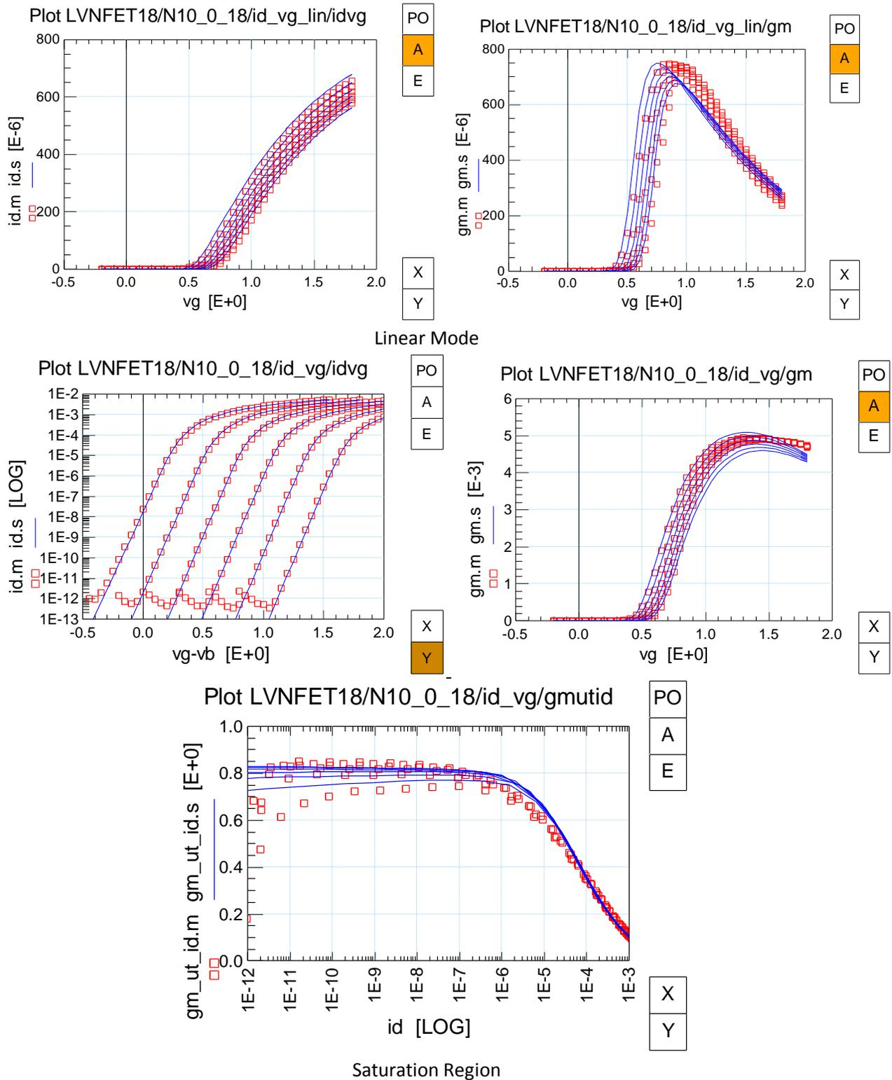
Fig. 1.52: Output Characteristics  $I_{DS}$ - $V_{GS}$ ,  $g_m$ - $V_{GS}$ ,  $g_m/I_{DS}$  (NMOS W/L=10um/0.18um)
