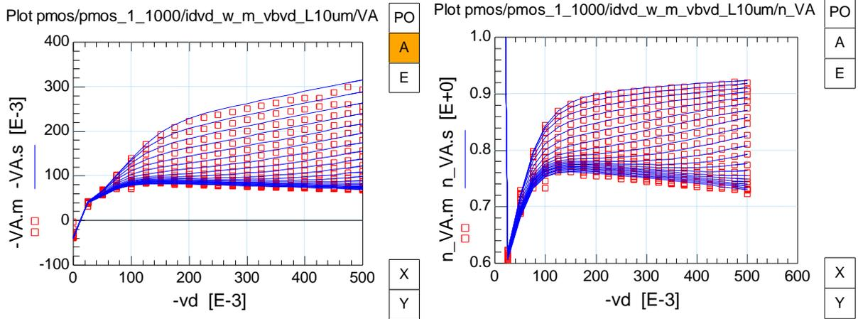
Fig. 1.30:  $V_A$ , and  $n$  vs.  $V_{DS}$  characteristics for the Drain-Bulk connected PMOS device ( $W/L=1\mu\text{m}/10\mu\text{m}$ )
