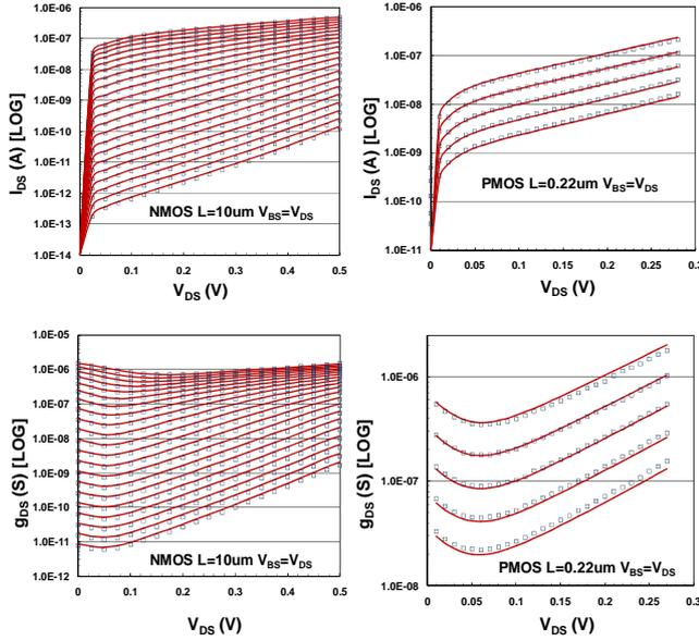
Fig. 2: Drain-bulk connected NMOS (left) and PMOS (right) transistor, with respective output characteristics,  $W/L=1\mu\text{m}/10\mu\text{m}$  (left) and  $W/L=10\mu\text{m}/0.22\mu\text{m}$ .  $I_{DS}$ ,  $g_{DS}$  vs.  $V_{DS}$  are shown for various values of  $V_{GS}$  (markers: TCAD simulation data(left), measurements (right), lines: EKV3 model (left), analytical charge-based model (right)).
