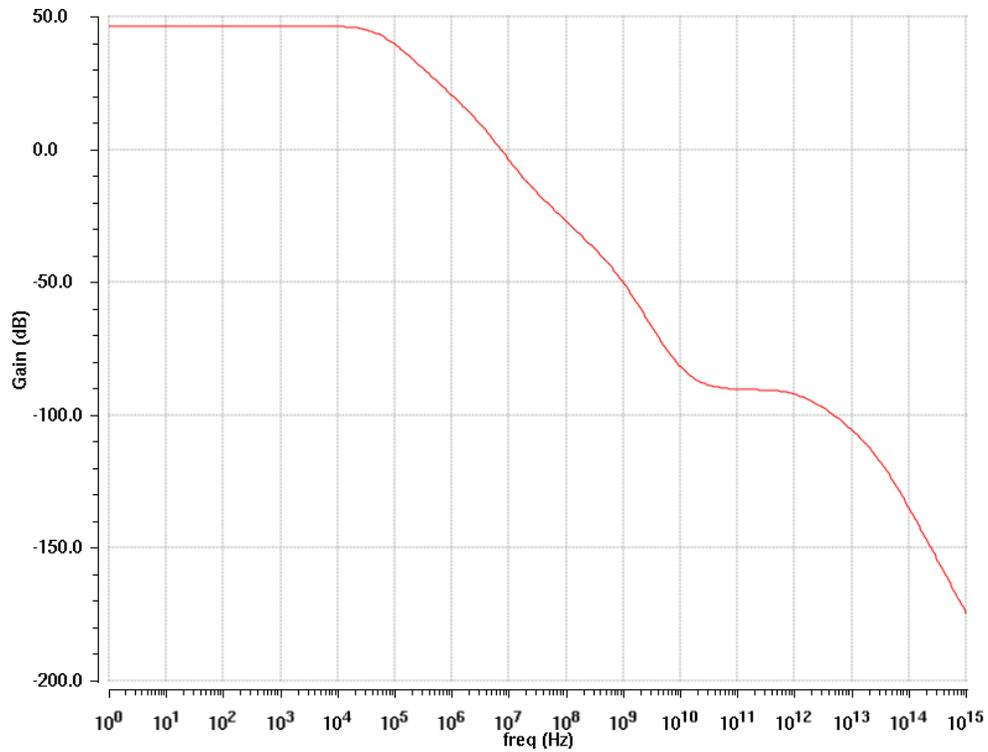
Fig. 5.28: Frequency Response with the gain enhancement disabled
