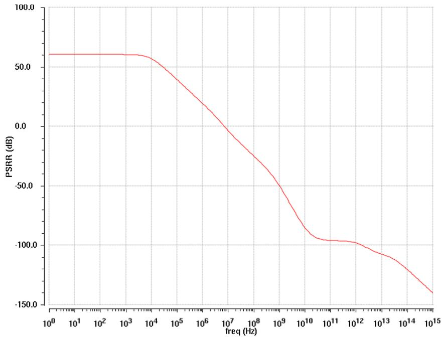
Fig. 5.31: PSRR response of two stage OTA
