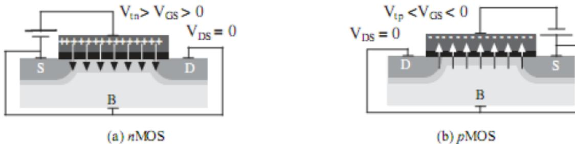
Fig. 1.4: (a) Depleting the NMOS channel of holes with small positive values of gate–source voltage, and (b) depleting the PMOS channel of electrons with small negative values of gate–source voltage
