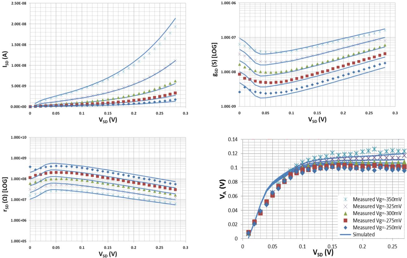
Fig. 1.18: Drain-Bulk Connected PMOS W/L=10um/10um
