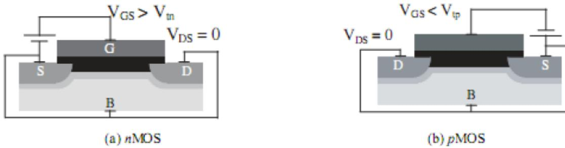
Fig. 1.5: Creating conducting channel for (a) NMOS and (b) PMOS transistors.
