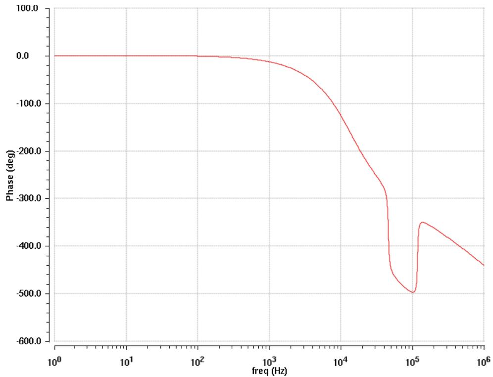
Fig. 6.6: Phase vs. frequency of the 0.5V low-pass elliptic filter
