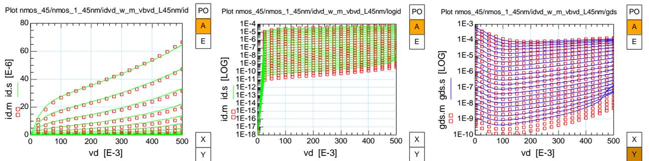
Fig. 1.41: NMOS Drain-Bulk output characteristics  $I_{DS}$ ,  $g_{DS}$  vs.  $V_{DS}$  ( $W/L=1\mu\text{m}/45\text{nm}$ )
