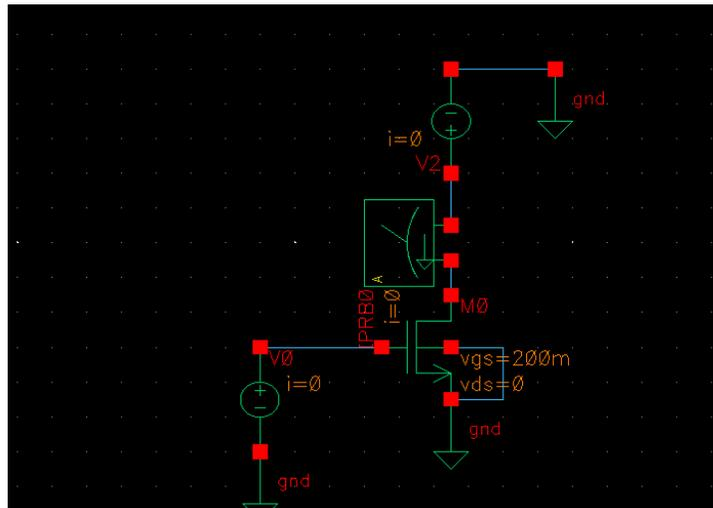
Fig. 5.1: Conventional NMOS simulation setup
