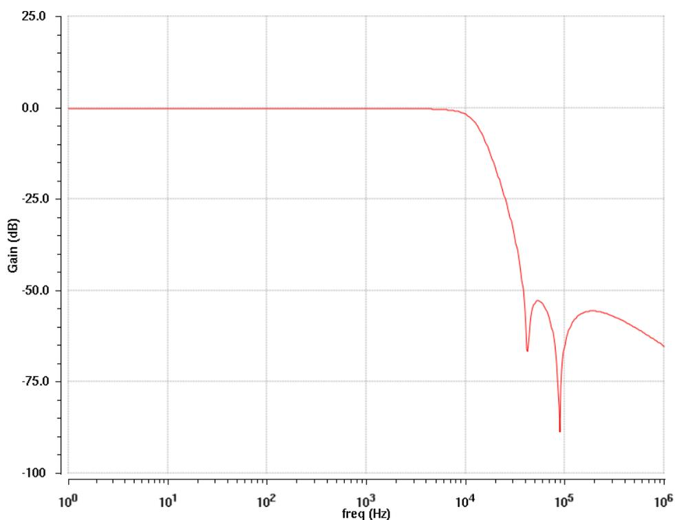
Fig. 6.3: Simulated filter characteristics, Gain vs. frequency ( $V_{DD}=1V$ )
