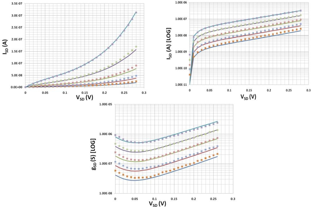
Fig. 1.10: Drain-bulk connected PMOS transistor, with respective output characteristics,  $I_{SD}$ ,  $g_{SD}$  vs.  $V_{SD}$  are shown for various values of  $V_{SG}$  (markers: measurements, lines: analytical charge-based model).
