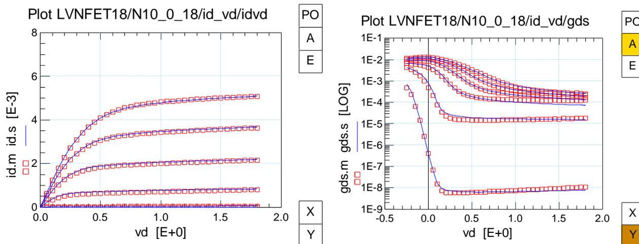
Fig. 1.53: Output Characteristics  $I_{DS}-V_{DS}$ ,  $g_{DS}-V_{DS}$  (NMOS W/L=10um/0.18um)
