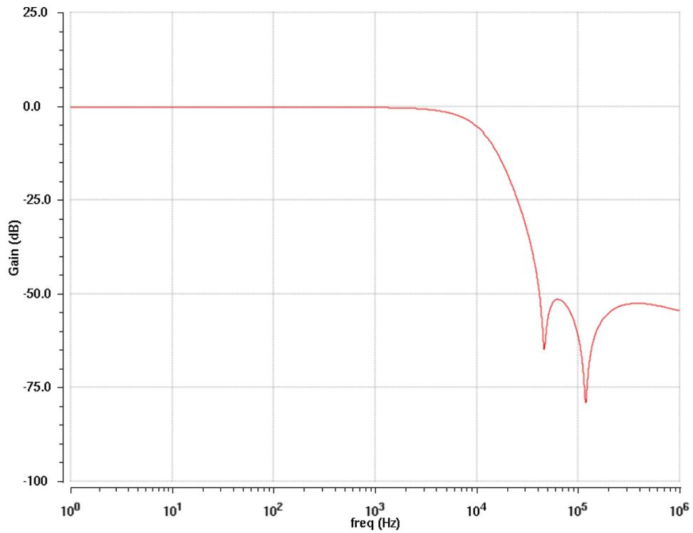
Fig. 6.5: Gain vs. frequency of the 0.5V low-pass elliptic filter
