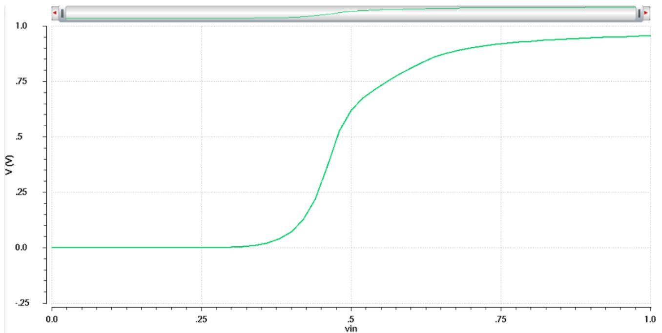
Fig. 5.12: DC transfer characteristics (Differential output-Positive input)
