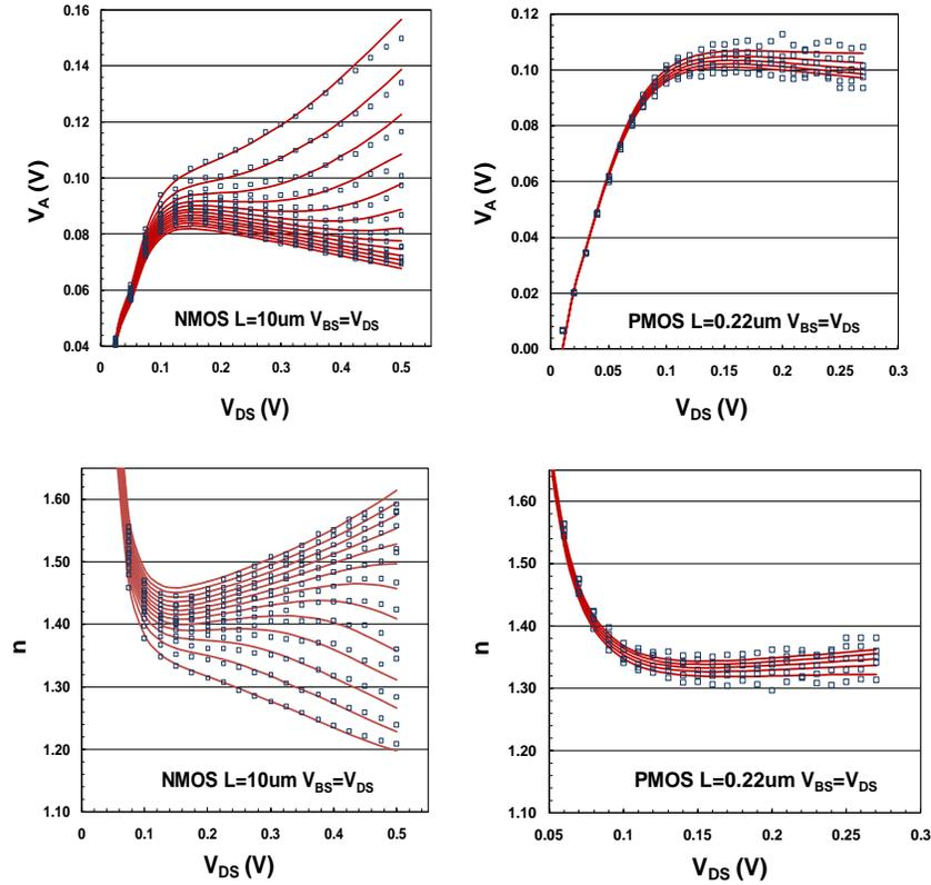
Fig. 1.44: Early Voltage  $V_A$  and slope Factor  $n$  extracted from Equation (1.19) of drain-bulk connected NMOS (left) and PMOS (right) devices (markers: TCAD/measured data, lines: EKV3/analytical model).
