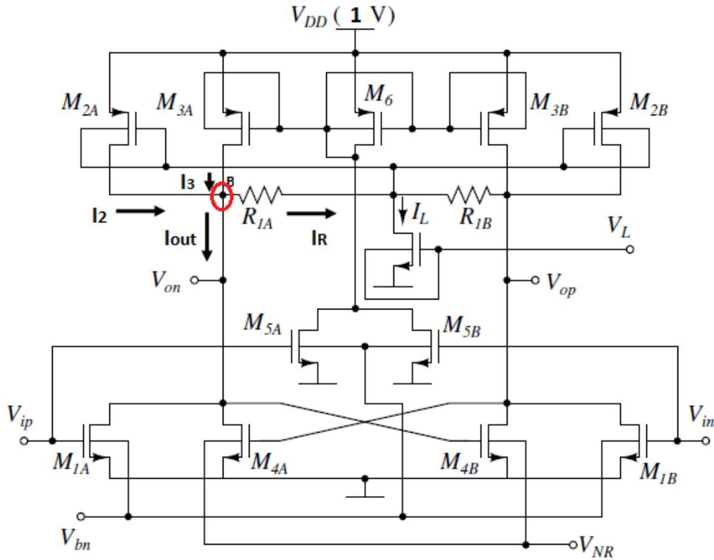
Fig. 5.20: DC Analysis of Gate-input OTA
