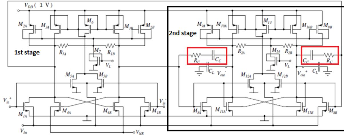
Fig. 5.25: Two-stage, fully differential, gate-input OTA, with Miller compensation.
