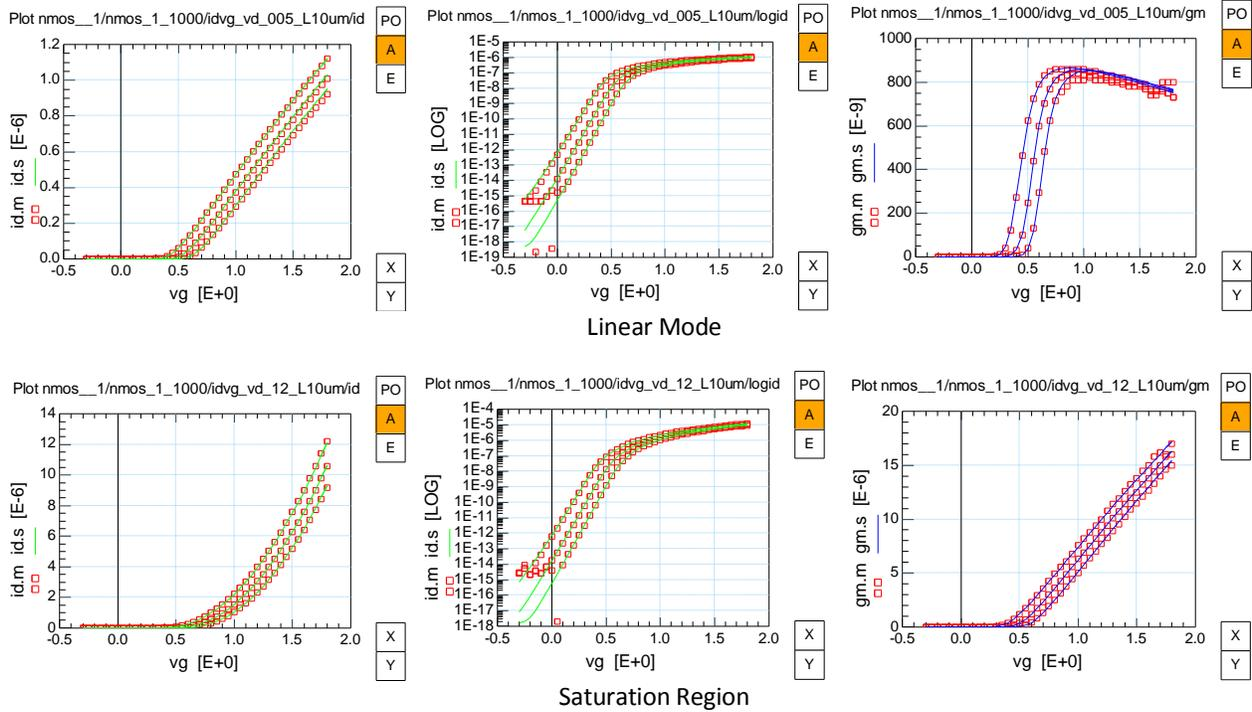
Fig. 1.19: NMOS Source-Bulk output characteristics  $I_{DS}$ ,  $g_m$  vs.  $V_{GS}$  ( $W/L=1\mu m/10\mu m$ ), linear region (up) and saturation region (down)
