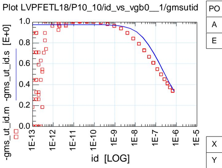
Fig. 1.59: Output Characteristics  $I_{DS}-V_S$   $g_{ms}-V_S$ ,  $g_{ms}/I_{DS}$   $V_G=V_B$  (PMOS W/L=10um/10um)
