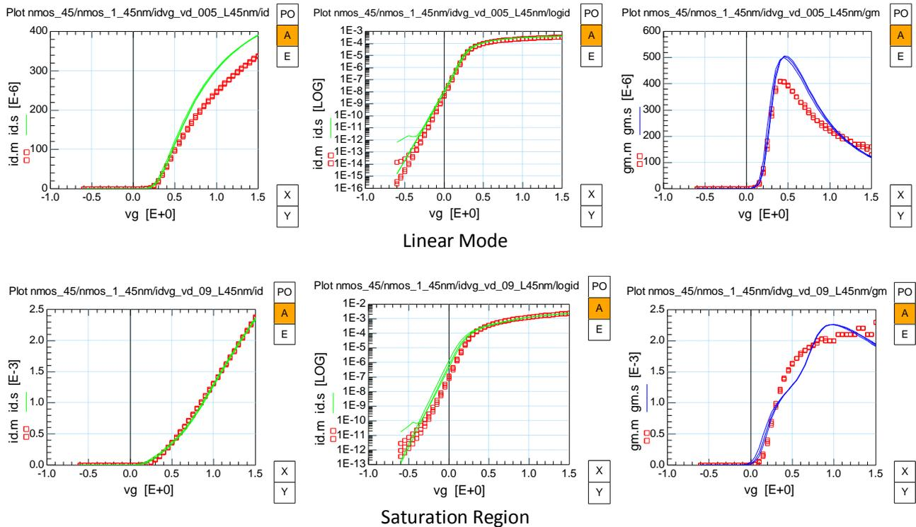
Fig. 1.39: NMOS Source-Bulk output characteristics  $I_{DS}$ ,  $g_m$  vs.  $V_{GS}$  ( $W/L=1\mu\text{m}/45\text{nm}$ )
