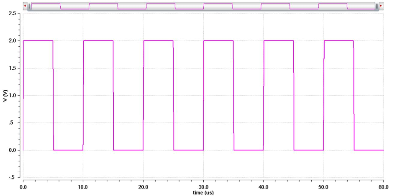
Fig. 5.17: Input signal for Slew Rate simulation
