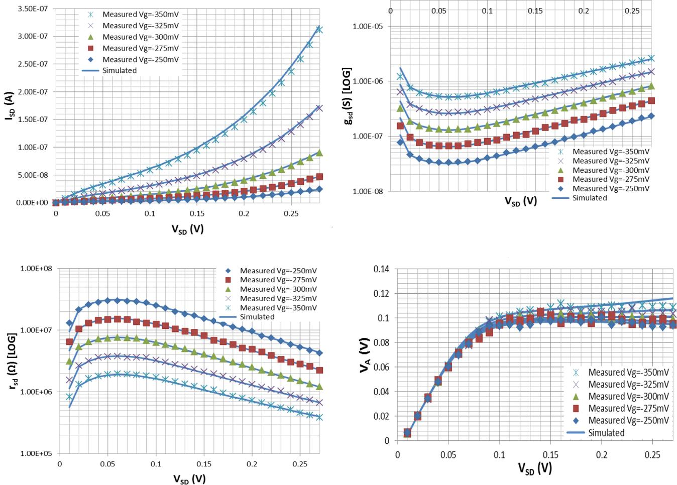
Fig. 1.16: Drain-Bulk Connected PMOS (W/L=10um/0.18um)
