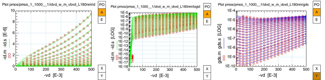
Fig. 1.33: PMOS Drain-Bulk output characteristics  $I_{DS}$ ,  $g_{DS}$  vs.  $V_{DS}$  ( $W/L=1\mu\text{m}/180\text{nm}$ )
