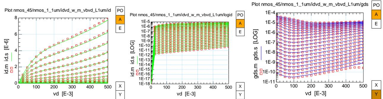
Fig. 1.37: NMOS Drain-Bulk output characteristics  $I_{DS}$ ,  $g_{DS}$  vs.  $V_{DS}$  ( $W/L=1\mu m/1\mu m$ )
