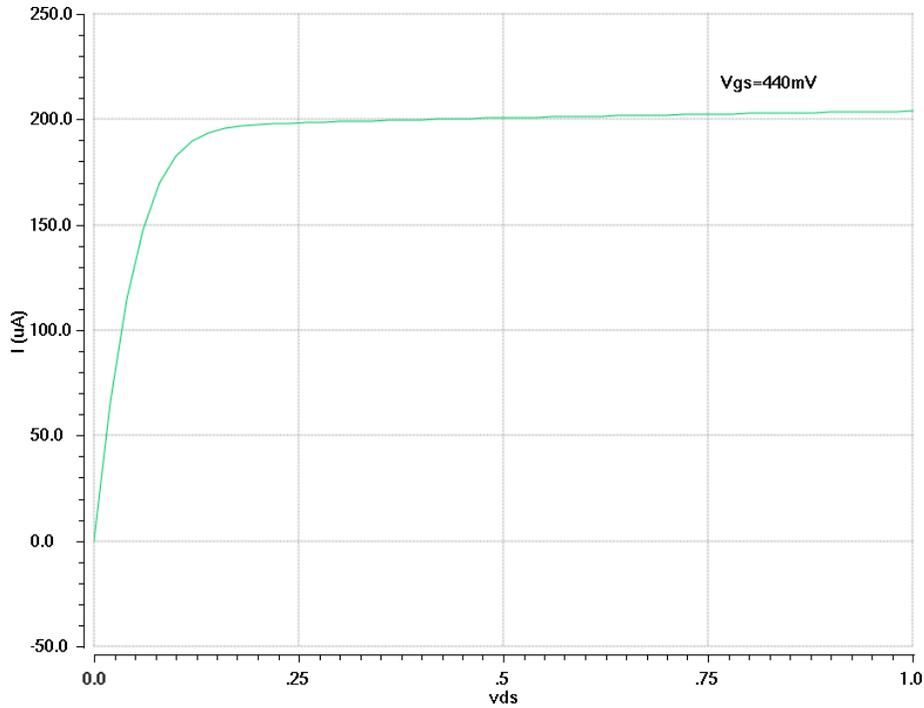
Fig. 5.8: I-V characteristics of grounded-gate NMOS current mirror
