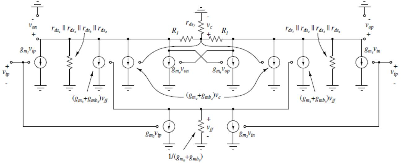
Fig. 3.6: Small-signal equivalent circuit of a single gain stage of the gate-input OTA.
