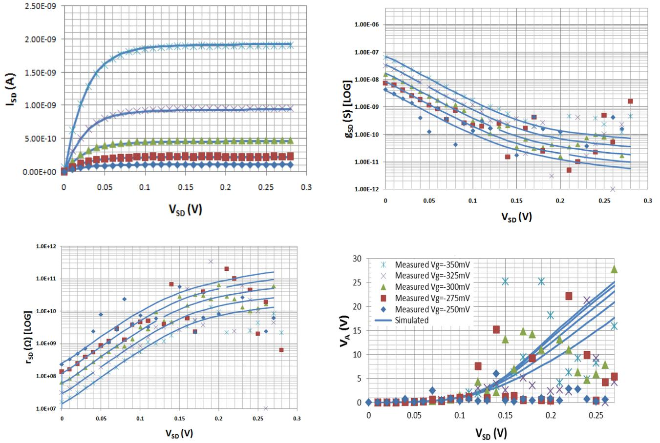
Fig. 1.17: Source-Bulk Connected PMOS W/L=10um/10um
