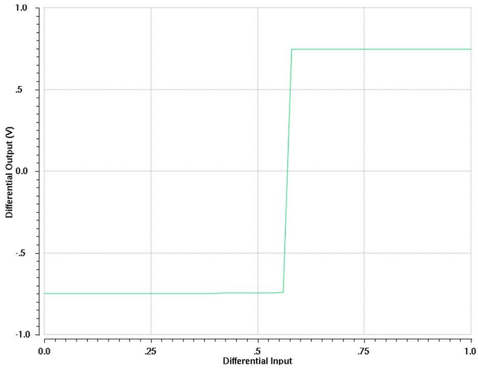
Fig. 5.26: DC input-output transfer characteristics of two stage OTA
