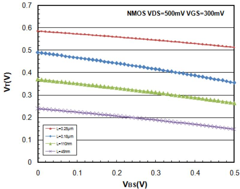
Fig. 2.8: Simulations of device  $V_T$  as a function of  $V_{BS}$  for advanced technology generations.
