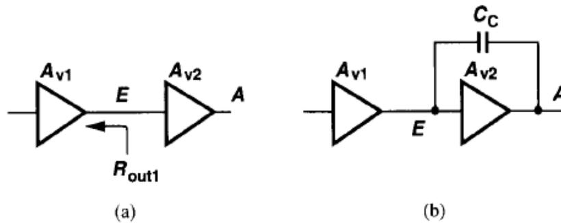
Fig. 3.13: Miller compensation of a two-stage op amp
