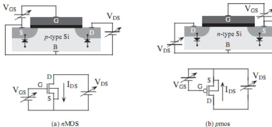
Fig. 1.3: Normal transistor biasing (a) NMOS and (b) PMOS
