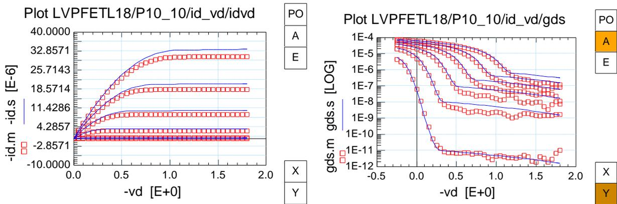
Fig. 1.58: Output Characteristics  $I_{DS}-V_{DS}$   $g_{DS}-V_{DS}$  (PMOS  $W/L=10\mu m/10\mu m$ )
