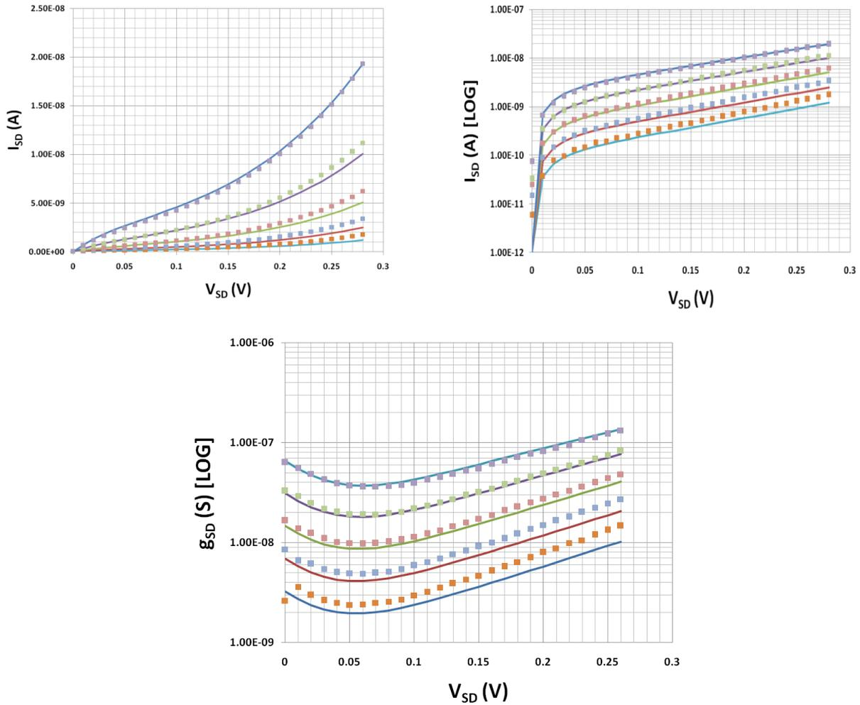
Fig. 1.12: Drain-bulk connected PMOS transistor, with respective output characteristics,  $W/L=10\mu m/10\mu m$ .  $I_{SD}$ ,  $g_{SD}$  vs.  $V_{SD}$  are shown for various values of  $V_{SG}$  (markers: measurements, lines: analytical charge-based model)
