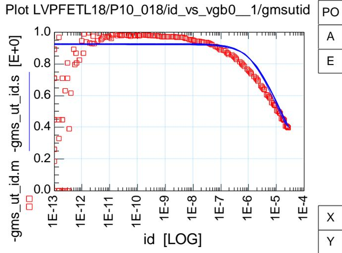
Fig. 1.64: Output Characteristics  $I_{DS}-V_S$   $g_{ms}-V_{DS}$ ,  $g_{ms}/I_{DS}$   $V_G=V_B$  (PMOS W/L=10um/0.18um)
