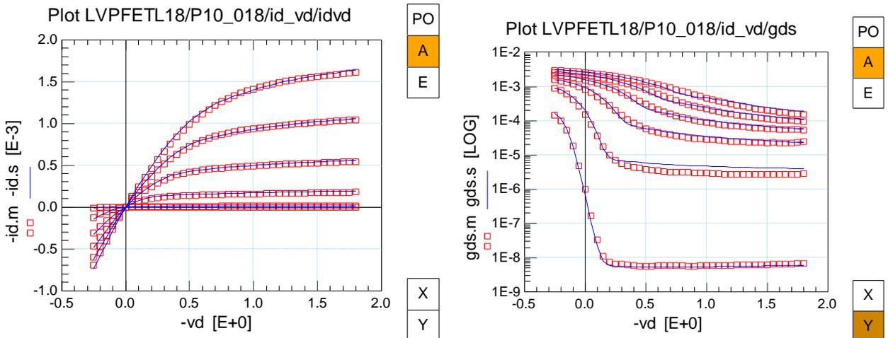
Fig. 1.63: Output Characteristics  $I_{DS}$ - $V_{DS}$ ,  $g_{DS}$ - $V_{DS}$  (PMOS W/L=10um/0.18um)
