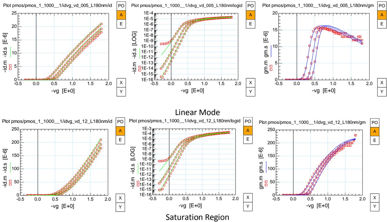
Fig. 1.31: PMOS Source-Bulk output characteristics  $I_{DS}$ ,  $g_m$  vs.  $V_{GS}$  ( $W/L=1\mu\text{m}/180\text{nm}$ )
