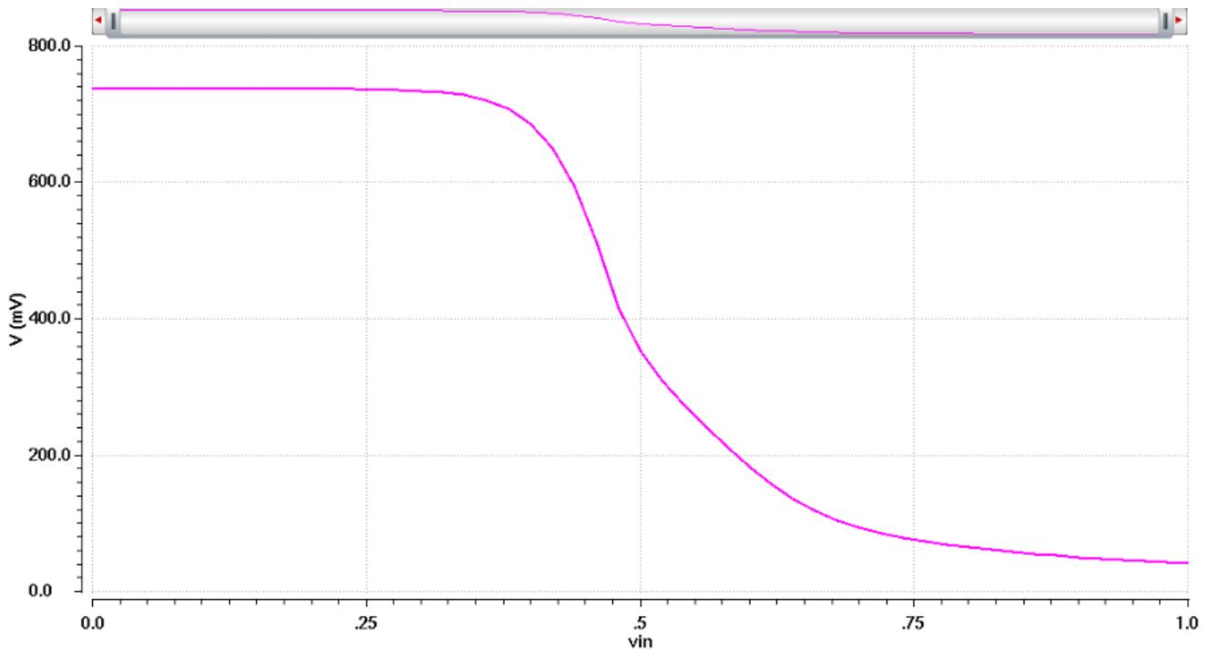
Fig. 5.11: DC transfer characteristics (Negative output-Positive input)
