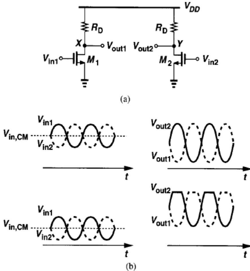
Fig. 3.3: (a) Simple differential circuit, (b) illustration of sensitivity to the input common-mode level
