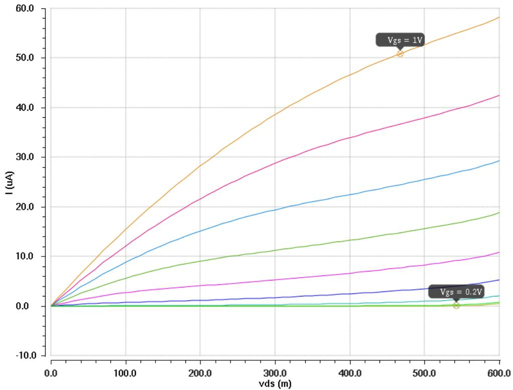
Fig. 5.5:  $I_{DS}$ - $V_{DS}$ , Drain-Bulk connected NMOS ( $W/L=10\mu\text{m}/10\mu\text{m}$ )
