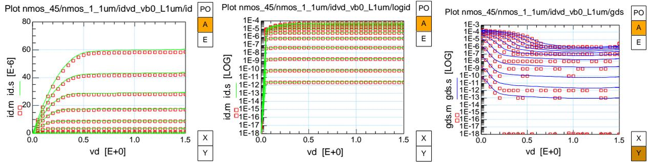
Fig. 1.36: NMOS Source-Bulk output characteristics  $I_{DS}$ ,  $g_{DS}$  vs.  $V_{DS}$  ( $W/L=1\mu m/1\mu m$ )
