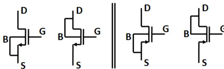
Fig. 1.9: NMOS (left) and PMOS (right) transistors, with their local substrate (or well) connected to either source or drain.
