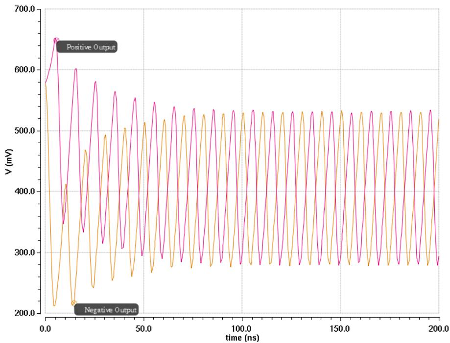
Fig. 5.23: Output signals in time domain (one stage OTA)
