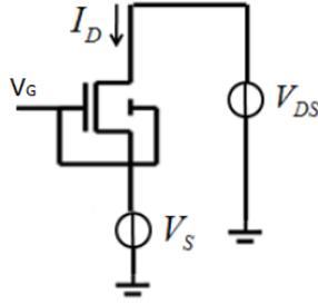
Fig. 1.47: Grounded-Gate MOSFET
