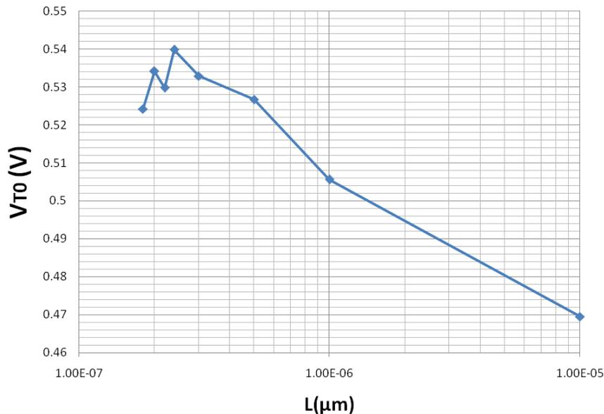
Fig. 1.14: Threshold Voltage vs. Channel Length
