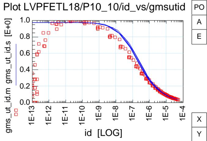
Fig. 1.59: Output Characteristics  $I_{DS}-V_S$   $g_{ms}-V_S$ ,  $g_{ms}/I_{DS}$  (PMOS W/L=10um/10um)
