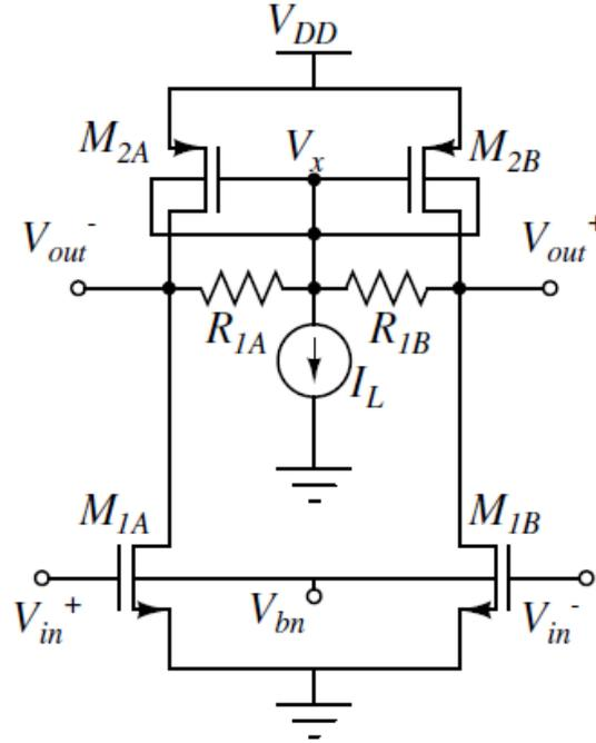
Fig. 3.2: Basic configuration of gate-input OTA
