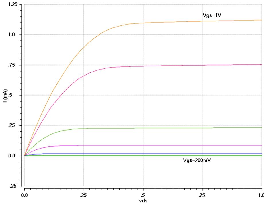
Fig. 5.3:  $I_{DS}-V_{DS}$ , Conventional NMOS ( $W/L=10\mu\text{m}/280\text{nm}$ )
