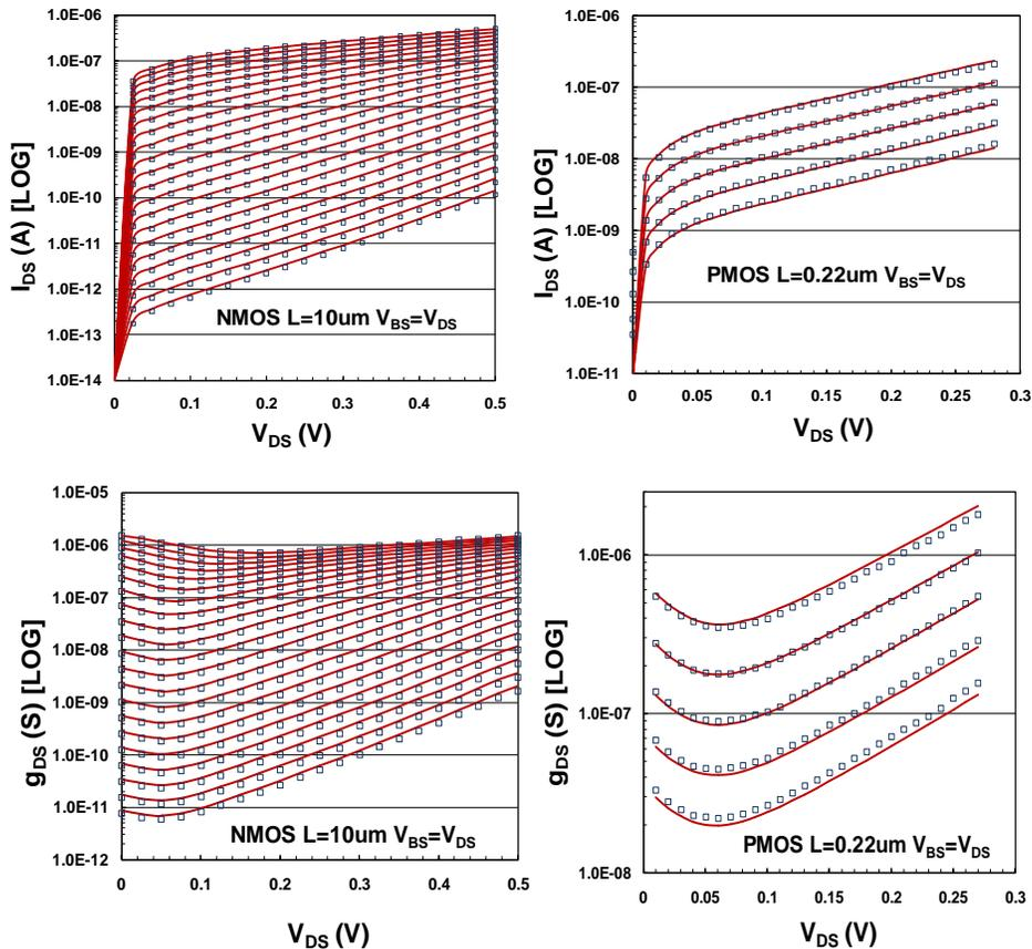
Fig. 1.43: Drain-bulk connected NMOS (left) and PMOS (right) transistor, with respective output characteristics,  $W/L=1\mu\text{m}/10\mu\text{m}$  (left) and  $W/L=10\mu\text{m}/0.22\mu\text{m}$ .  $I_{DS}$ ,  $g_{DS}$  vs.  $V_{DS}$  are shown for various values of  $V_{GS}$  (markers: TCAD simulation data(left), measurements (right), lines: EKV3 model (left), analytical charge-based model (right)).
