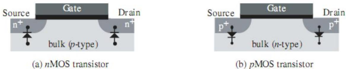
Fig. 1.2: Relative doping and equivalent electrical connections between device terminals for (a) NMOS and (b) PMOS transistors
