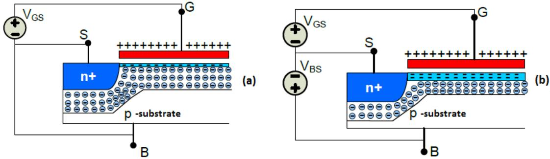
Fig. 2.6: Effect of forward-biasing the body-source junction in a weakly-inverted NMOS device: (a) Depletion and channel charges shown for a given  $V_{GS}$  and no body-source forward bias. (b) Depletion and channel charges shown for the same  $V_{GS}$  and small body-source forward bias.
