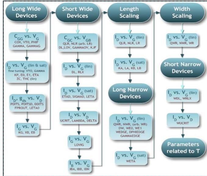
Fig. 1.69: DC parameter extraction basic scheme
