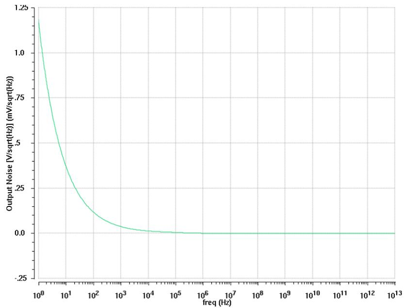
Fig. : Output – referred white noise spectral density
