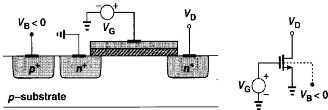
Fig. 2.4: NMOS device with negative bulk voltage
