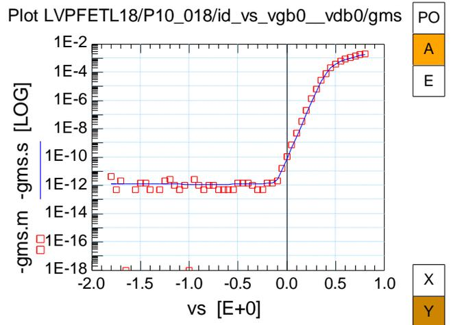
Fig. 1.64: Output Characteristics  $I_{DS}-V_S$   $g_{ms}-V_{DS}$ ,  $V_G=V_B=V_D$  (PMOS W/L=10um/0.18um)
