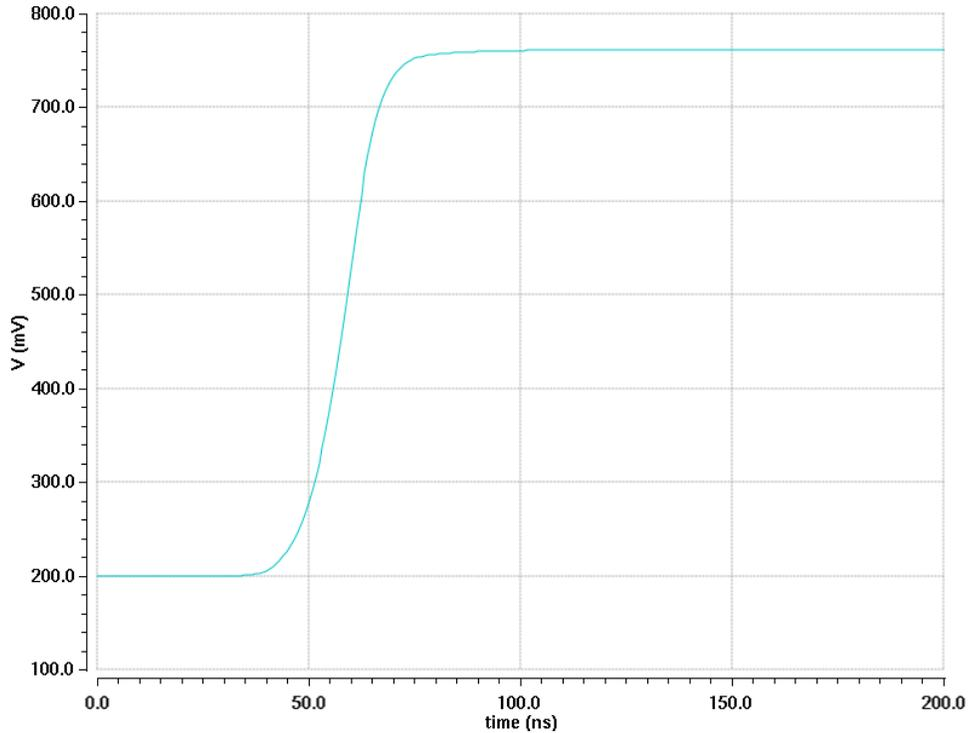
Fig. 5.24: Transient Output for simulating the Slew Rate
