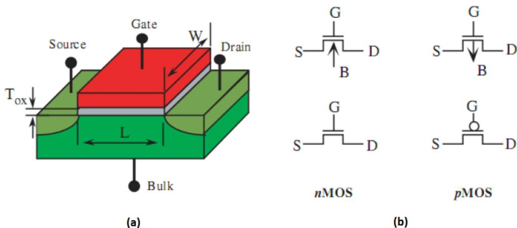
Fig. 1.1: (a) MOS structure (b) Symbols used at the circuit level
