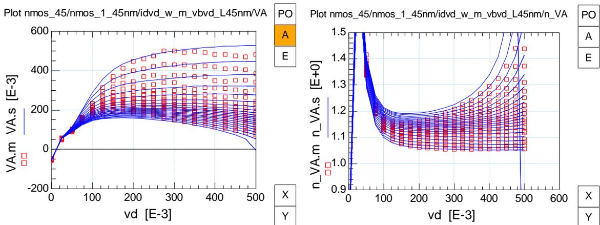
Fig. 1.42:  $V_A$ , and  $n$  vs.  $V_{DS}$  characteristics for the Drain-Bulk connected NMOS device ( $W/L=1\mu\text{m}/45\text{nm}$ )
