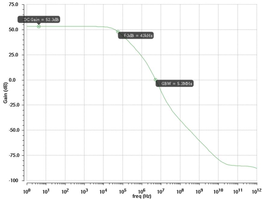
Fig. 5.35: Gain vs. frequency (0.5V OTA)
