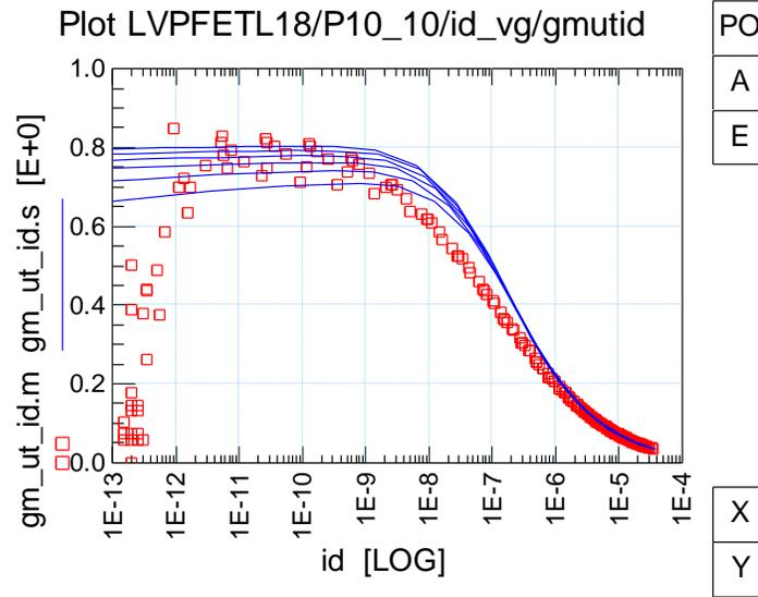
Fig. 1.57: Output Characteristics  $I_{DS}-V_{GS}$   $g_m-V_{GS}$ ,  $g_m/I_{DS}$  Saturation Region (PMOS  $W/L=10\mu m/10\mu m$ )
