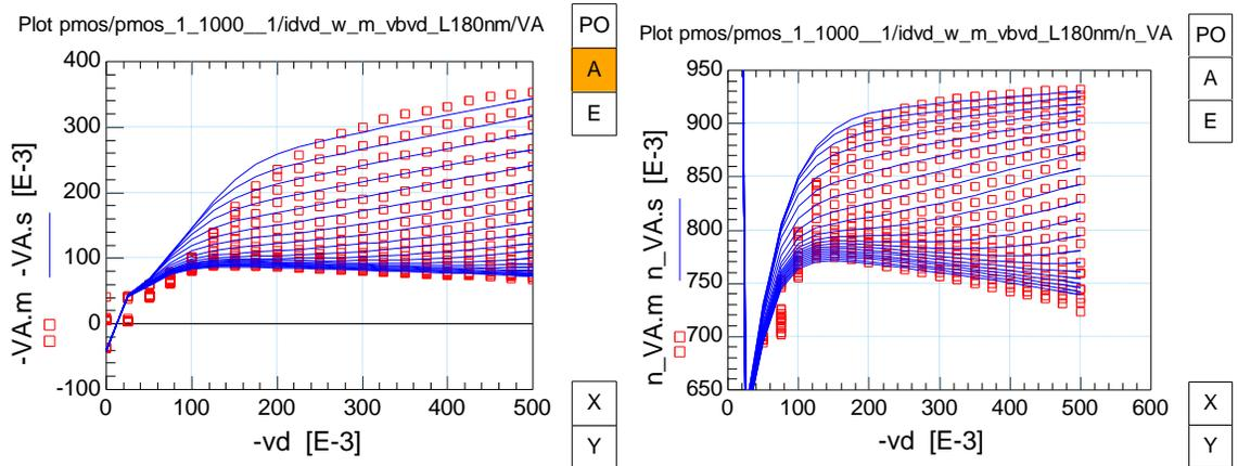
Fig. 1.34:  $V_A$ , and  $n$  vs.  $V_{DS}$  characteristics for the Drain-Bulk connected PMOS device ( $W/L=1\mu\text{m}/180\text{nm}$ )
