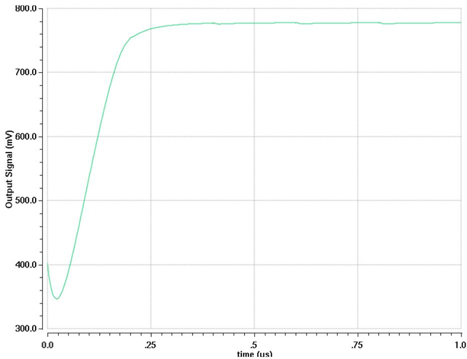
Fig. 5.33: Output Signal for Slew Rate simulation (two-stage OTA)
