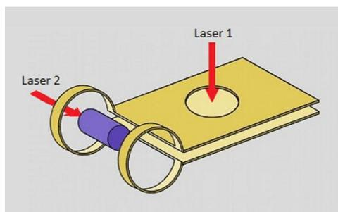
Figure 2. Generation of a 10 kiloTesla magnetic field of about 2ns duration in the coils by firing a >kilojoule nanosecond laser pulse 1 into the hole between the plates. The HB11 fusion fuel is a solid cylinder of 1cm length and 1 mm radius coaxially located in the coils and the block-ignition of the fusion flame is produced by a ps-30 PW laser pulse of 0.2 mm diameter for block ignition from laser 2.
