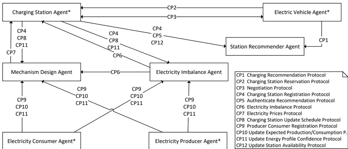
Figure 5.1: Overview of the proposed architecture depicting also the communication protocols used. Stars (\*) denote agent types with multiple instances. Arrows start from the agent that initiates the protocol and point to the receiver agents.
