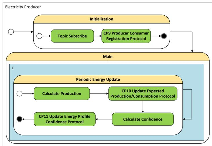
Figure 5.19: The intra-agent model of the Electricity Producer.
