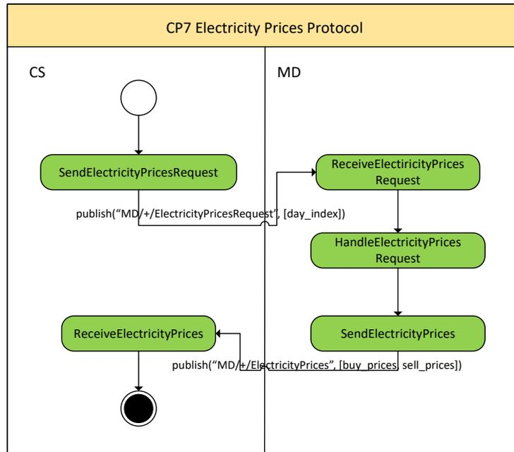
Figure 5.8: The model of the Electricity Prices Protocol (CP7)
