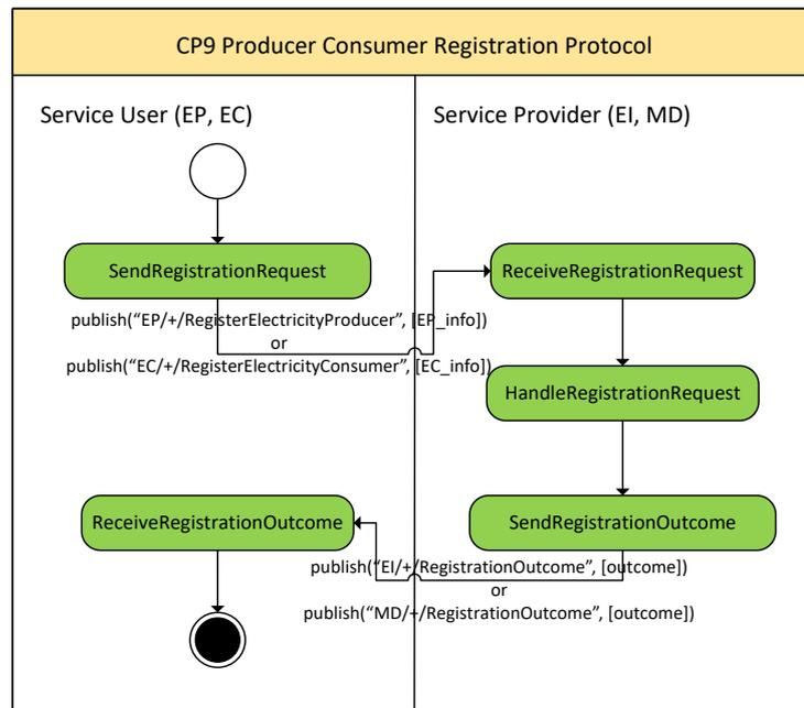
Figure 5.10: The model of the Producer Consumer Registration Protocol (CP9)
