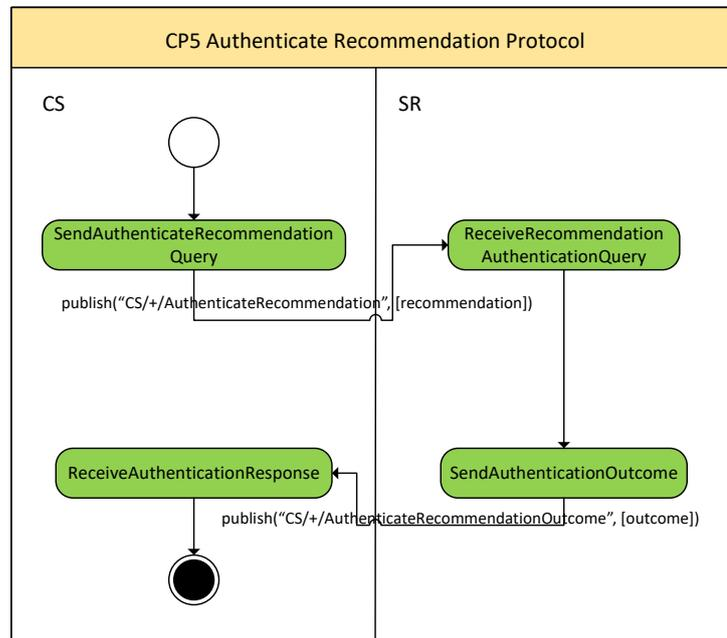
Figure 5.6: The model of the Authenticate Recommendation Protocol (CP5)
