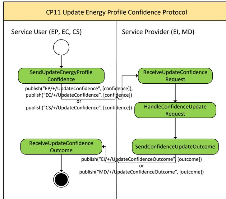
Figure 5.12: The model of the Update Energy Profile Confidence Protocol (CP11)
