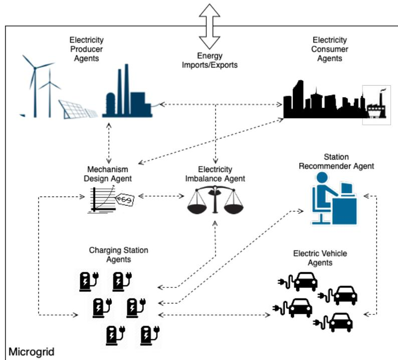
Figure 4.1: Overview of the proposed MAS architecture for the V2G/G2V problem.
