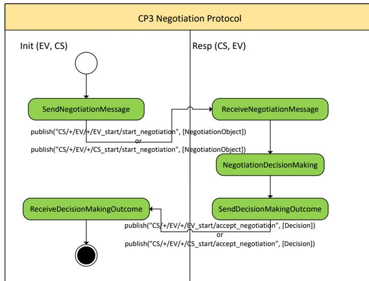
Figure 5.4: The model of the Negotiation Protocol (CP3)
