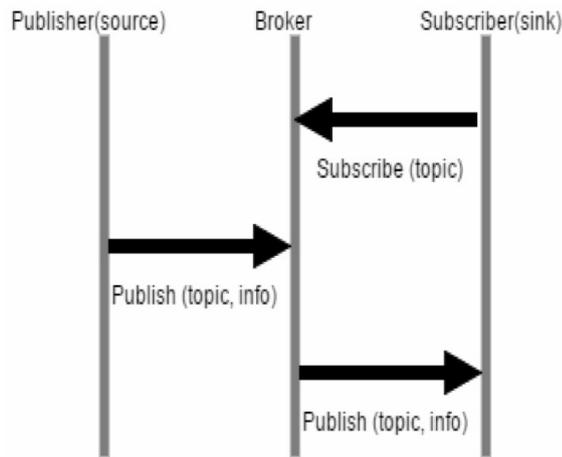
Figure 2.3: Publishers, subscribers and broker connection using MQTT [53]
