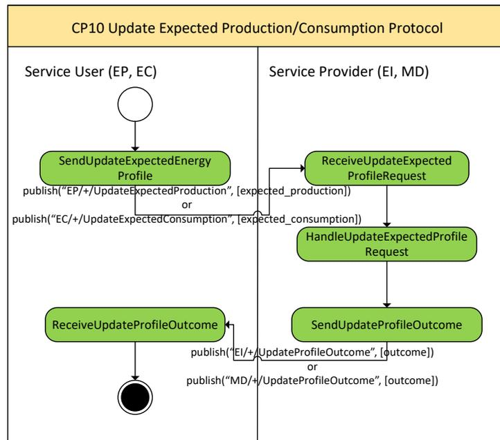
Figure 5.11: The model of the Update Expected Production/Consumption Protocol (CP10)
