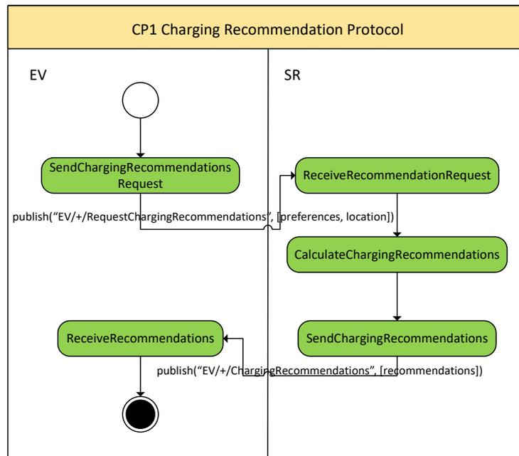
Figure 5.2: The model of the Charging Recommendation Protocol (CP1)
